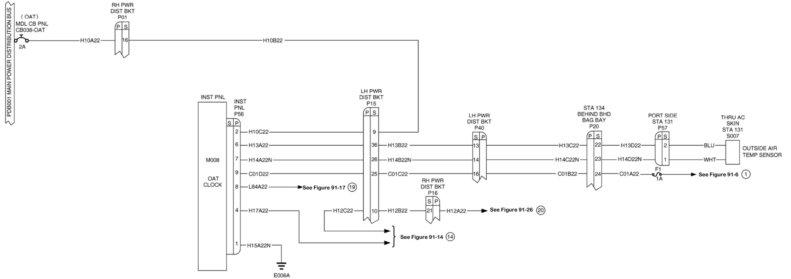
Figure 91-23 Outside Air Temperature Sensor and Clock System
