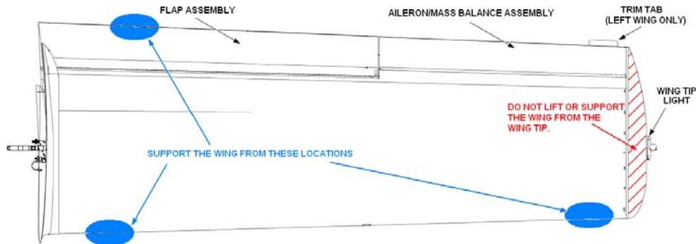
**Figure 57-11 Wing Handling Positions**
