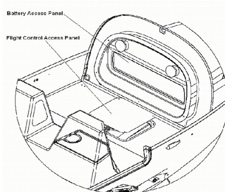
**Figure 25-2 Battery Access and Flight control Access Panels**
