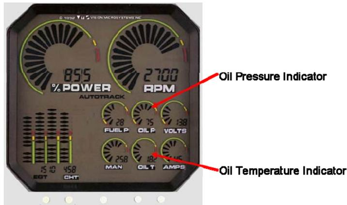
Figure 79-6 VM1000FX Oil Temperature and Pressure Indicators
