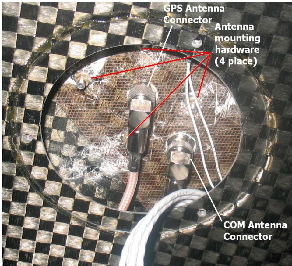
**Figure 23-11 View of the Underside of the Forward COM/NAV/GPS Antenna**
