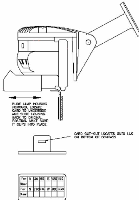
Figure 11-34 Example of the Compass Correction Card and Its Location on the Magnetic Compass
