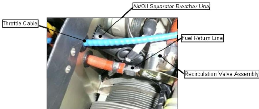
Figure 72-12 Fuel Return Line Penetration
