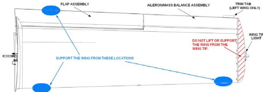
**Figure 57-8 Wing Handling Positions**
