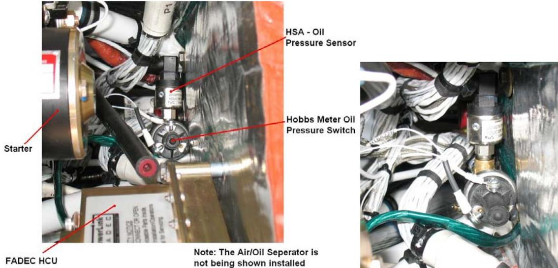
**Figure 77-13 Location of the Oil Pressure Switch (Hobbs) and the Oil Pressure Sensor (HSA) (The Air/Oil Separator Not Shown)**
