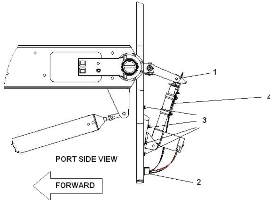
**Figure 27-55 Pitch Trim Actuator and Linkage**
