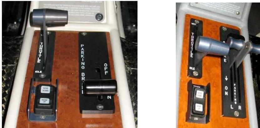
**Figure 09-3 Parking Brake in an Airplane with Toe Brakes (Left) and with Finger Brakes (Right)**
