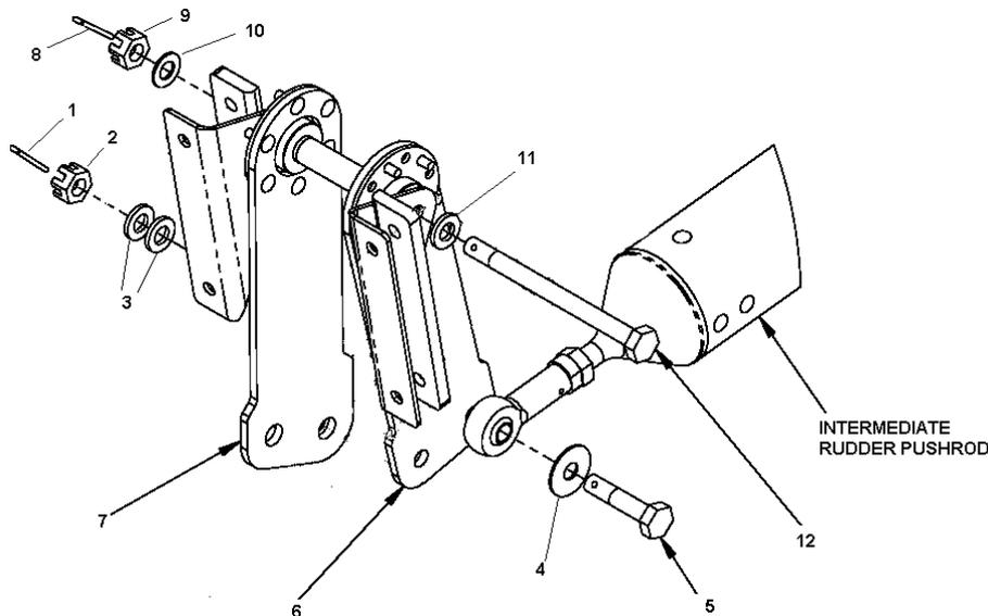
**Figure 27-30 Intermediate Rudder Pushrod and Center Idler-plate**
