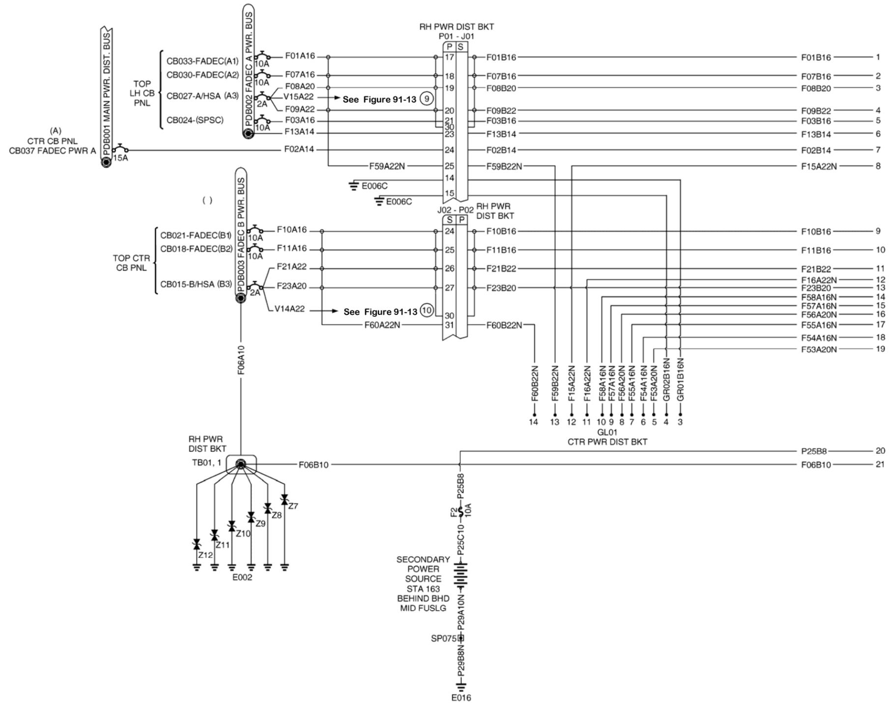
Figure 91-9 FADEC System Cabin Harness (1 OF 3)
