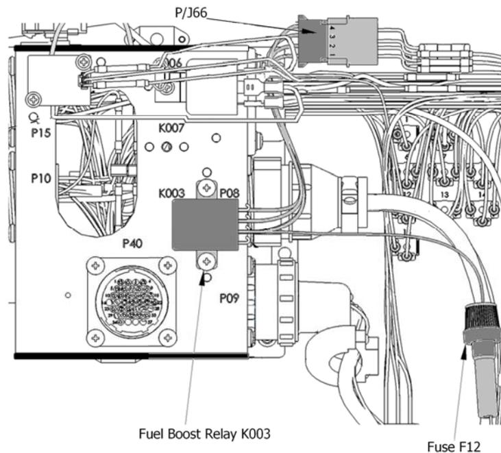
**Figure 28-15 Fuel Boost Relay Location**
