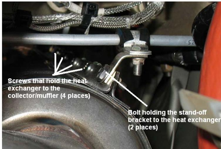
**Figure 78-5 Heat Exchanger Hardware**
