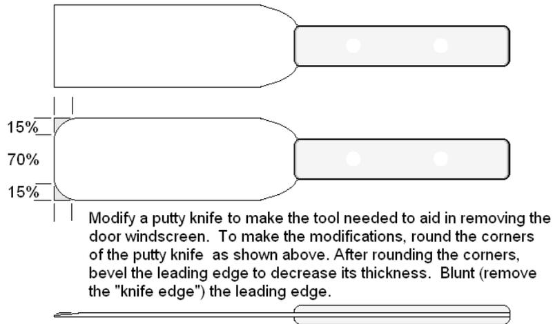
**Figure 56-3 Details of the Tool to Aid in Removal of the Door Windscreen**
