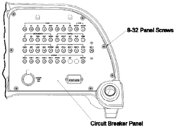
Figure 77-11 Circuit Breaker Panel
