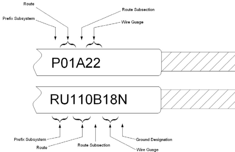
**Figure 20-7 Wire Number Coding Standard**
