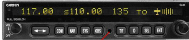
Hex-Key access to Unlock the Transceiver
