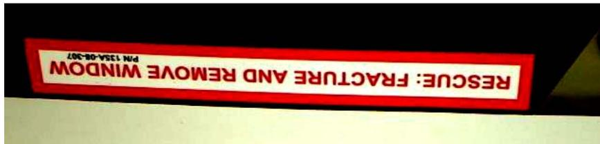
**Figure 52-11 Placard Instructing Rescuers to fracture and Remove Window in the Event of an Emergency (Placard is properly installed when it appears up side down when the door is in the closed position).**
