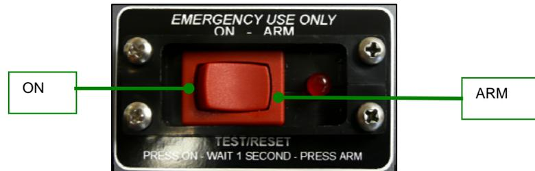
**Figure 25-37 Remote Switch – ELT Reset**
