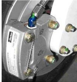
**Figure 20-2 Main wheel caliper safety wire**
