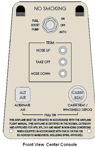
Figure 21-4 Center Console Cabin Heat Control
