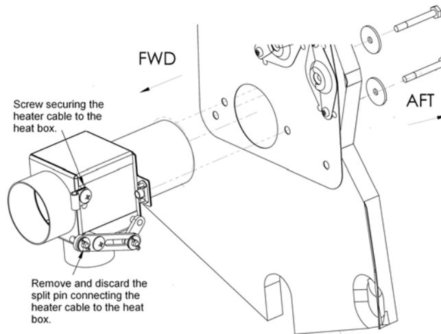
**Figure 21-13 Cabin Heat Box Assembly Installation**
