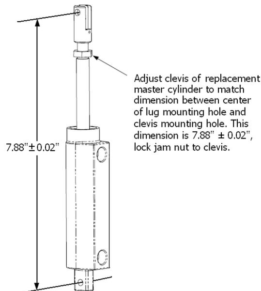
**Figure 32-26 Master Cylinder Clevis Adjustment**
