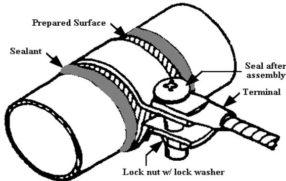
Figure 51-60 Bonding to a Metal Pipe/Tube/Hose
