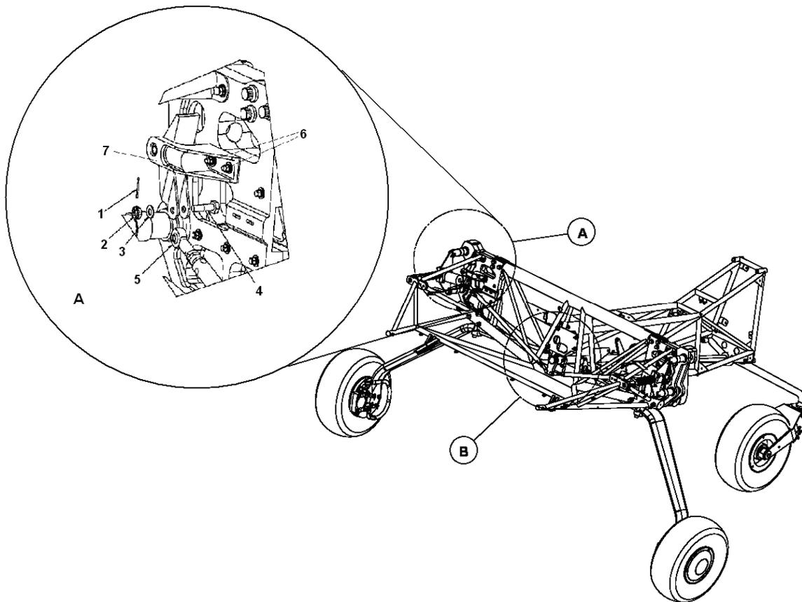
**Figure 27-16 Aileron Inboard Quick-disconnect Device**
