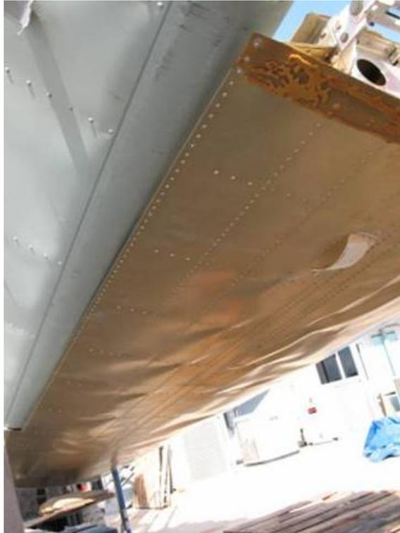
**Figure 57-14 Outer And Inner Panels Buckling On The Topside Skin Of Wing (Wing is Mounted With The Topside Down)**
