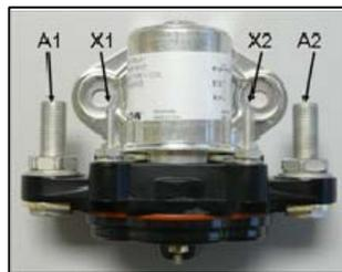
**Figure 24-19 Master Relay Showing the Relay's Connections**
