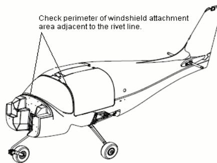
**Figure 56-20 Check Perimeter of Forward Windscreen for Cracks**
