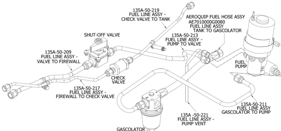
**Figure 28-14 Fuselage Fuel Lines**
