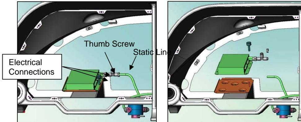
**Figure 34-14 Encoder Removal**
