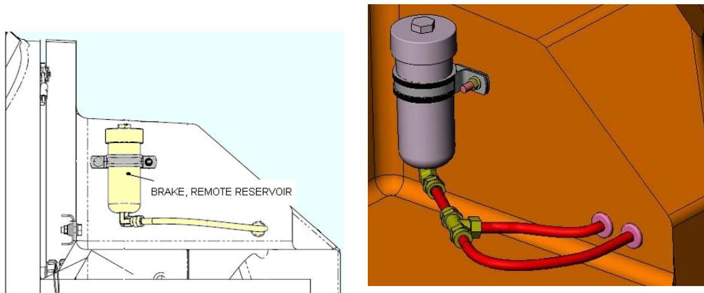
**Figure 32-40 Remote Reservoir for the Finger Brake System (Left) and the Toe Brake System with T-Fitting (Right)**
