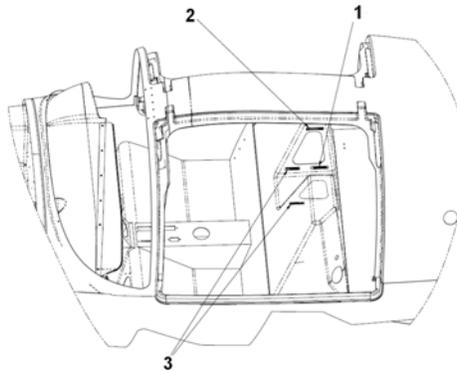
**Figure 11-20 Location of the Placards on the Center Console Seat Back**
