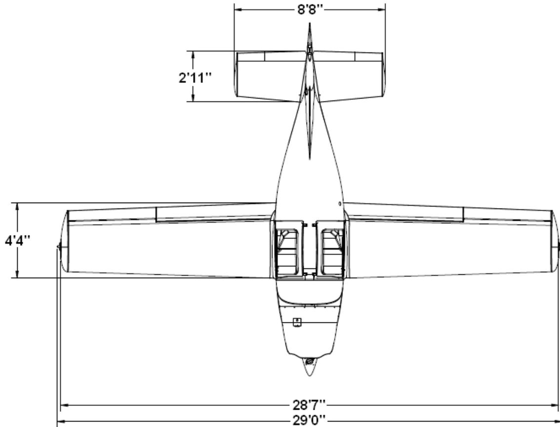
**Figure 06-3 (Reference Only) Top View of Airplane Dimensions**
