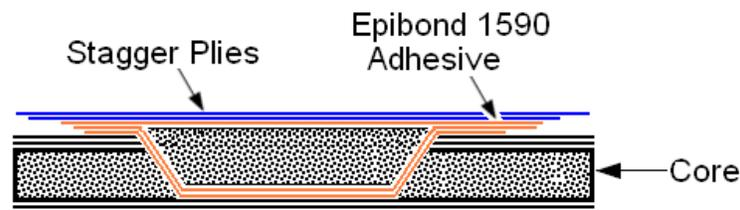
**Figure 51-11 Application of the Epibond Adhesive and the Staggered Plies of Plain Weave**
