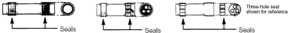
**Figure 20-10 Sealing Sleeves**
