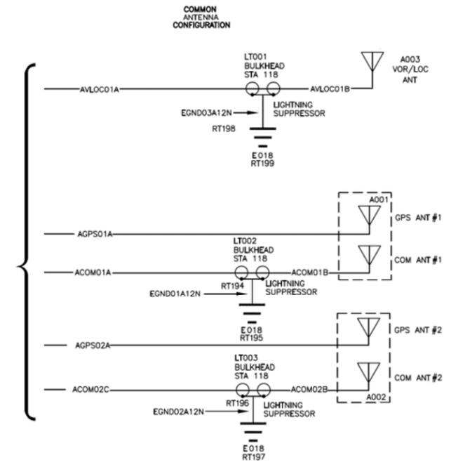
Figure 91-37 Avionics (Antenna Connections)
