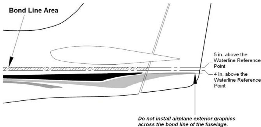
**Figure 11-4 Bond Line of the Fuselage – Do not Install Exterior Graphics or Placards Across the Bond Line**
