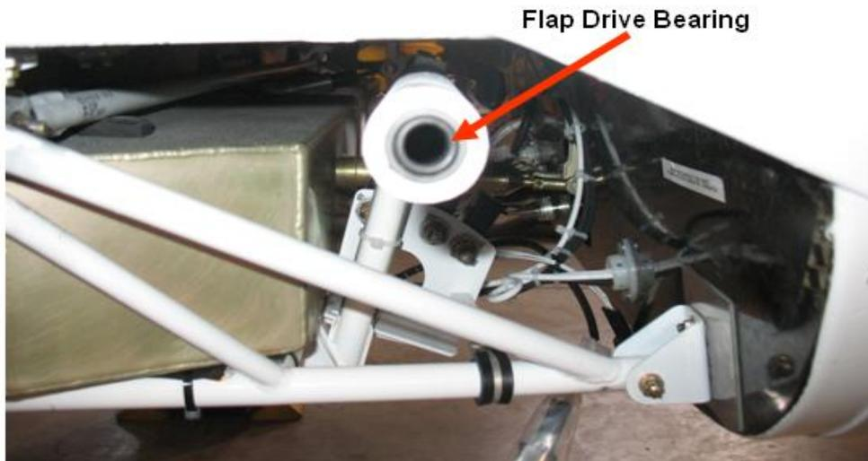
**Figure 27-75 Flap Drive Bearing**
