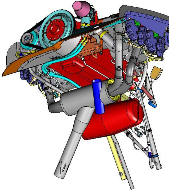
**Figure 78-1 Engine Exhaust System**
