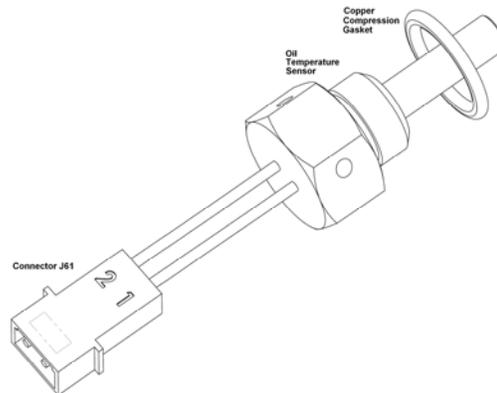
**Figure 77-17 Oil Temperature Sensor Showing the Copper Compression Gasket**
