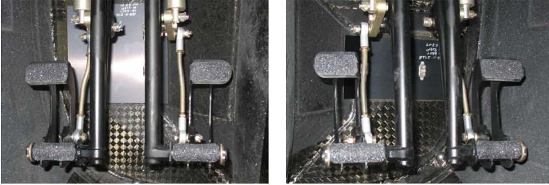
**Figure 09-2 Pilot's (Left) and Co-pilot's (Right) toe brakes**
