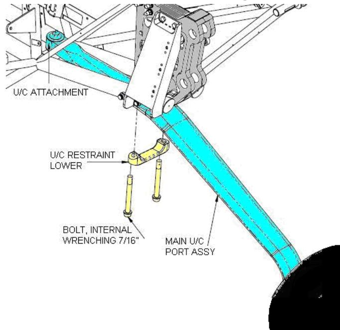
**Figure 32-2 Main Landing Gear Port Attachment Bolt and undercarriage Restraint Lower (Saddle)**
