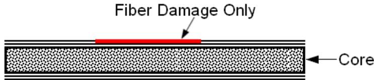
**Figure 51-32 Cross Section of the Damaged Area**
