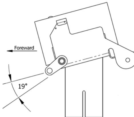
**Figure 71-49 Install The Flapper Arm With The Control Tab Pointing Forward**
