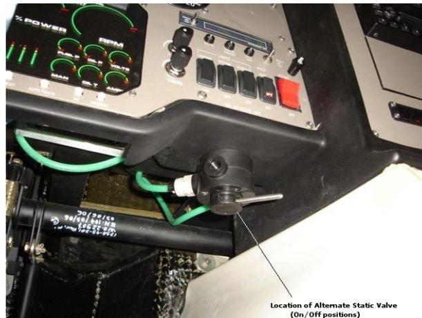
**Figure 34-2 Location of Alternate Air Valve**
