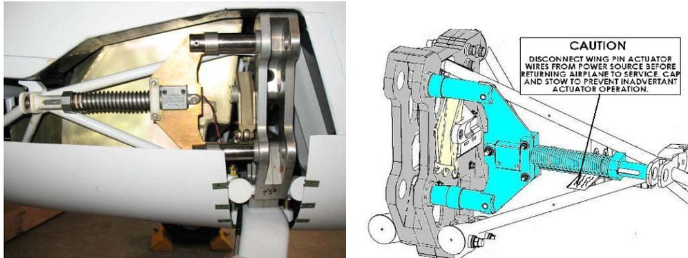
Figure 57-10 Electrical Wing Lock Mechanism
