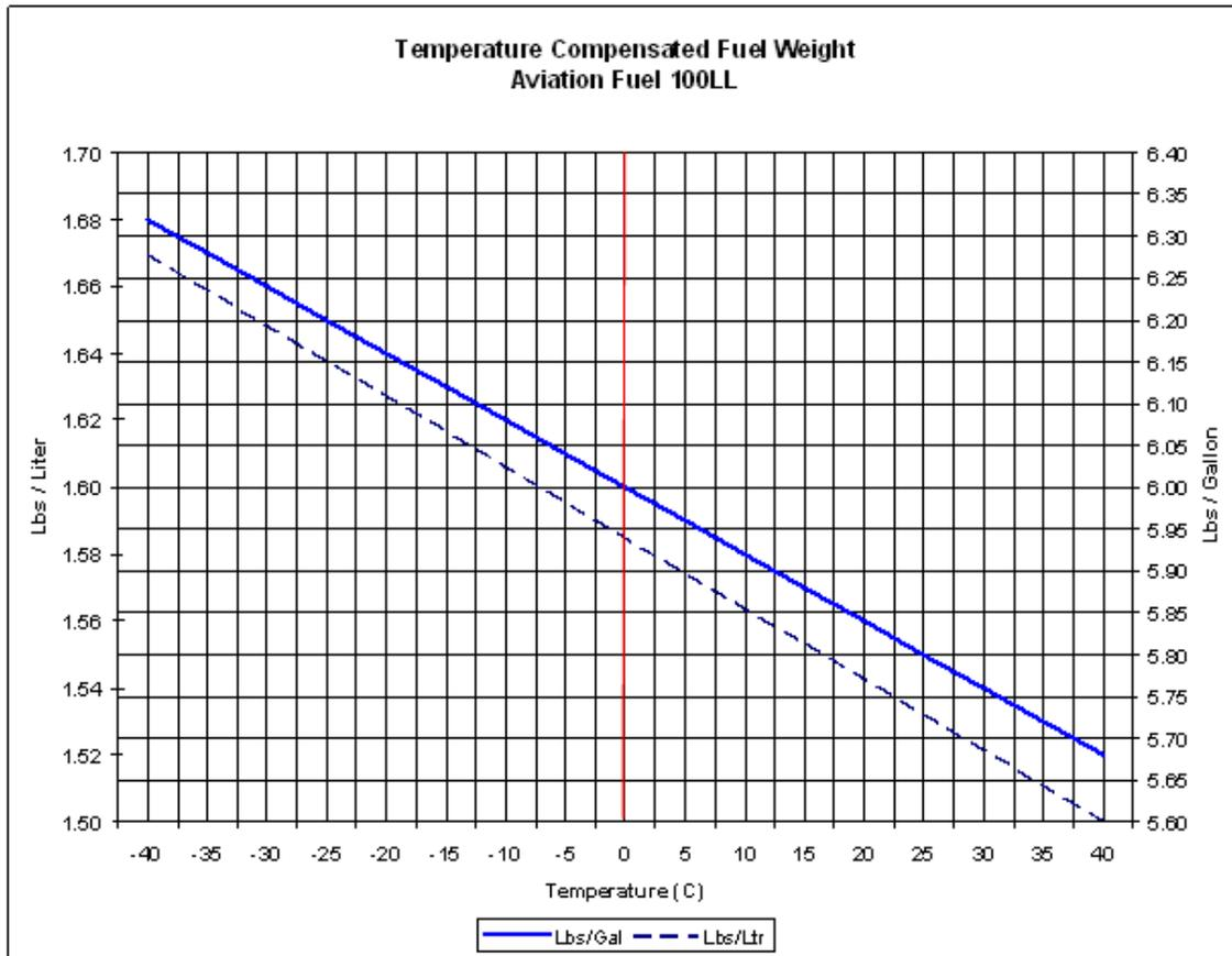
**Figure 28-22 Temperature Compensated Fuel Weight - 100LL**
