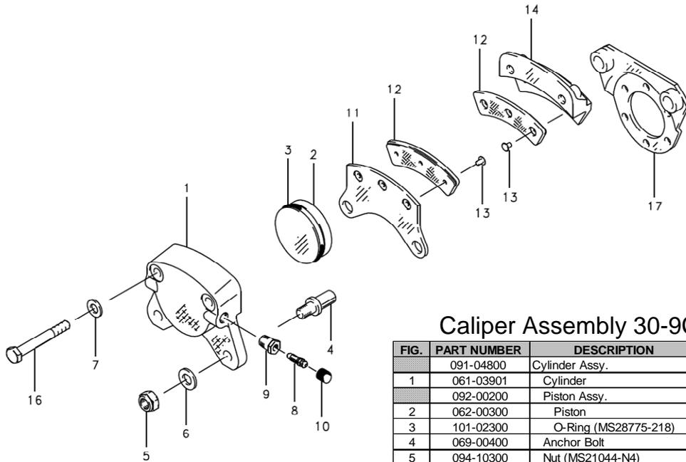
**Caliper Assembly 30-9C**
