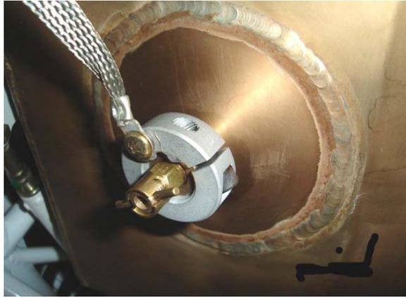
**Figure 12-3 Location of Fuel Tank Sump Drain**
