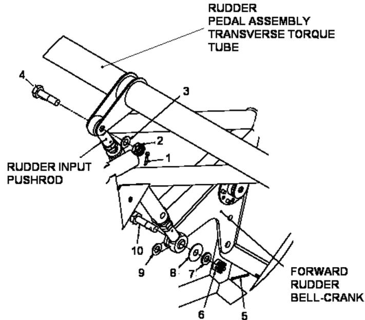
Figure 27-39 Exploded View of the Rudder Input Pushrod
