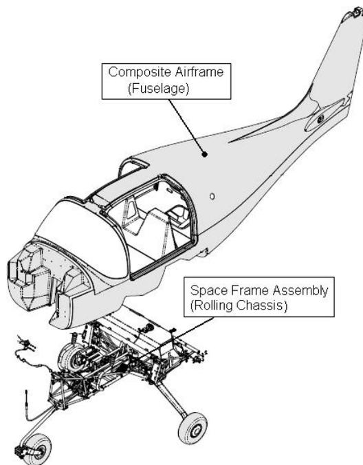
**Figure 53-1 Composite Airframe (fuselage)
