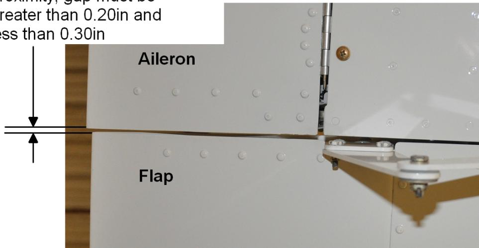
**Figure 27-73 Clearance between Flap and Aileron**
