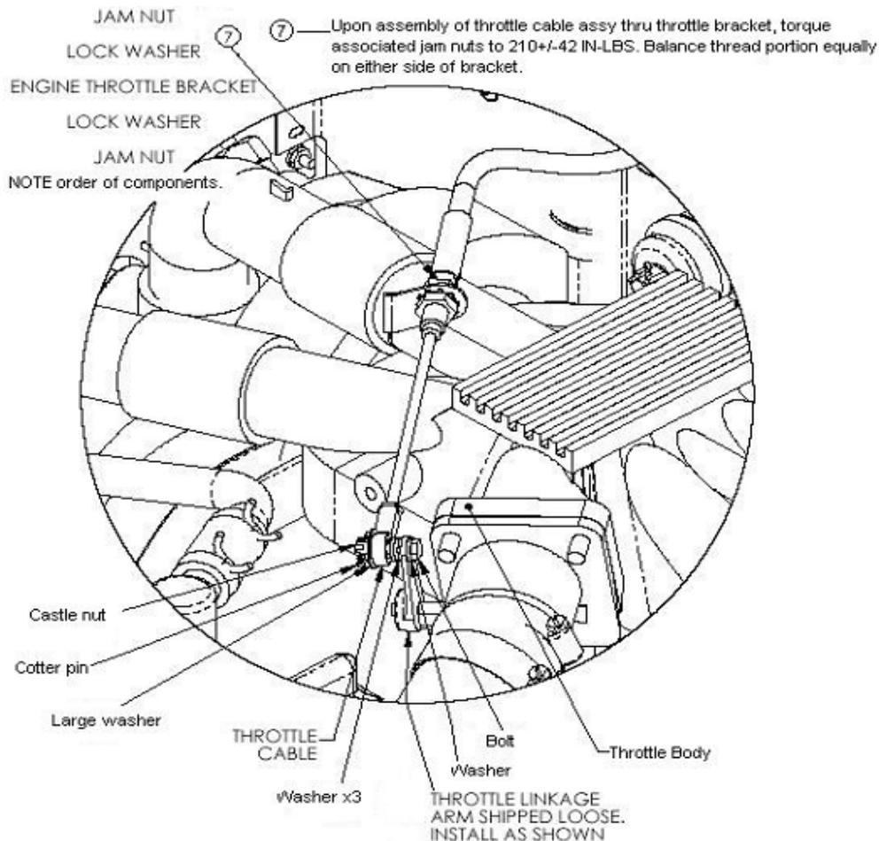
Figure 76-2 Throttle Cable Assembly
