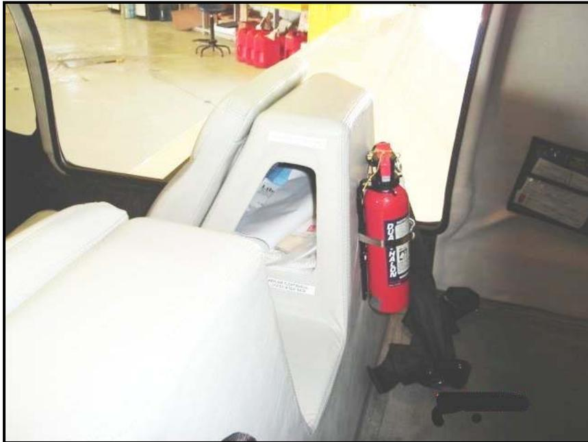
Figure 25-3 Location of Fire Extinguisher Behind the Passenger's/Co-Pilot's Seat
