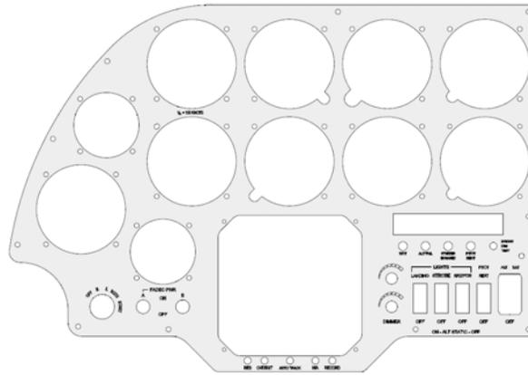
Figure 11-22 Placard for the Typical Instrument Panel
