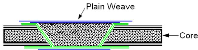
**Figure 51-22 Application of the Staggered Plies of Plain Weave**
