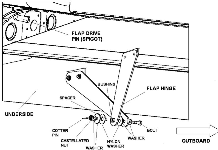
**Figure 27-66 Flap Hinge Assembly**
