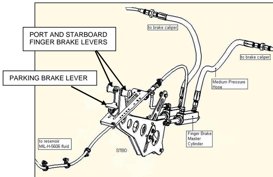
**Figure 32-33 Finger Brake System**
