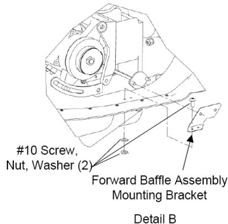
**Figure 72-7 Forward Baffle Assembly Upper Bracket**
