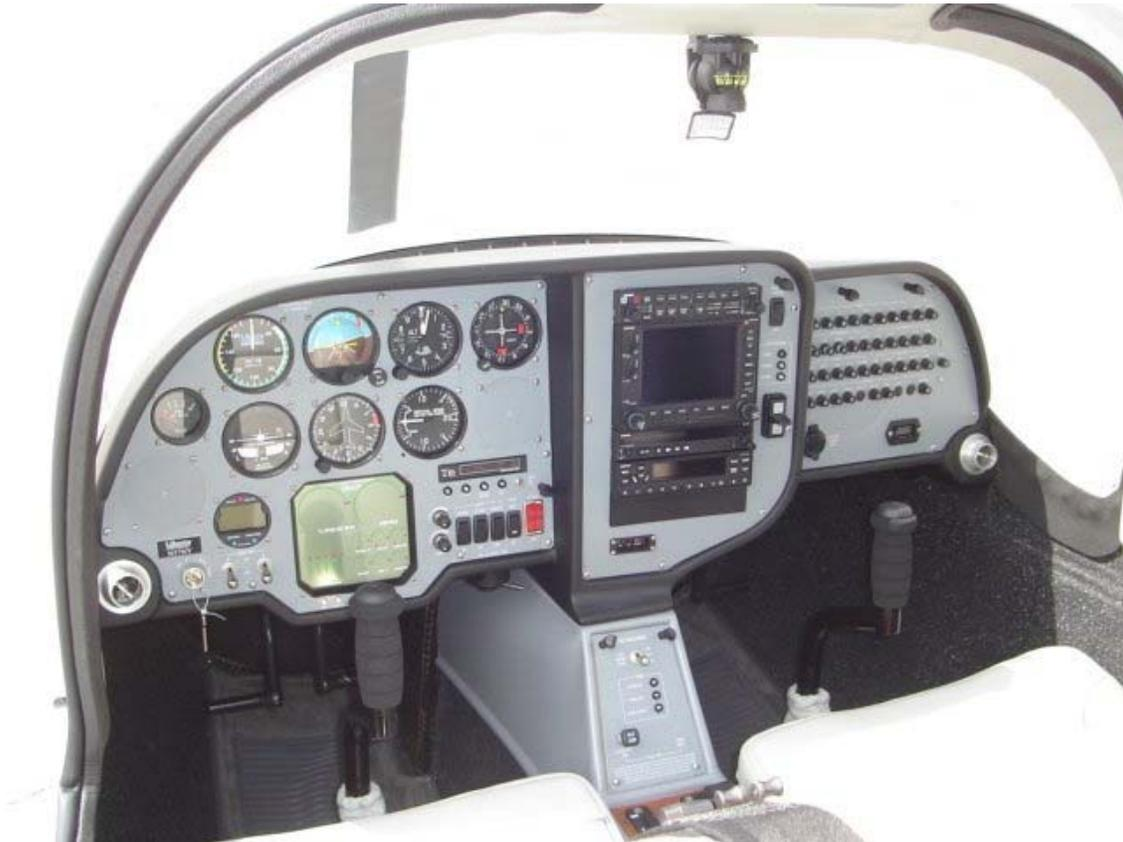
Figure 34-1 View of the Cockpit Navigation Instruments
