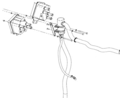
Figure 79-3 Exploded View of Air/Oil Separator
