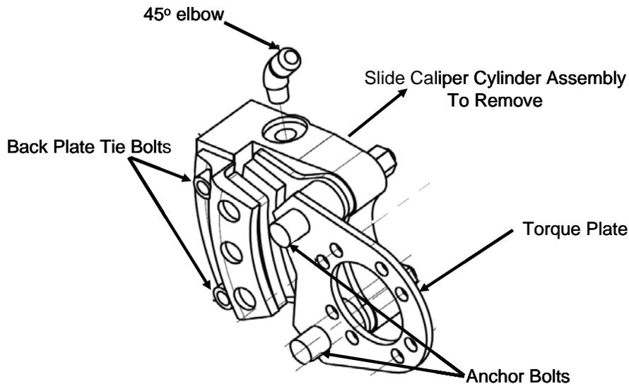
**Figure 32-35 Caliper Assembly**
