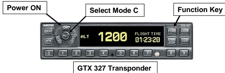
**Figure 34-19 GTX327 Transponder**
