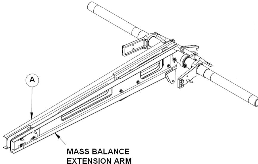
**Figure 55-5 Stabilator Mass Balance Arm**
