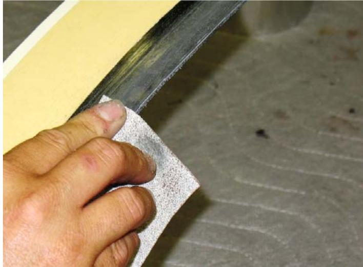
**Figure 56-4 Sanding the Carbon Surface to Prep the Surface**
