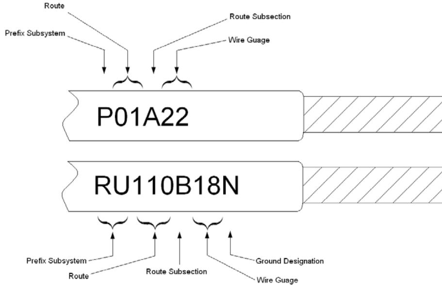
**Figure 91-1 Wire Number Coding Standard**
