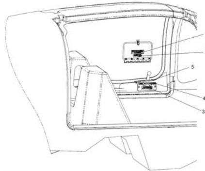
**Figure 11-19 Interior of the Port Door Showing the Location of the Placards**
