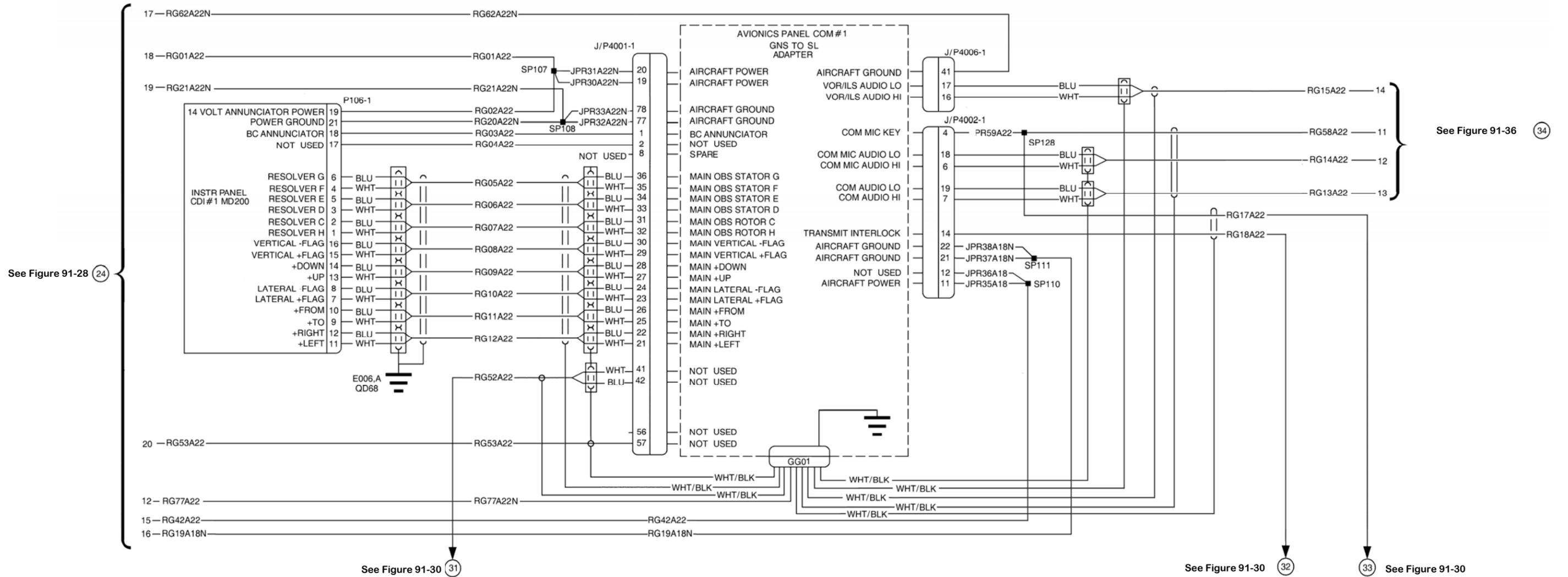
Figure 91-29 Avionics (Dual GNS System) 1 of 2
