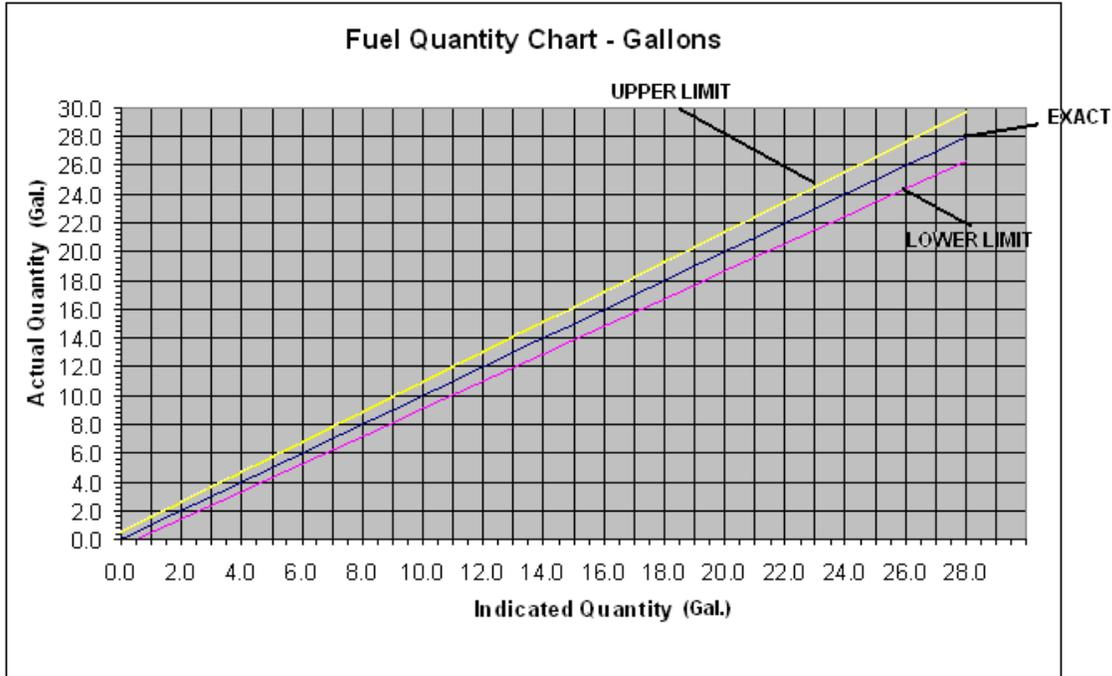
**Figure 28-29 Fuel Quantity Tolerance Chart – Gallons**
