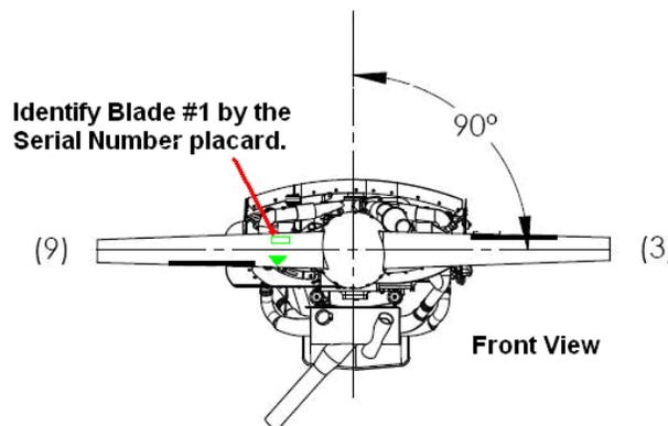
With engine cylinder #1 at Top Dead Center Compression, mount the propeller with blade #1 at the 9 o'clock position as shown above.
