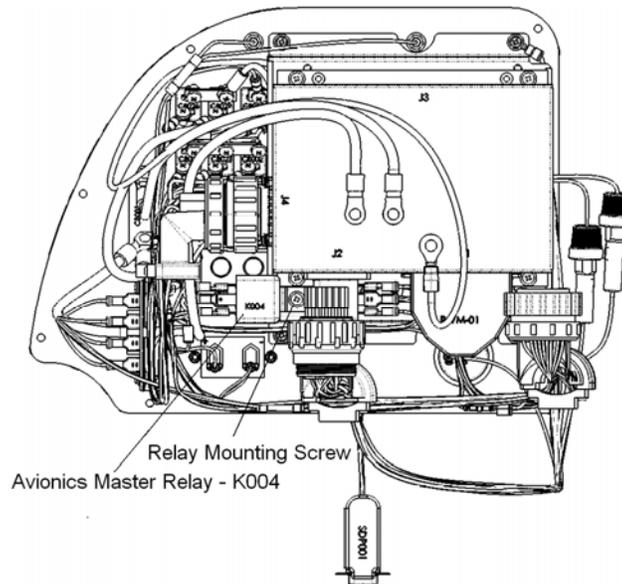
**Figure 24-23 Avionics Master Relay Location**
