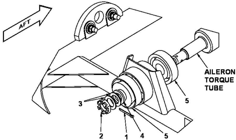
**Figure 27-21 Aileron Torque Tube (Front)**
