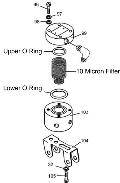
**Figure 73-4 Fuel Distribution Block Filter Assembly**
