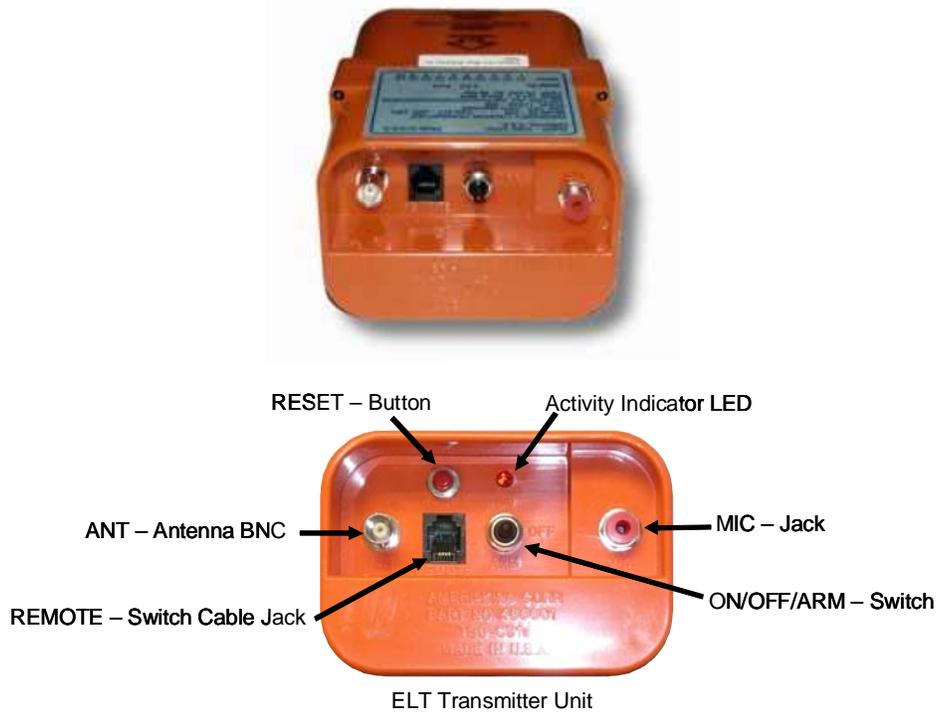
**Figure 25-12 Emergency Locator Transmitter – 121.5/243 MHz – TSO-C91a**
