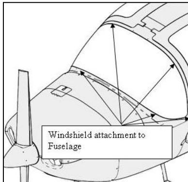
**Figure 53-6 Location Of The Windshield Attachment With The Fuselage**
