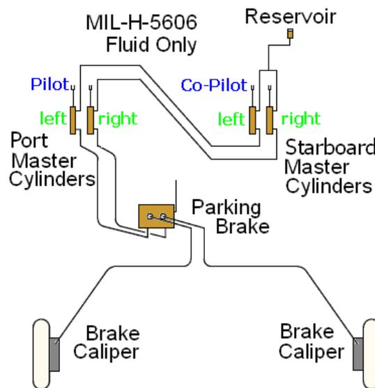
**Figure 32-24 Schematic Toe Brake System**
