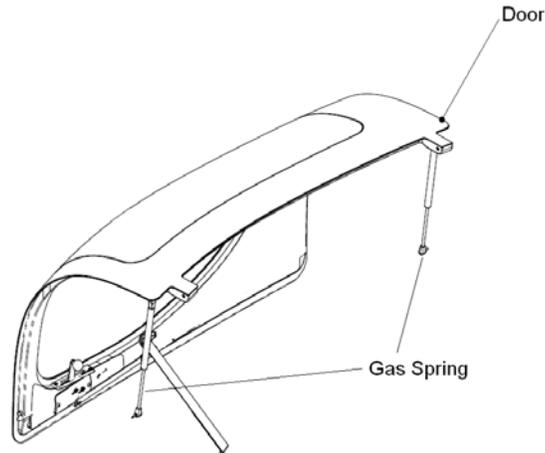
**Figure 52-10 Location of the Gas Spring Cylinder (Typical for Both Doors, Starboard Side Shown)**
