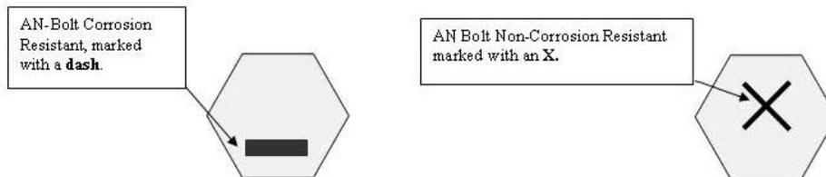
Figure 20-1 Bolt Markings to Indicate Corrosion Resistance
