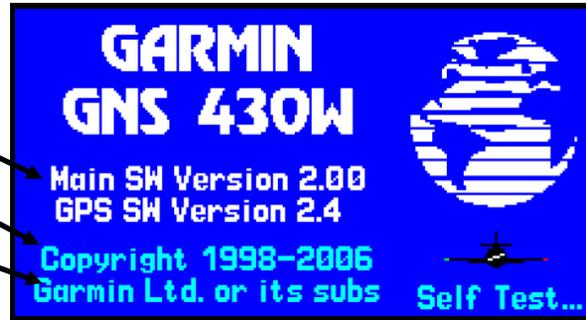
**Figure 34-49 GNS Model and Software Verification**
