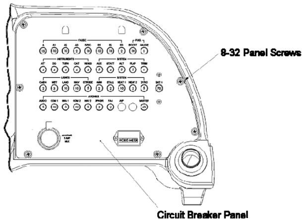
Figure 77-3 Circuit Breaker Panel
