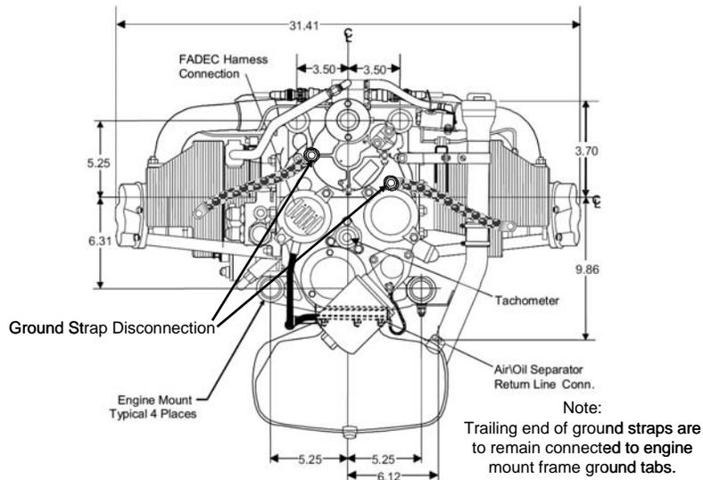
**Figure 71-5 Engine Ground Strap Disconnection**
