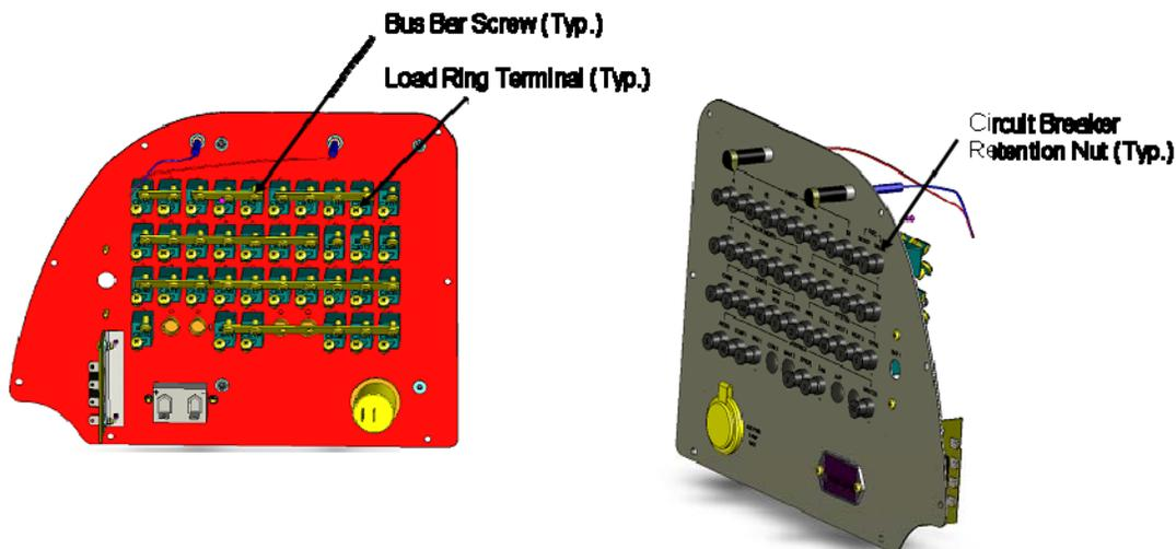
**Figure 24-16 Circuit Breaker Mounting Hardware**
