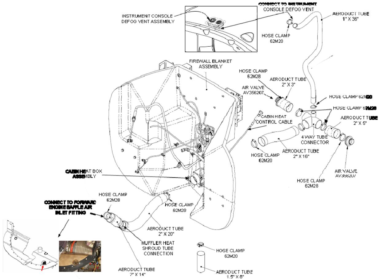
**Figure 21-3 Heating and Defogging System**
