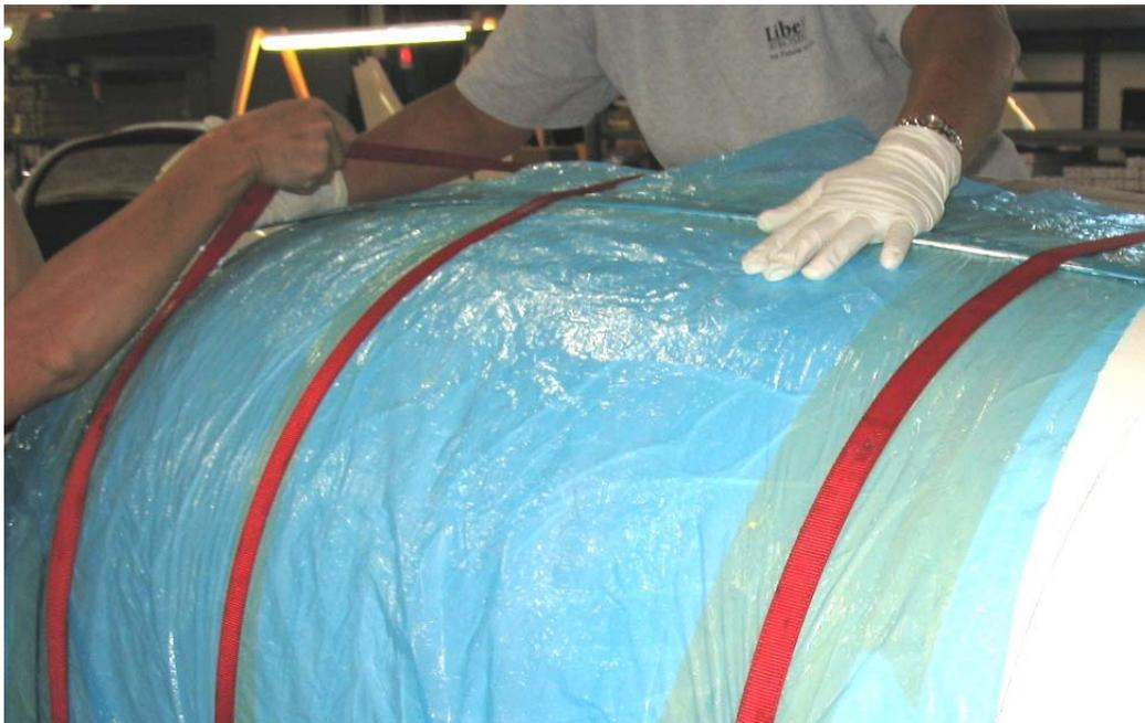
**Figure 56-9 Place the Metal Bands Under the Cloth Straps Over the Horizontal Upper Seam of the Doorframe and the Windscreen**
