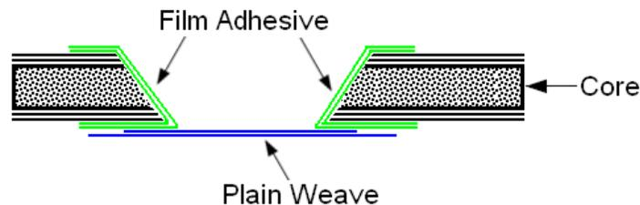
**Figure 51-19 Application of Staggered Plies of Plain Weave**
