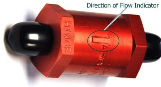
**Figure 28-13 Check Valve Showing The Arrow That Indicates The Direction Of The Flow – Arrow Points Aft**
