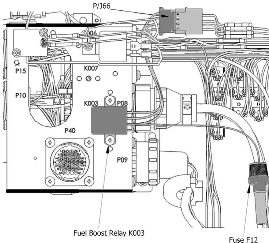
**Figure 28-17 Fuel Boost Relay Removal**
