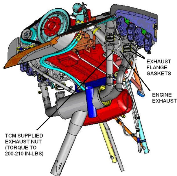
**Figure 78-3 Engine exhaust system**
