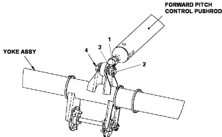
**Figure 27-63 Forward Pitch Control Pushrod to Yoke Assembly**
