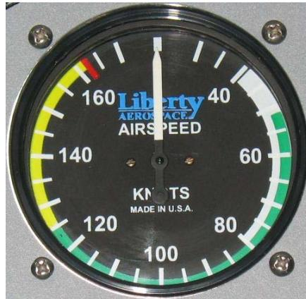
Figure 34-24 Airspeed Indicator
