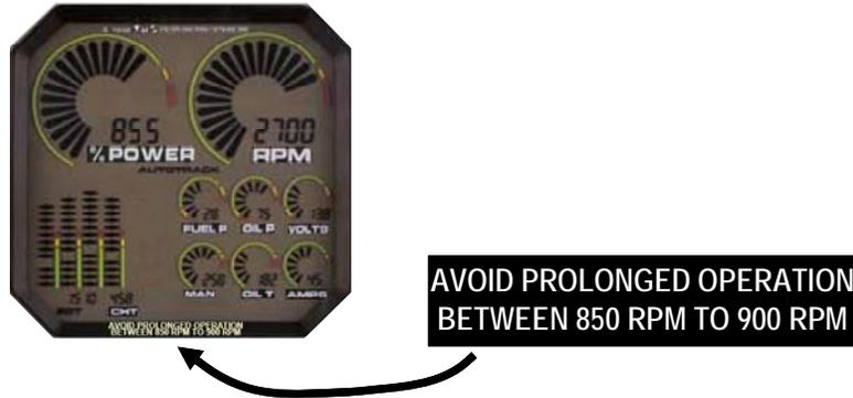
**Figure 11-24 RPM Limitation Placard**
