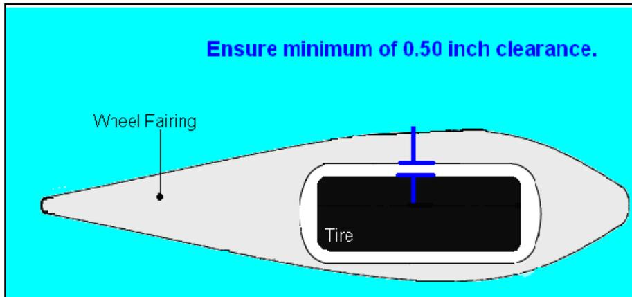
**Figure 32-12 Nose Fairing Tire Clearance**
