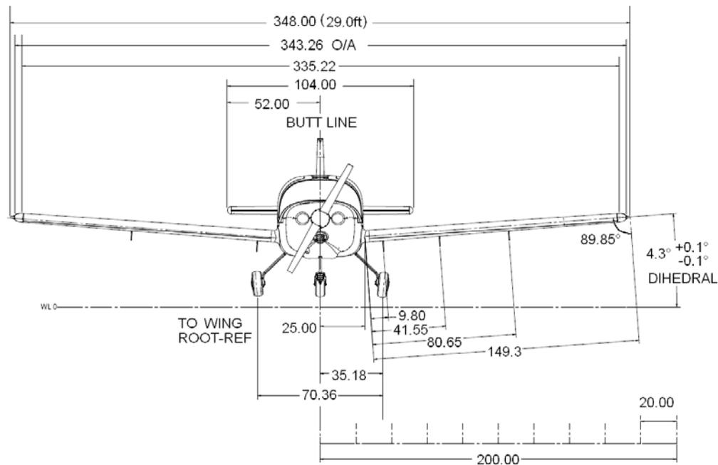
**Figure 03-3 Measurements from the Butt Line**
