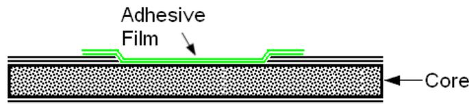
**Figure 51-30 Application of the Adhesive Film**
