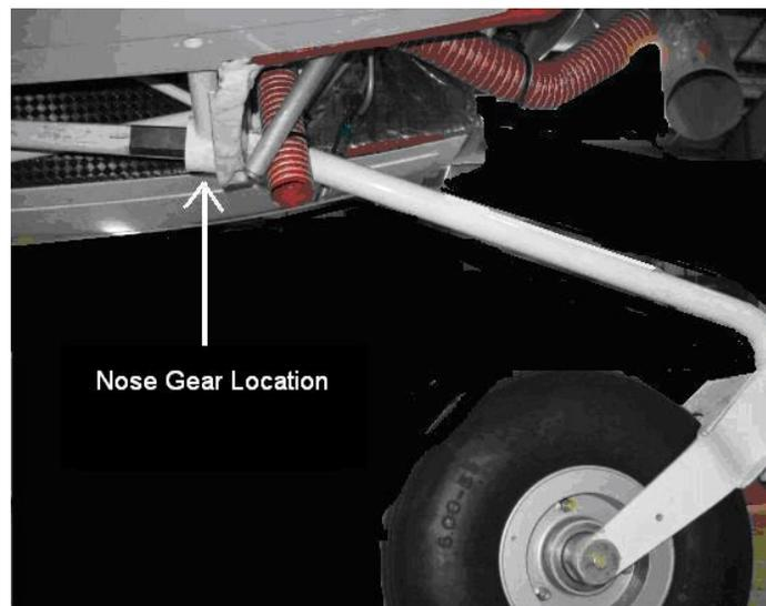
**Figure 07-5 Jacking Point for the Nose Gear**
