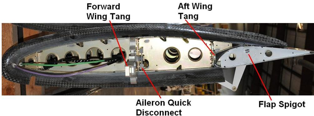
Figure 57-12 Wing Inspection Points
