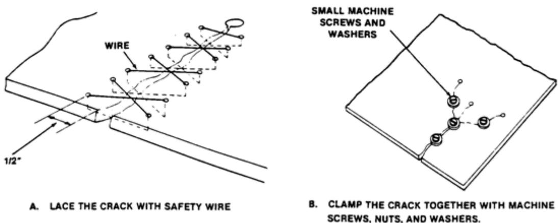
Figure 56-2 Temporary Repair of Cracked Forward Windscreen or Door Windscreen
