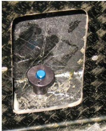
**Figure 52-4 Typical installation of the door hinge pin**
