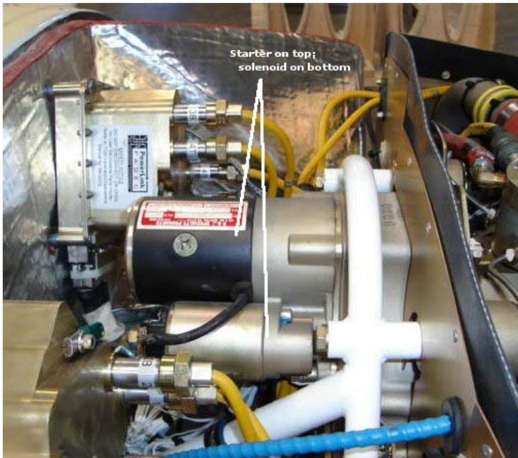
**Figure 80-1 Location of the Starter for the Engine**
