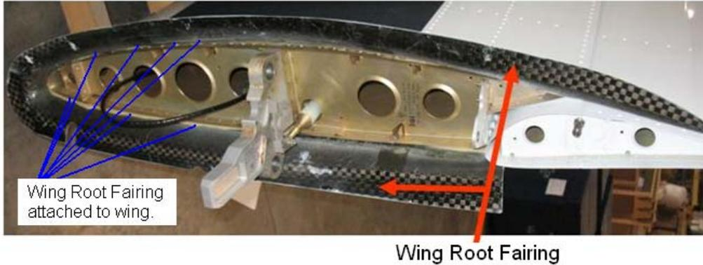
**Figure 57-24 Properly Secured Wing Root Fairing Attached to Wing Skin**
