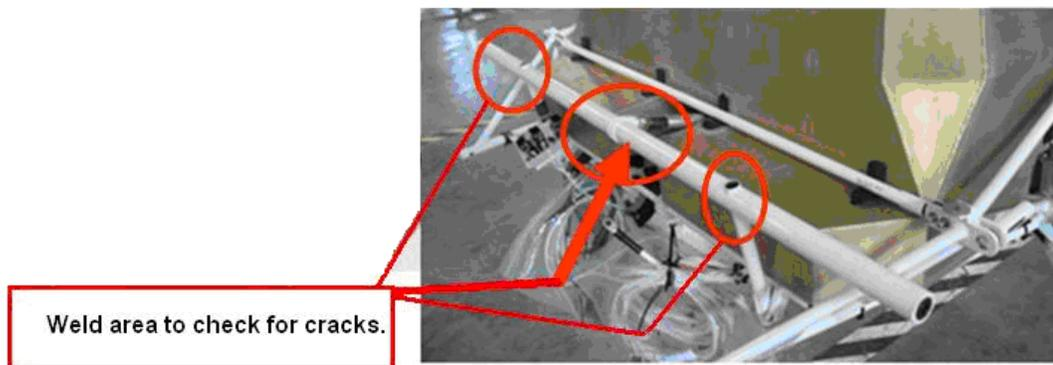
**Figure 27-79 Cracks Inspection Area**
