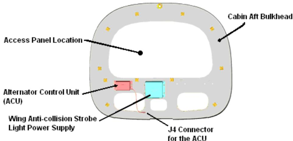
Figure 24-8 Alternator Control Unit (ACU) or Voltage Regulator Location
