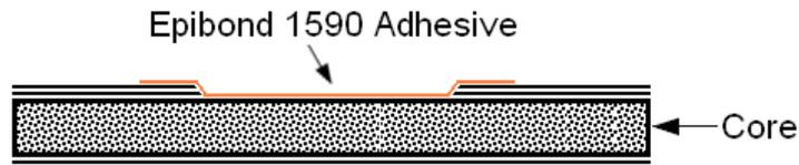
**Figure 51-34 Application of the Epibond Adhesive**
