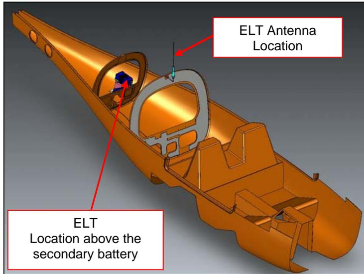
**Figure 25-13 Location of the Emergency Locator Transmitter and Antenna**
