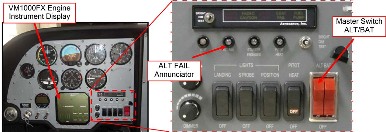
**Figure 24-2 Instrument panel showing the location of the ALT FAIL (Alternator Fail) indicator and the ALT/BAT switch**
