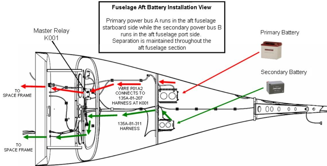
**Figure 24-3 Fuselage Aft Battery Installation View**
