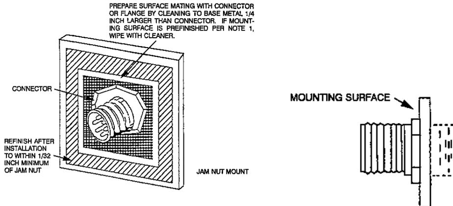
Figure 51-59 Bulkhead Connectors
