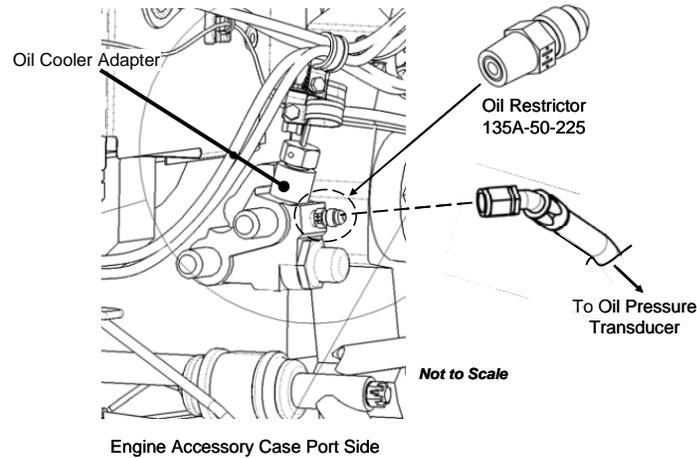
**Figure 71-8 Oil Pressure Line Disconnection**
