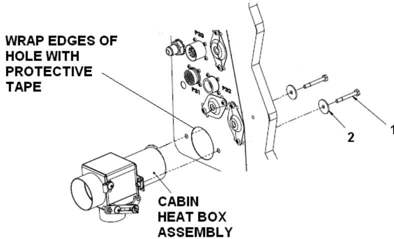
**Figure 71-31 Cabin Heat Box Assembly Removal and Installation**
