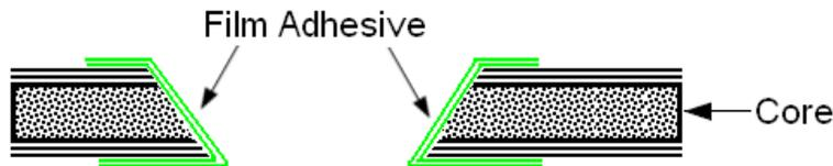
**Figure 51-18 Application of the Film Adhesive**
