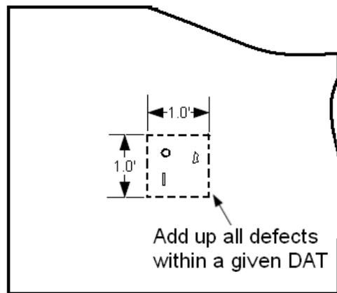
Figure 51-2 Example Application of Laminate DAT
