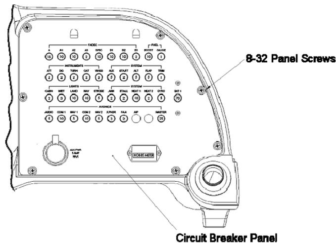
**Figure 24-14 Circuit Breaker Panel**
