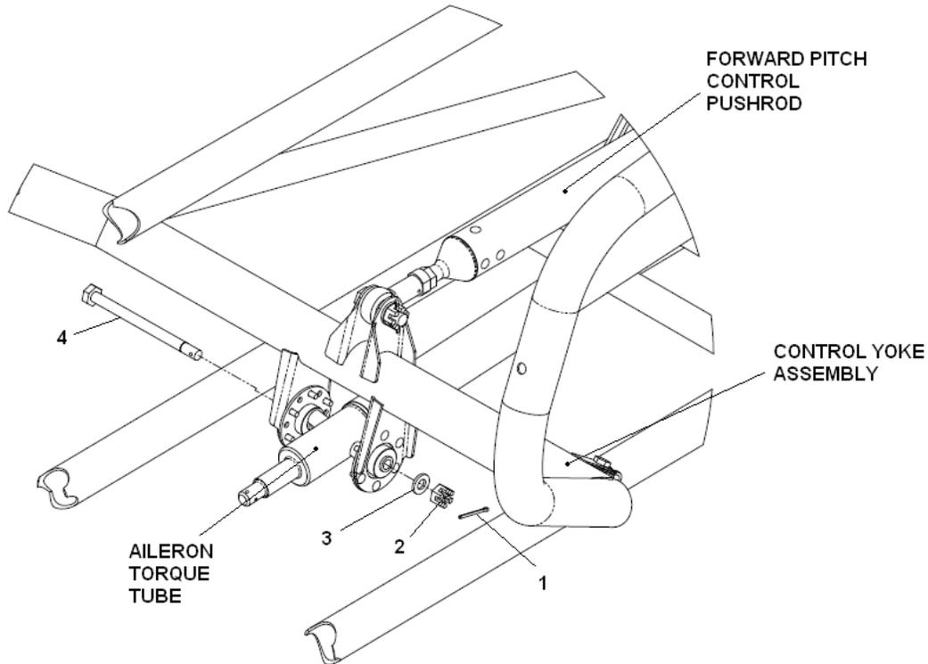
**Figure 27-62 Control Yoke Removal and Installation**
