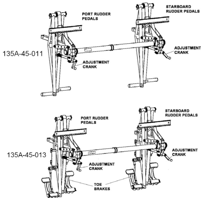
**Figure 27-24 Rudder Pedal Assemblies**
