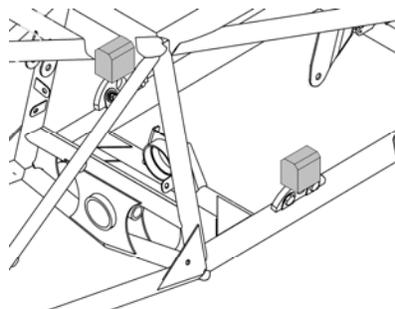
**Figure 27-87 Aileron Neutral Block Placement**
