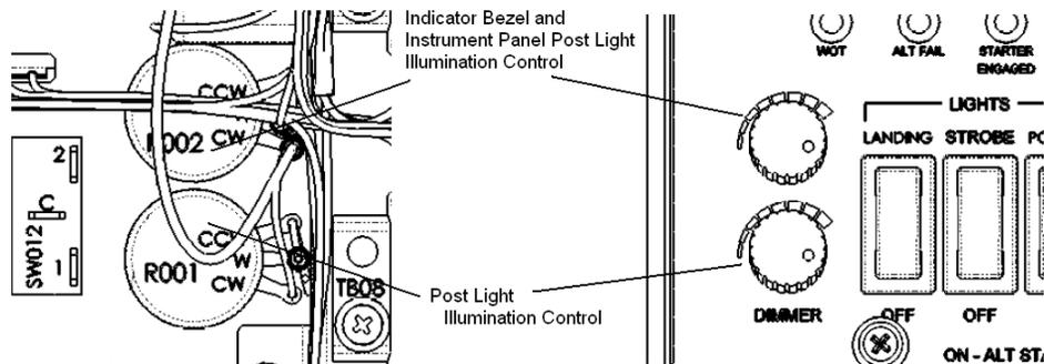
**Figure 33-1 Location of the Dimmer Controls for the Post Lights**
