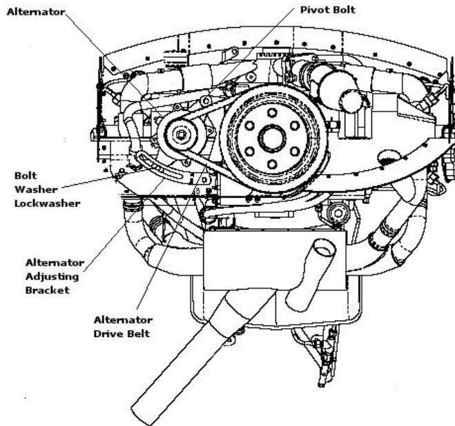
**Figure 72-2 Engine Front View**
