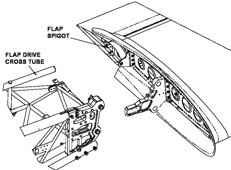
**Figure 27-67 Flap Drive Cross Tube and Spigot**
