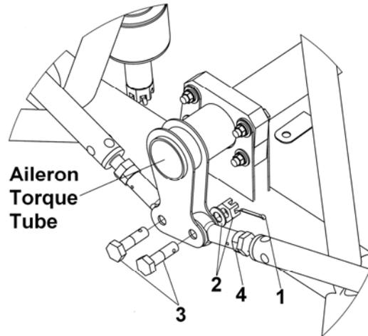
**Figure 27-19 Aileron Inboard Pushrod to Torque Tube**
