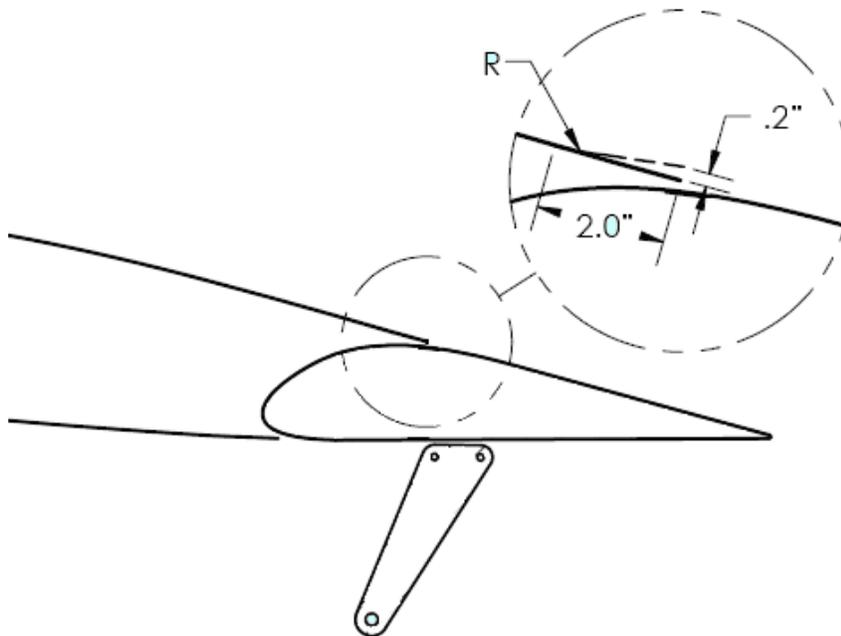
Figure 27-69 Opening “C” Channel of Wing-Flap Closeout
