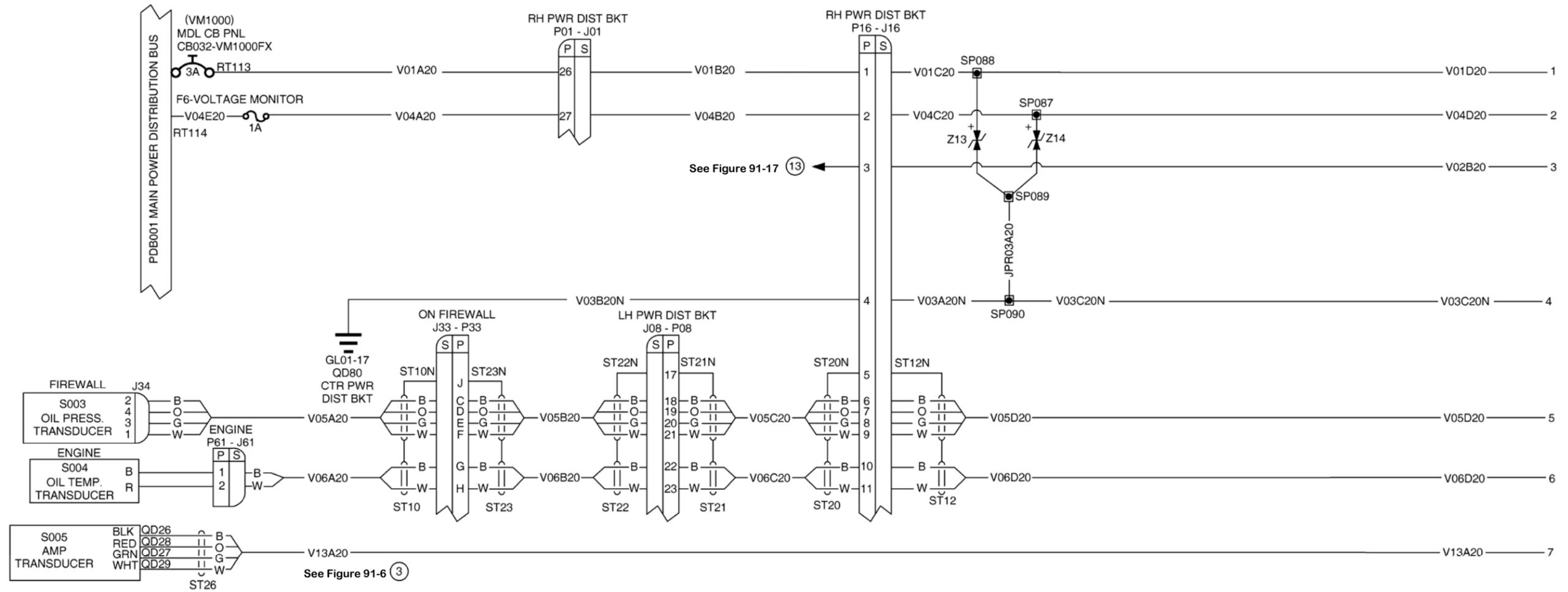
Figure 91-12 VM1000FX Engine Instrument System (1 OF 2)
