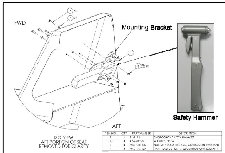
**Figure 25-4 Safety Hammer Location and Mounting**
