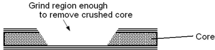
**Figure 51-5 Section of the Composite After Grinding**
