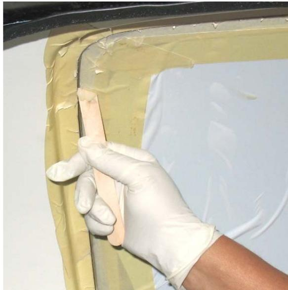
**Figure 56-11 Use a Tongue Depressor to Remove the Excess Adhesive from the Interior Edge Between the Doorframe and the Windscreen**
