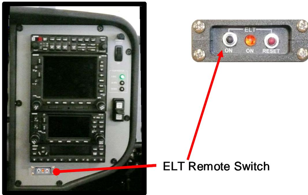
**Figure 25-14 ELT Remote Switch Location**
