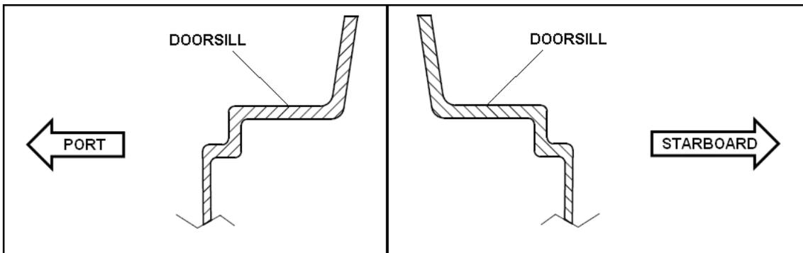
**Figure 08-5 Doorsills Used in Longitudinal Leveling**
