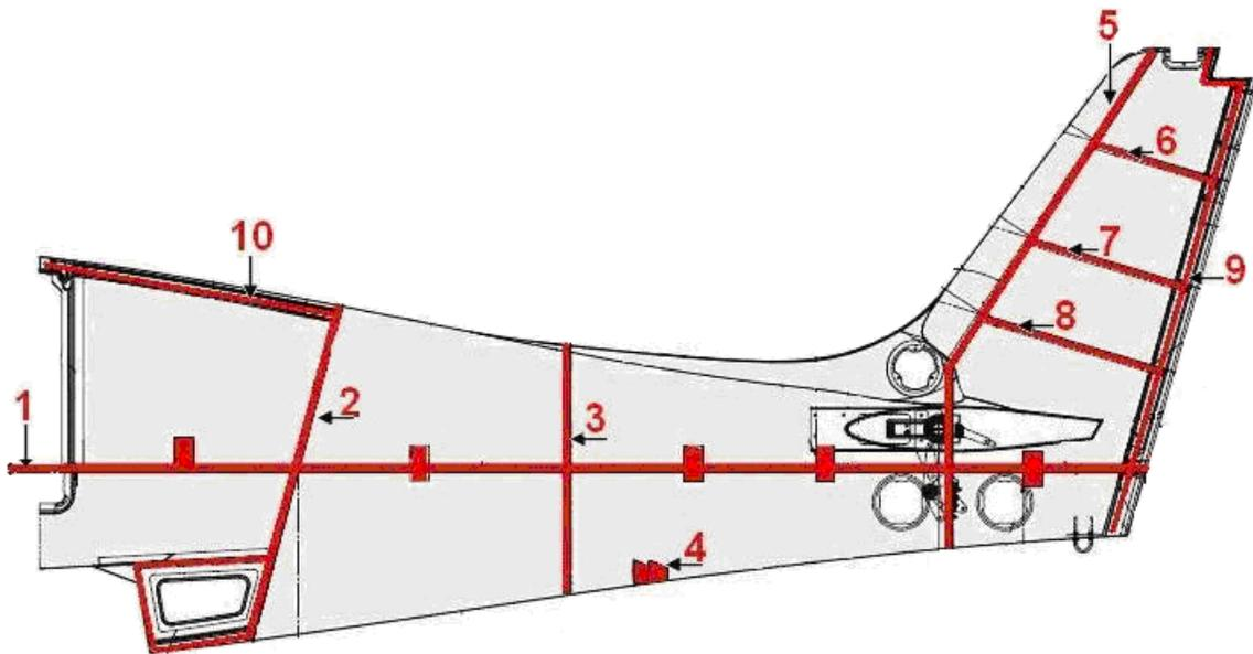
**Figure 04-4 Upper and Lower Fuselage Bond Lines**
