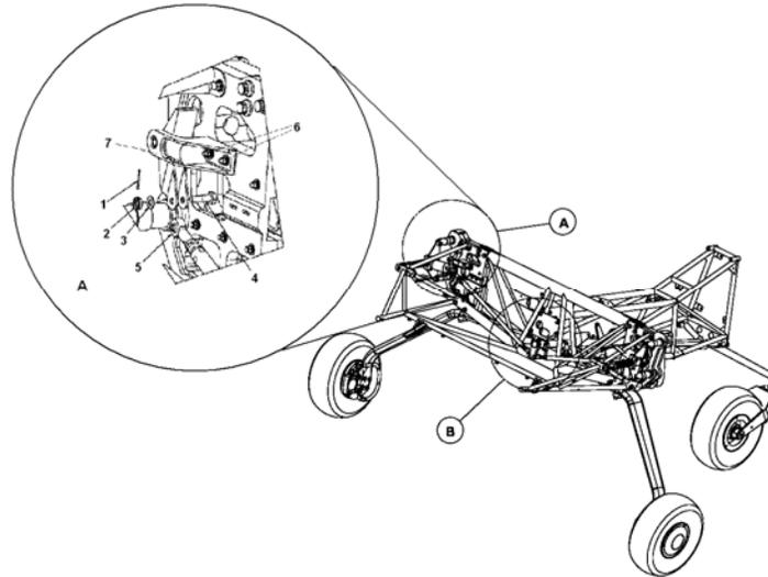
**Figure 27-17 Aileron Inboard Quick-disconnect Device**
