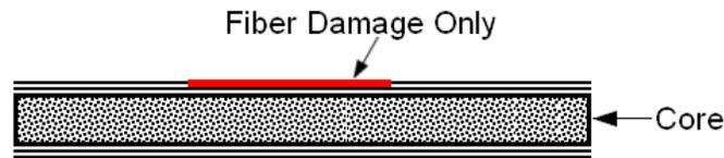
**Figure 51-36 Cross Section of the Damaged Area**
