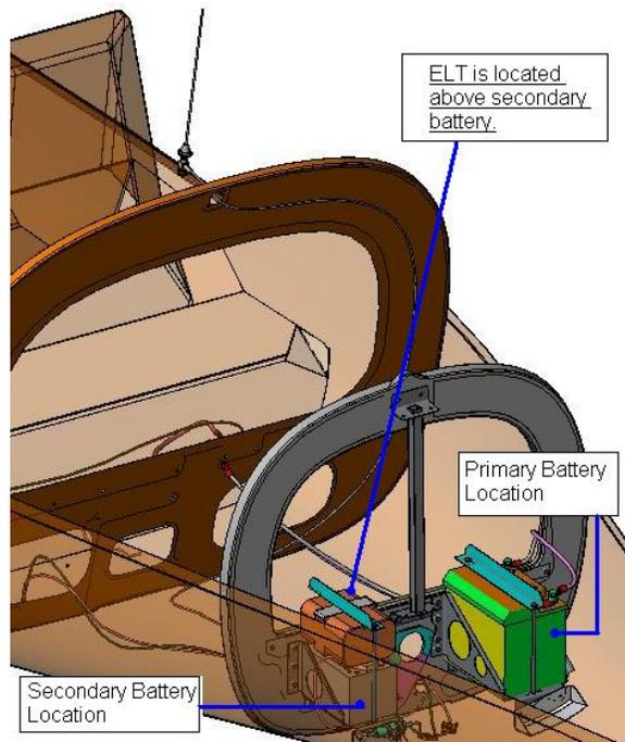
Figure 24-11 Location of Batteries Aft of Baggage Closeout Area
