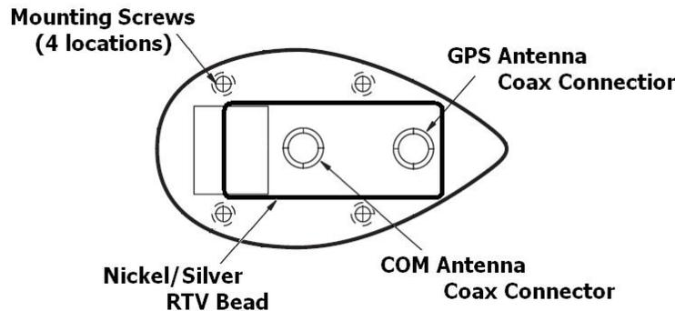
**Figure 23-17 COM/GPS Antenna Conductive Sealant**
