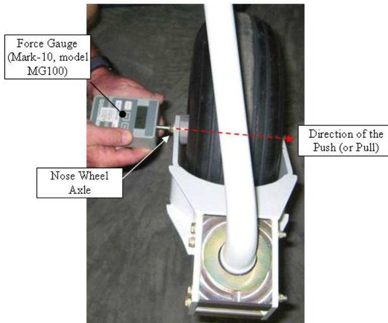
**Figure 32-46 Nose Wheel Shimmy Load Test**
