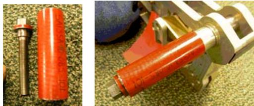
**Figure 57-7 Extractor Wing Pin Tool Kit**
