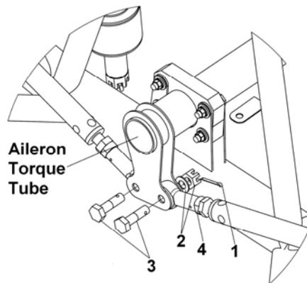
**Figure 27-18 Aileron Inboard Pushrod to Torque Tube**
