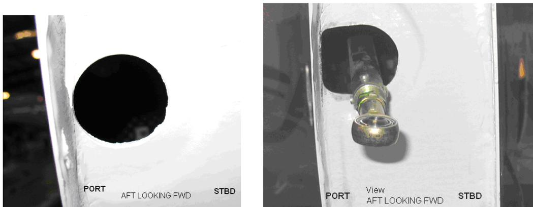
Figure 27-44 Before and After Extending the Pass-thru Hole
