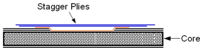
**Figure 51-35 Application of the Staggered Plies of Plain Weave**
