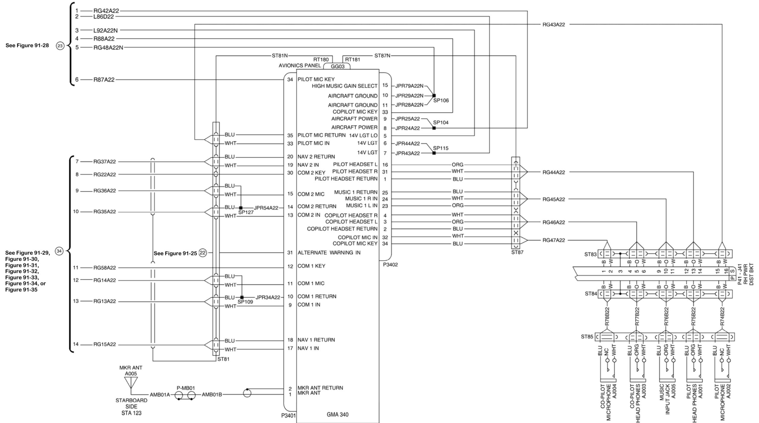
Figure 91-36 Avionics (Audio Panel)
