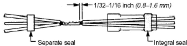
**Figure 20-25 Crimp Splice Multiple Wires**
