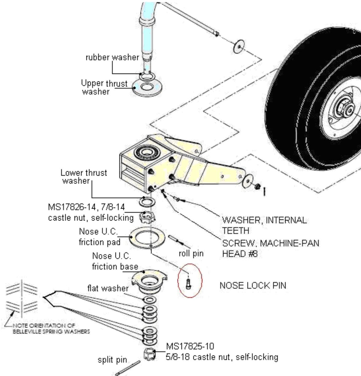
**Figure 32-43 Exploded View of Nose Wheel Steering Assembly**
