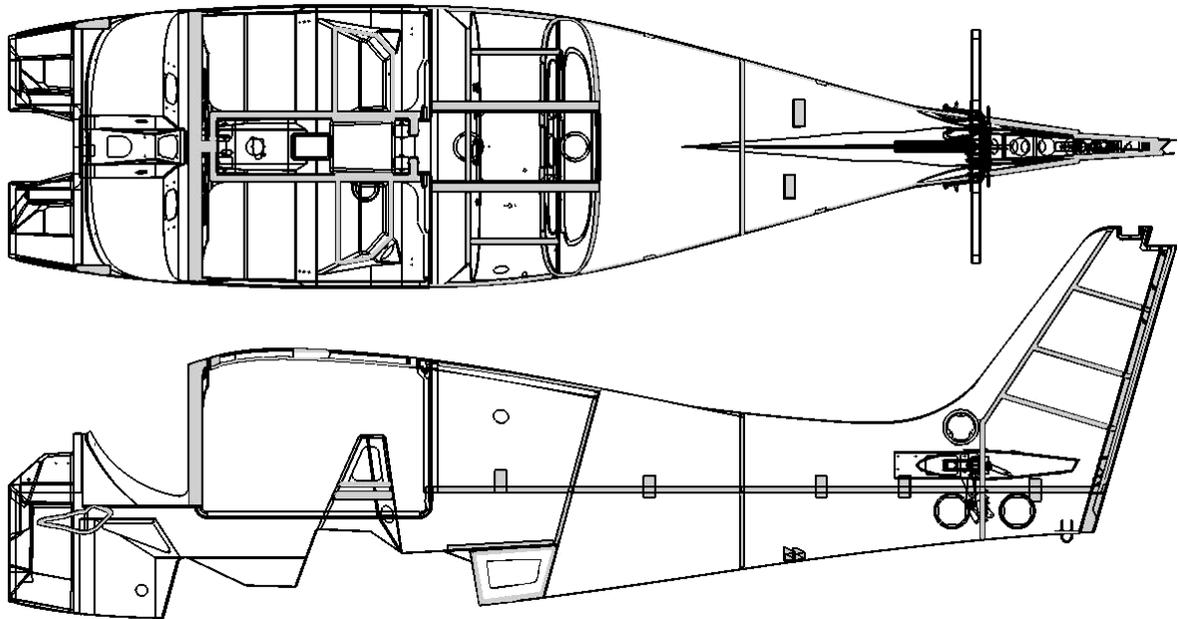
**Figure 51-40 The Bond-Line Locations (in Gray) On The Airplane’s Fuselage**
