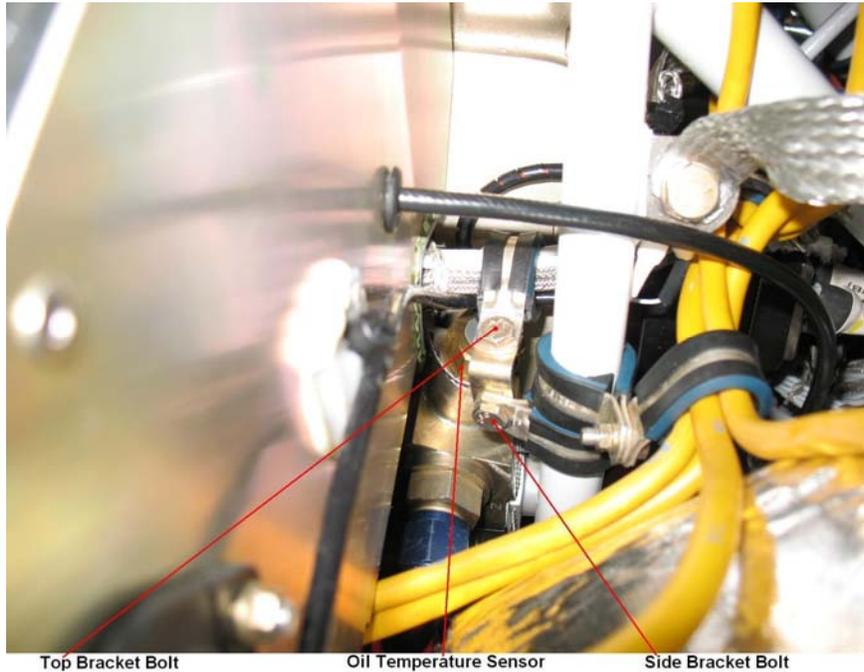
**Figure 79-10 Location of the Oil Temperature Sensor**
