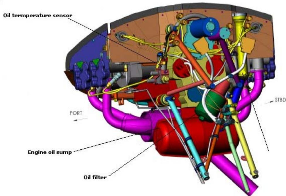
Figure 79-1 View Of Engine Oil Components, from Aft Looking Forward
