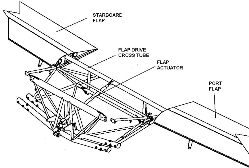
**Figure 27-64 Flaps Control Circuit Geometry**
