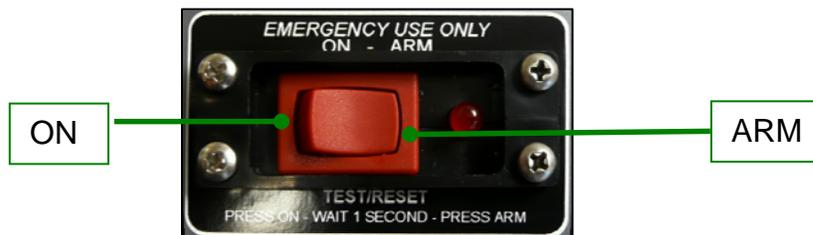
**Figure 25-35 Remote Switch – 406 MHz Transmitter Test**
