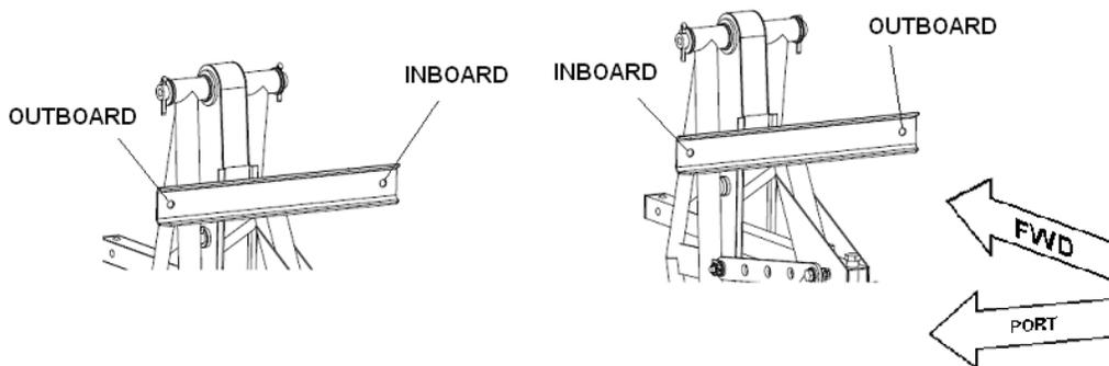
**Figure 27-40 Rudder Pedal Assembly Mounting Bolt Locations**
