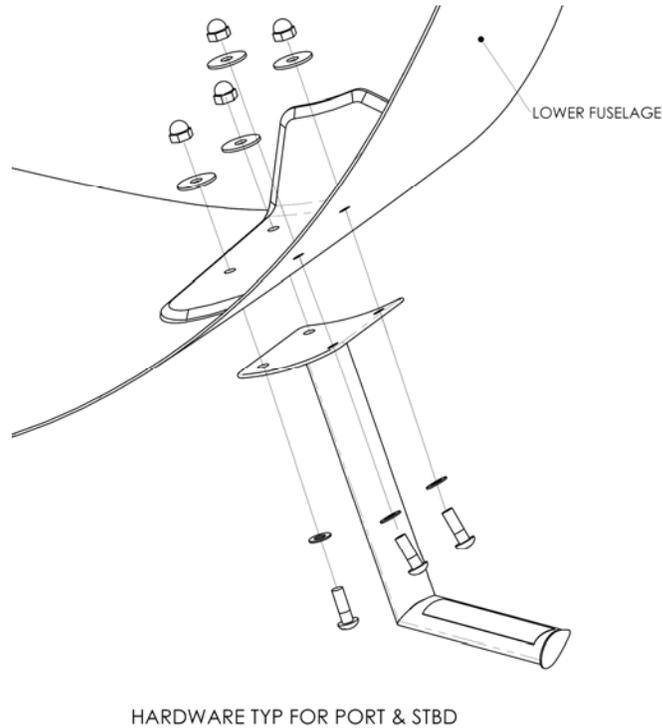
**Figure 53-30 Footstep Installation**
