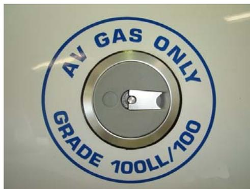
**Figure 53-27 Fuel Tank Filler Access or Gas Cap**
