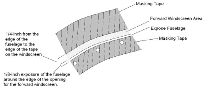
**Figure 56-19 Detail showing the Masked-off Area of the Forward Windscreen**
