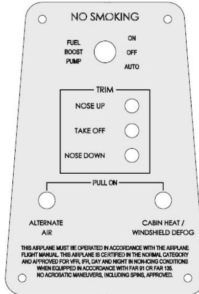
**Figure 11-3 Example of one of the placards (center console placard) that is available with different languages**
