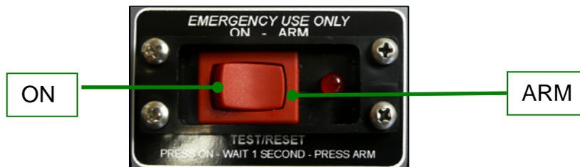
**Figure 25-34 Remote Switch – 121.5 MHz Transmitter Test**
