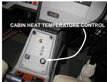
**Figure 21-10 Center Console Cabin Heat Temperature Control**
