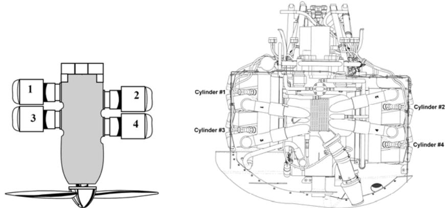
**Figure 61-1 TCM IO-240-B Cylinder Assignment**
