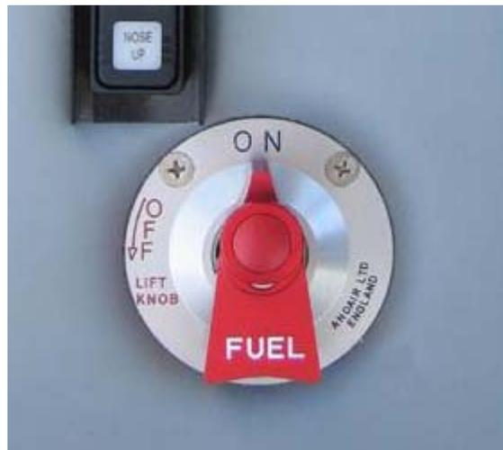
**Figure 28-9 Fuel Switch Center Console**
