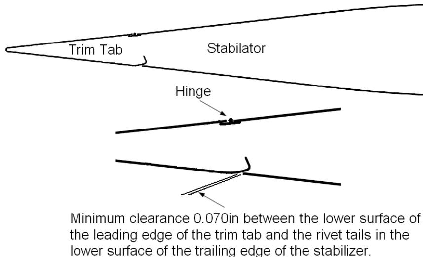
Minimum clearance 0.070in between the lower surface of the leading edge of the trim tab and the rivet tails in the lower surface of the trailing edge of the stabilizer.
