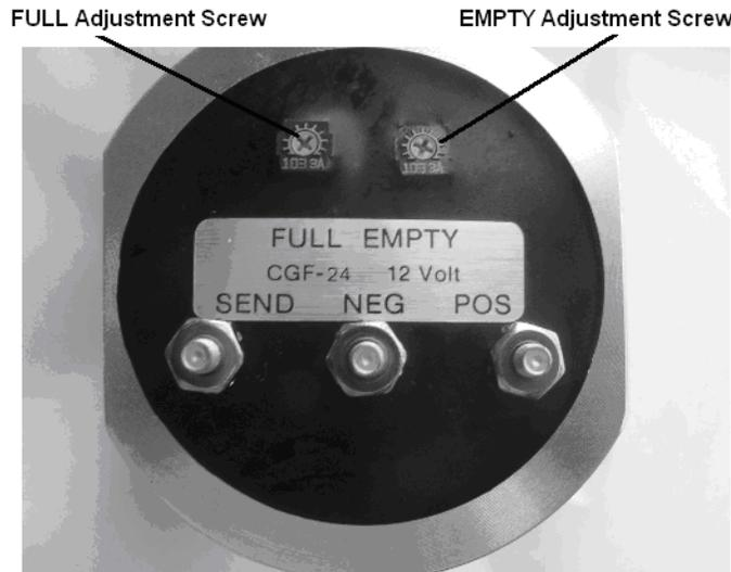
Verify correct control is being adjusted. Make only small adjustments.
