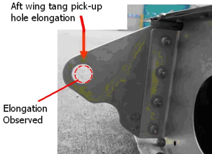
**Figure 57-16 Aft Wing Pick-Up Elongation**
