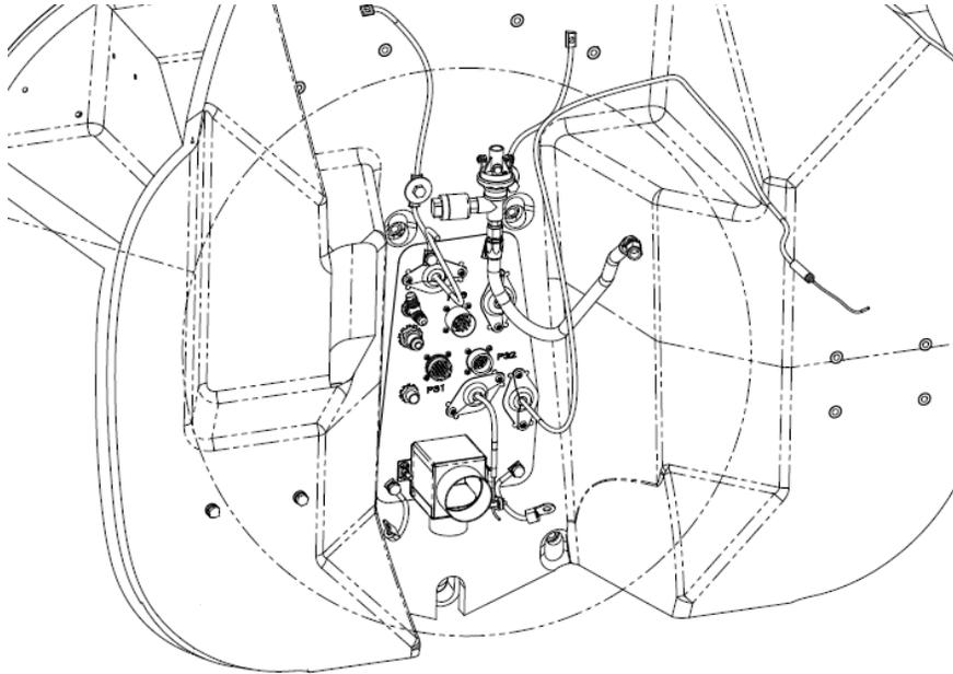
Figure 71-39 Firewall Interface Feed-through Panel
