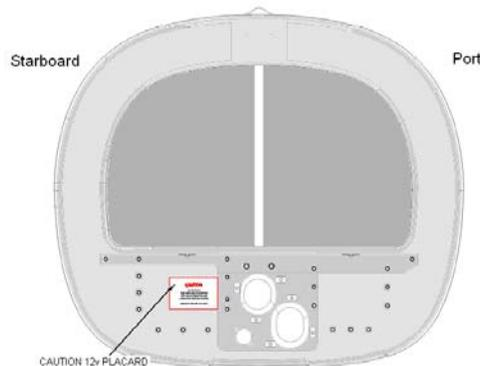
Figure 11-14 Aft side of the Mid Fuselage Bulkhead showing location of placard
