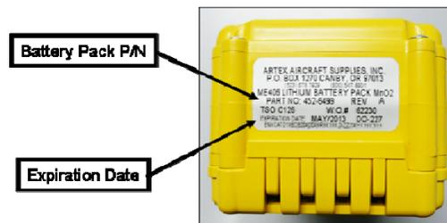
**Figure 25-29 Battery Identification Placard**
