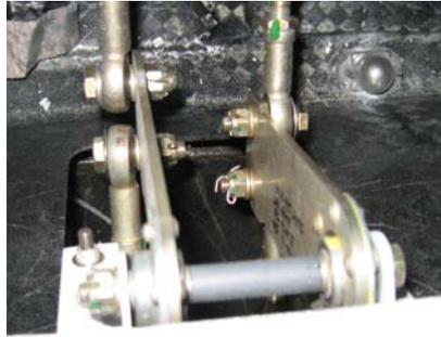
**Figure 53-23 FWD stabilizer and rudder pushrod and their bearings**
