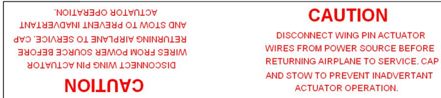
Figure 11-31 Details of the Caution Label on the Ball Drive Actuator
