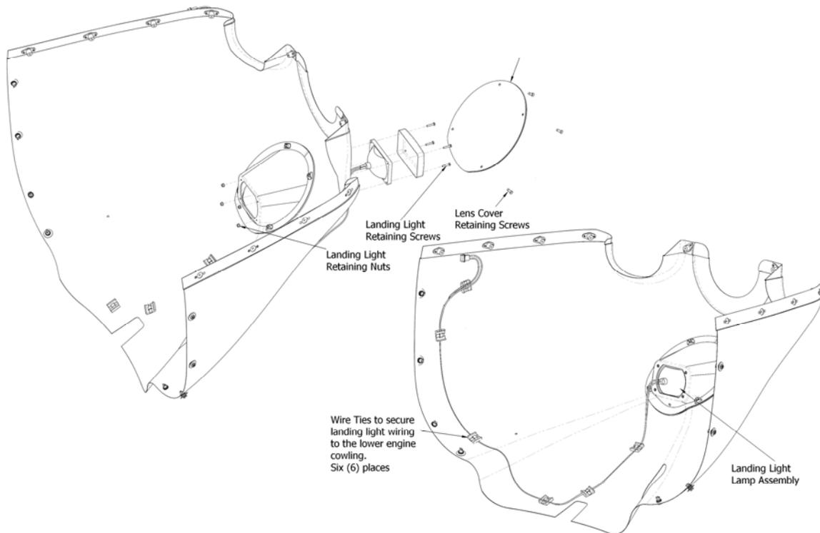
**Figure 33-12 Landing Light Installation**
