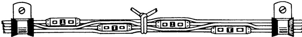
**Figure 20-8 Staggered Splices in Wire Bundle**
