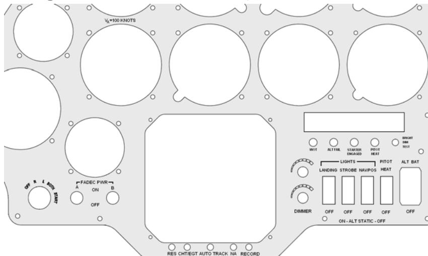
Figure 11-23 Enlarge View of the Instrument Panel P/N 135A-80-311
