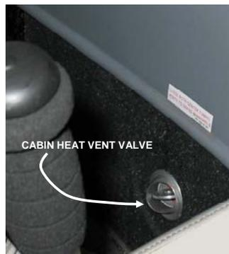
**Figure 21-11 Cabin Heat Vent Valve Installation**
