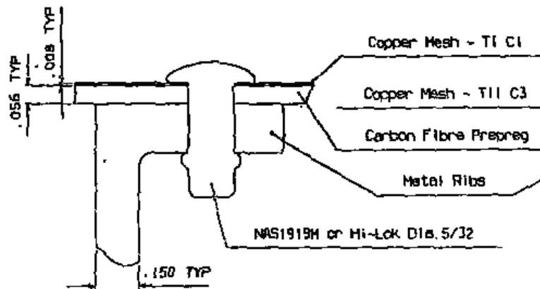
Figure 51-61 Composite to Metal Bonding
