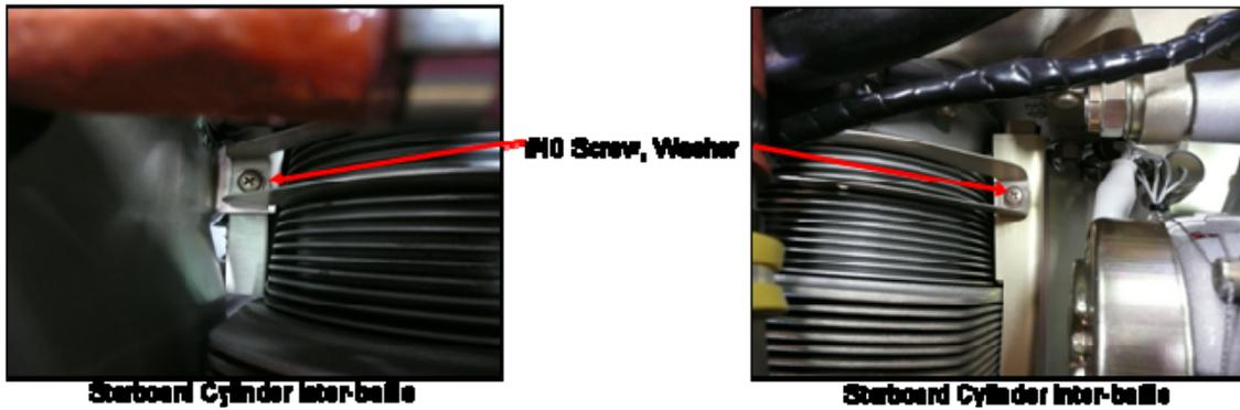
**Figure 72-9 Cylinder Inter-Baffle Screws**
