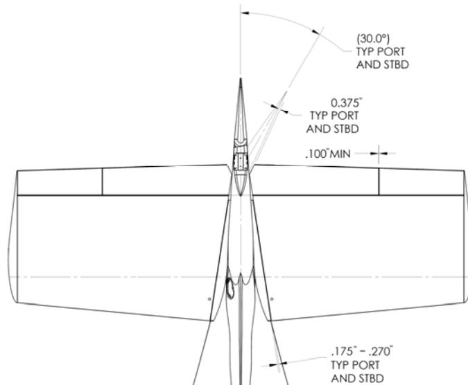
**Figure 27-95 Tail Section Measurements**
