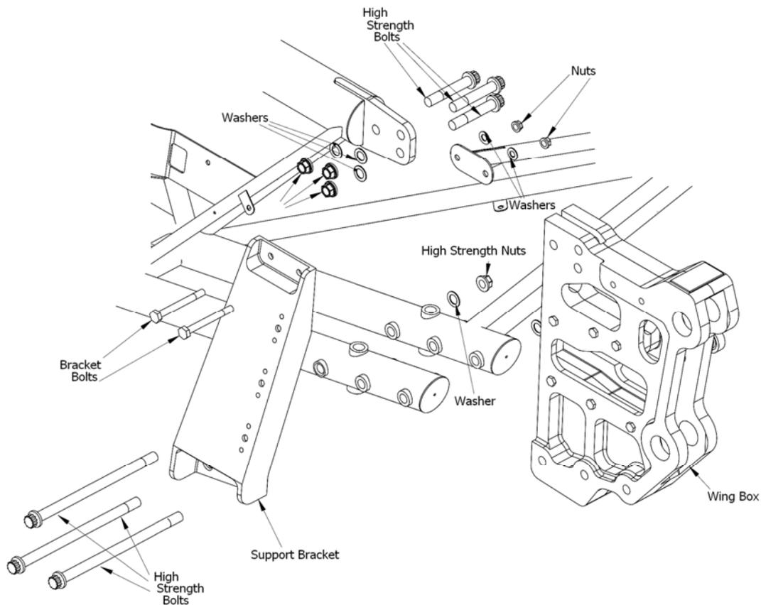
Figure 57-18 Wing Box Explodes View
