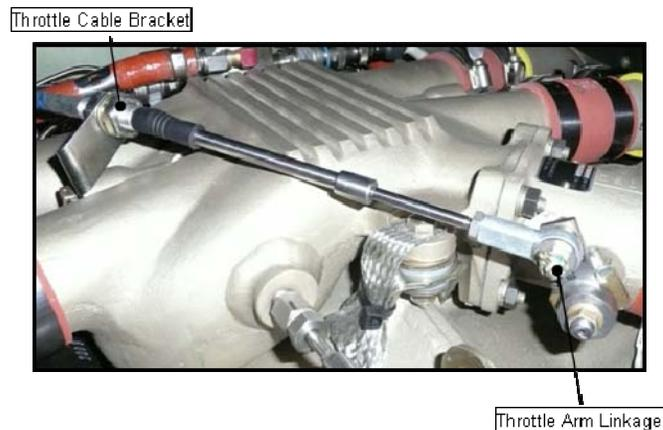
**Figure 72-10 Throttle Cable and Bracket**
