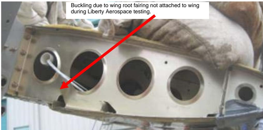
**Figure 57-25 Buckling Observed During Strength Test**
