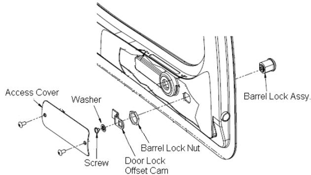
**Figure 52-9 Exploded View of Door Lock Assembly(Port Side Shown)**
