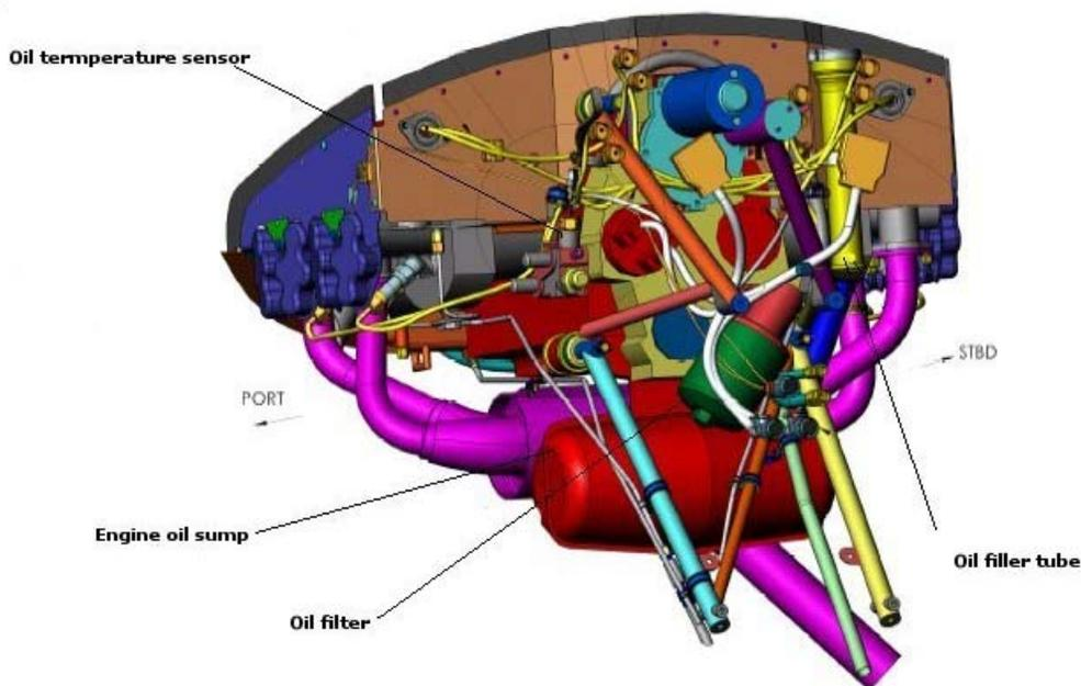
Figure 72-14 Cut-A-Way View of Engine and Oil Related Components
