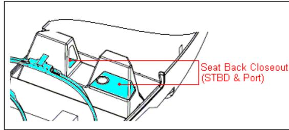
**Figure 53-9 Seat Back Closeout Access Panels**
