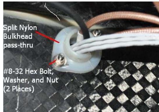
**Figure 25-11 Split Nylon cable pass-thru**
