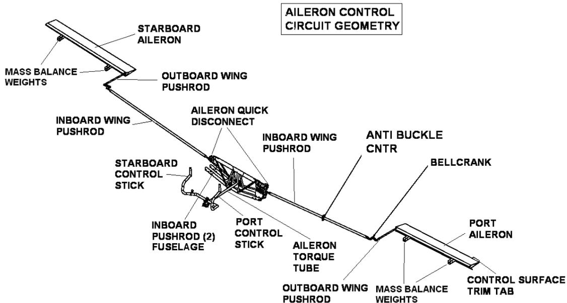
**Figure 27-2 Aileron Control Circuit Geometry**
