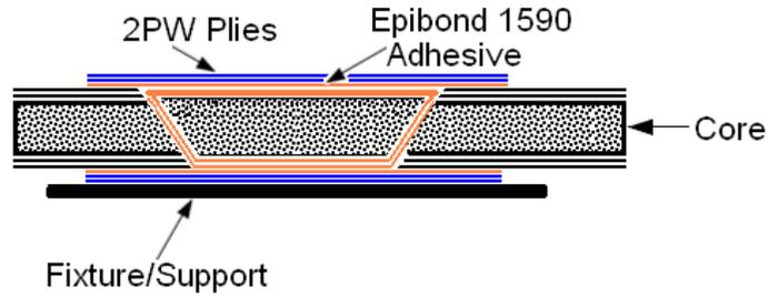
**Figure 51-15 Insertion of the New Foam Core and Application of the Epibond Adhesive and Staggered Plies of Plain Weave**
