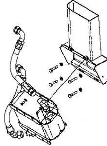
Figure 79-2 Exploded View of Engine Oil Cooler Installation
