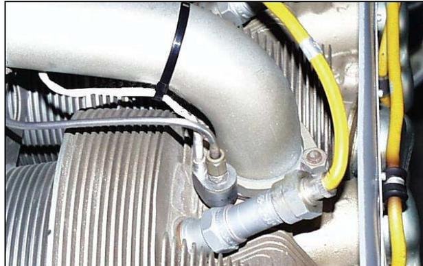
**Figure 71-42 High Voltage Harness Spark Plug Attachment**
