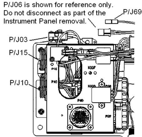
**Figure 34-13 Left Hand Side of the Power Distribution Harness Assembly**
