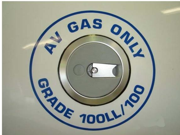
Figure 12-2 Fuel Specification Labeling
