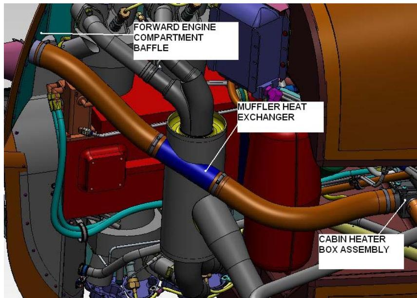
**Figure 78-2 Muffler Heat Exchanger to Cabin Heater Box**
