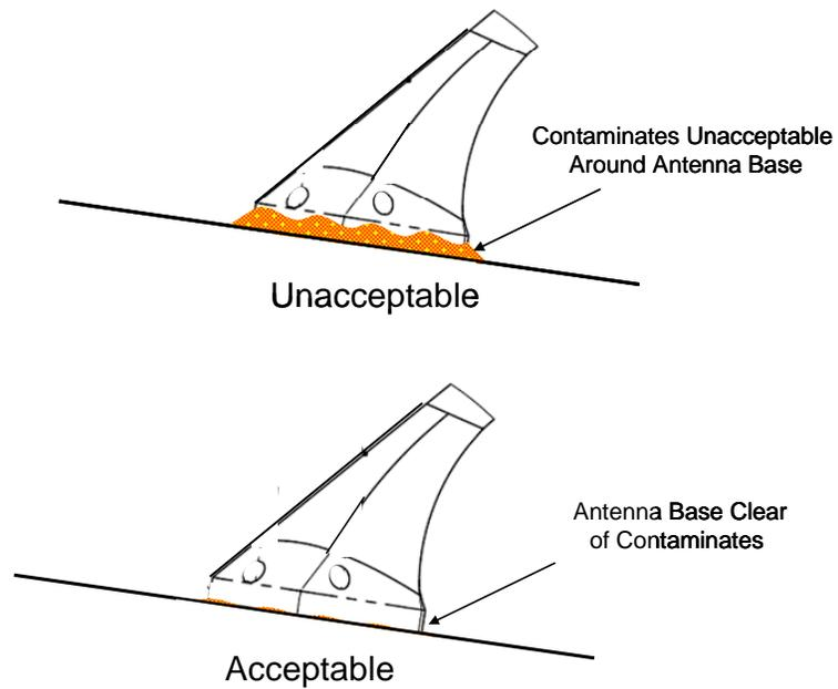
**Figure 23-18 Antenna Contamination Inspection**
