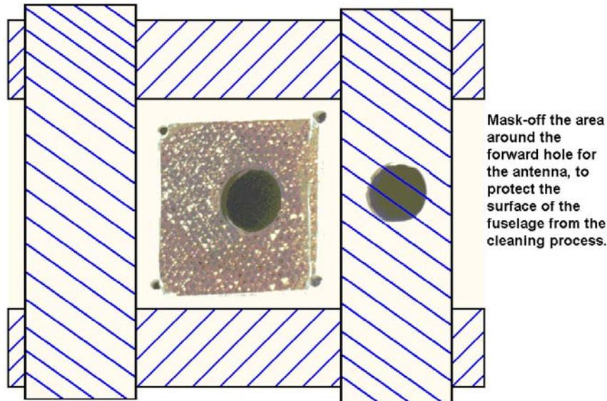
**Figure 23-16 Area of the Fuselage to Mask-Off to Protect the Fuselage**
