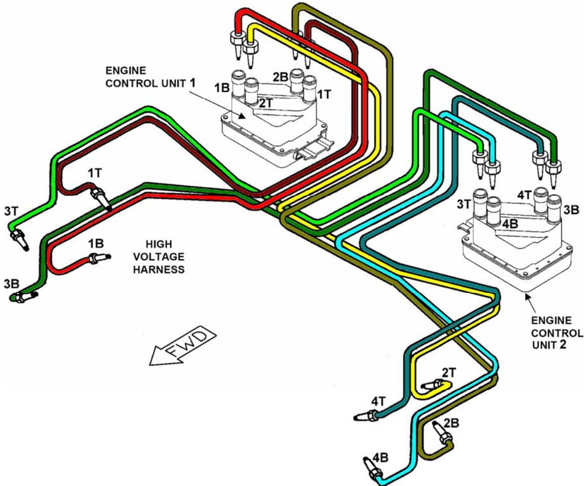
**Figure 74-1 ECU Connections to the Spark Plugs**
