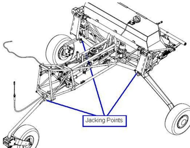
Figure 07-3 Jacking Points on the Space Frame
