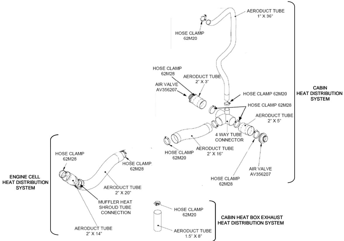
**Figure 21-2 Heating and Defogging Distribution System**
