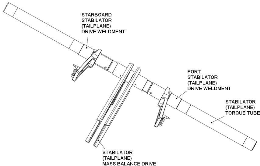
Figure 55-10 Stabilator Torque Tube
