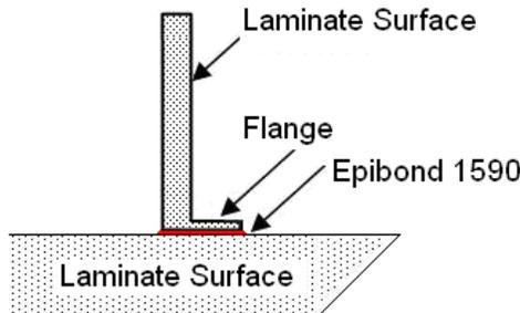
**Figure 04-2 Flange Joint**
