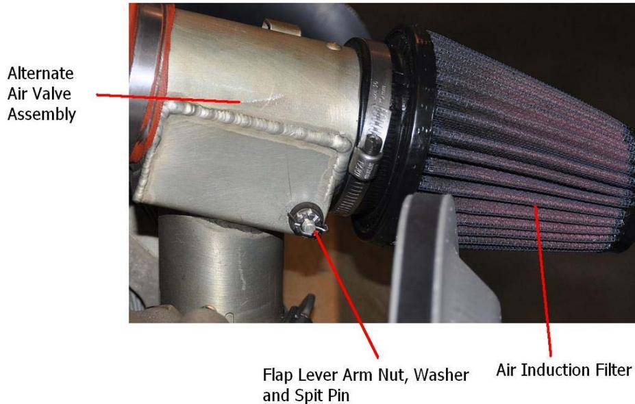
**Figure 71-48 Alternate Air Valve Assembly**
