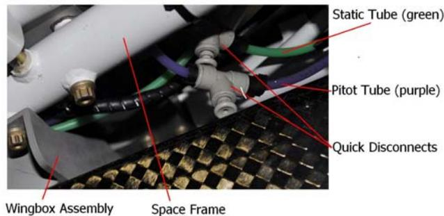
**Figure 30-2 Pitot and Static Quick Disconnects**
