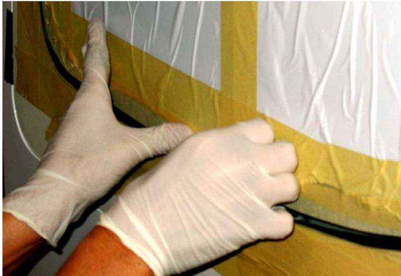
**Figure 56-7 Fitting the Windscreen into the Doorframe**
