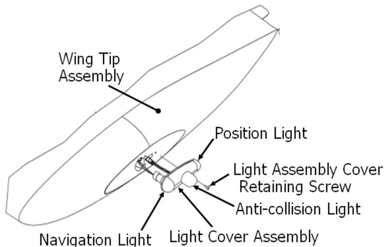
**Figure 33-10 Wing Tip Assembly**
