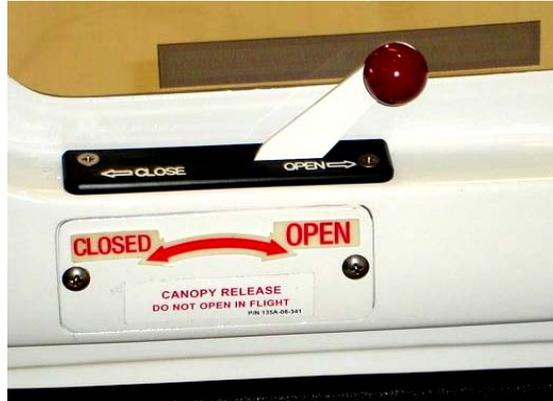
Figure 52-3 Interior Door Latching Mechanism (Starboard Side Shown)
