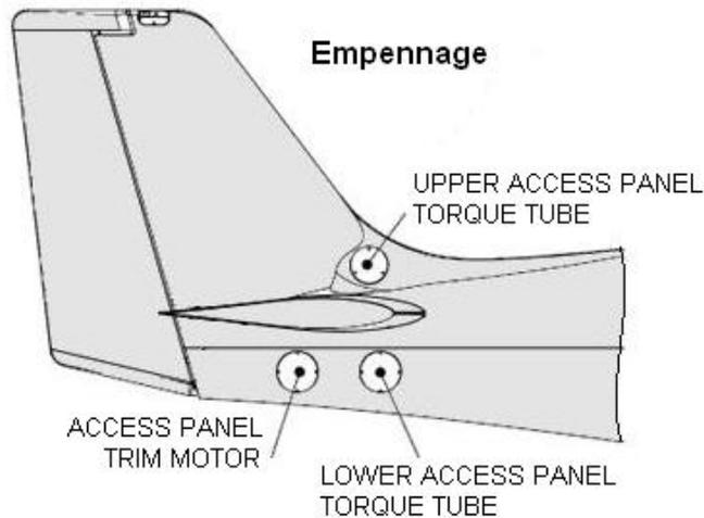
**Figure 53-26 Starboard Access Panels**
