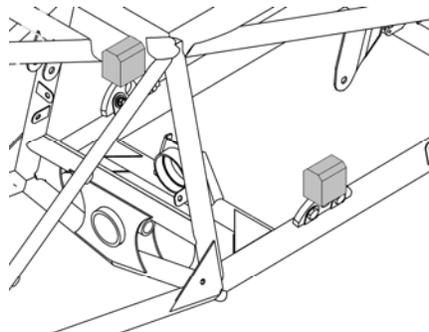
**Figure 27-83 Aileron Neutral Blocks Placement**
