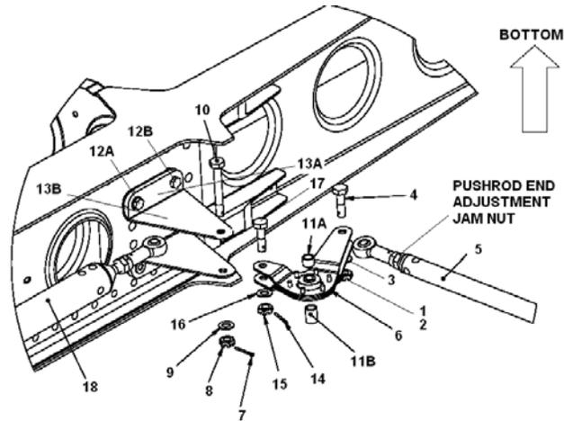
**Figure 27-9 Aileron Wing Bell-crank Assembly**
