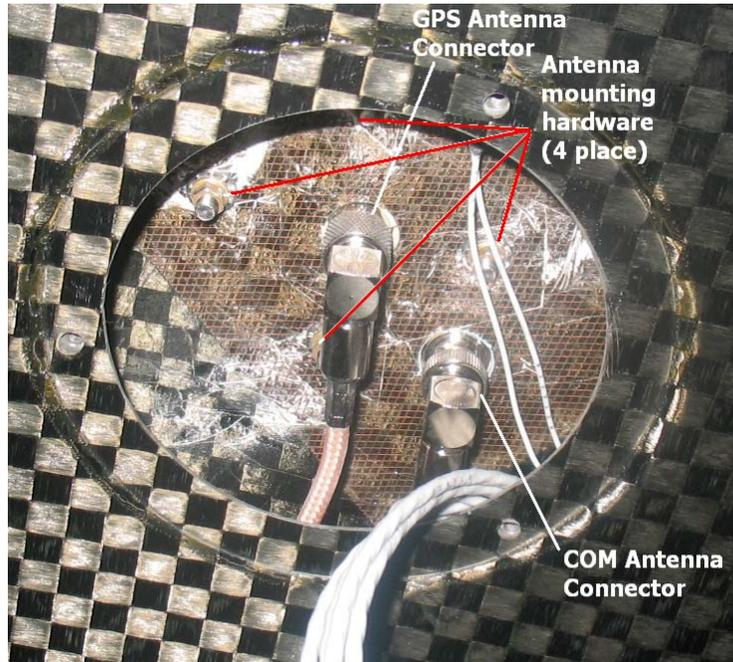
**Figure 23-15 View of the Underside of the COM/GPS Antenna**
