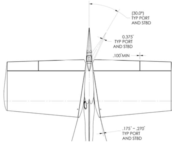
**Figure 27-92 Tail Section Clearance Measurements Between Horizontal Stabilator and the Vertical Stabilizer**
