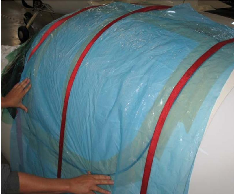
**Figure 56-8 Placing the Straps Over the Mold Release Paper**
