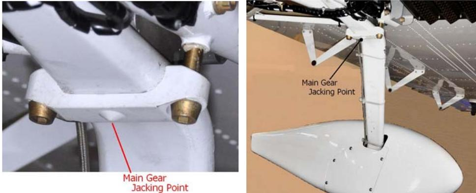
**Figure 07-4 Main Gear Jacking Points**
