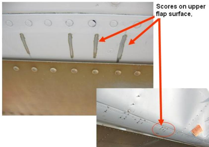
**Figure 27-77 Metal Scores on Flap Surfaces**
