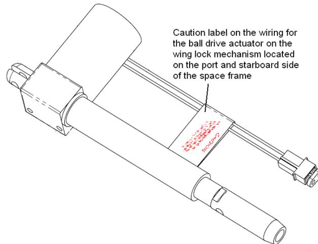
Figure 11-30 Ball Drive Actuator Showing the Location of the Caution Label
