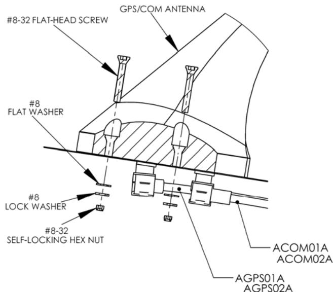
**Figure 23-14 CI 2580-200 COM/GPS Antenna Installation details**
