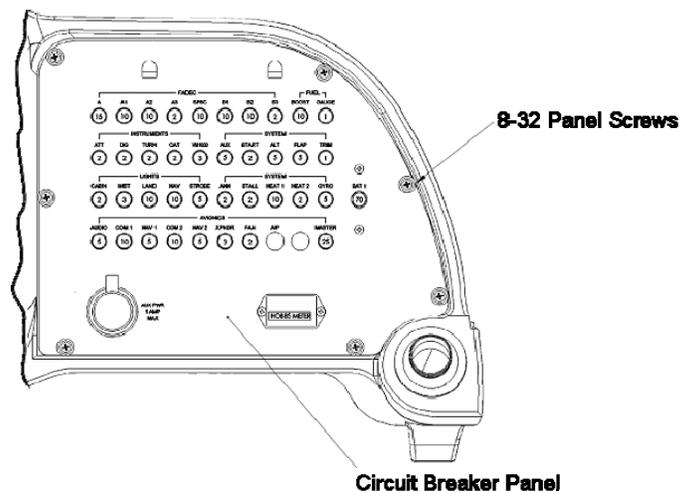
Figure 77-1 Circuit Breaker Panel
