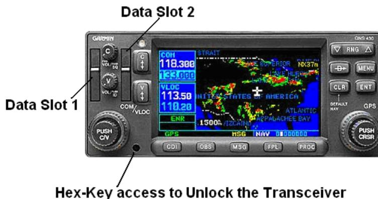
**Figure 23-4 GNS 430 Face Plate Key Slot**
