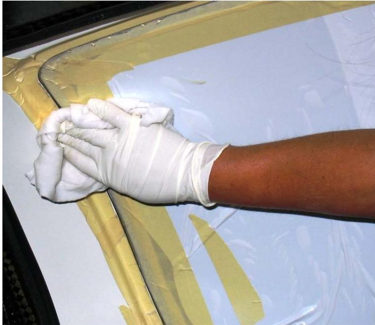
**Figure 56-12 Clean the Interior of the Joint Between the Doorframe and the Windscreen with a Clean Cloth Moistened with Alcohol**
