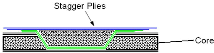
**Figure 51-8 Application of the New Staggered Plies of Plain Weave**
