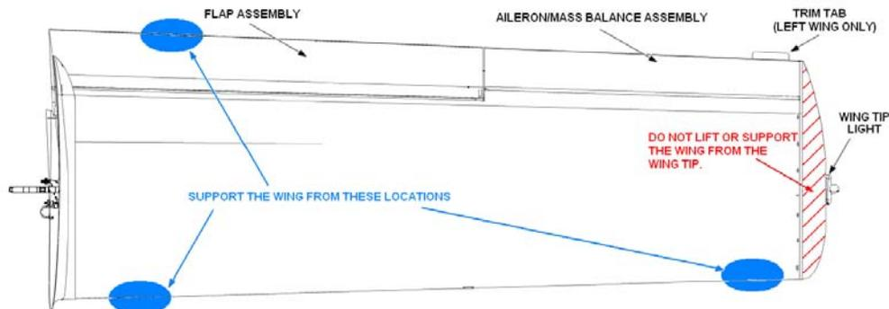
**Figure 57-9 Wing Handling Positions**
