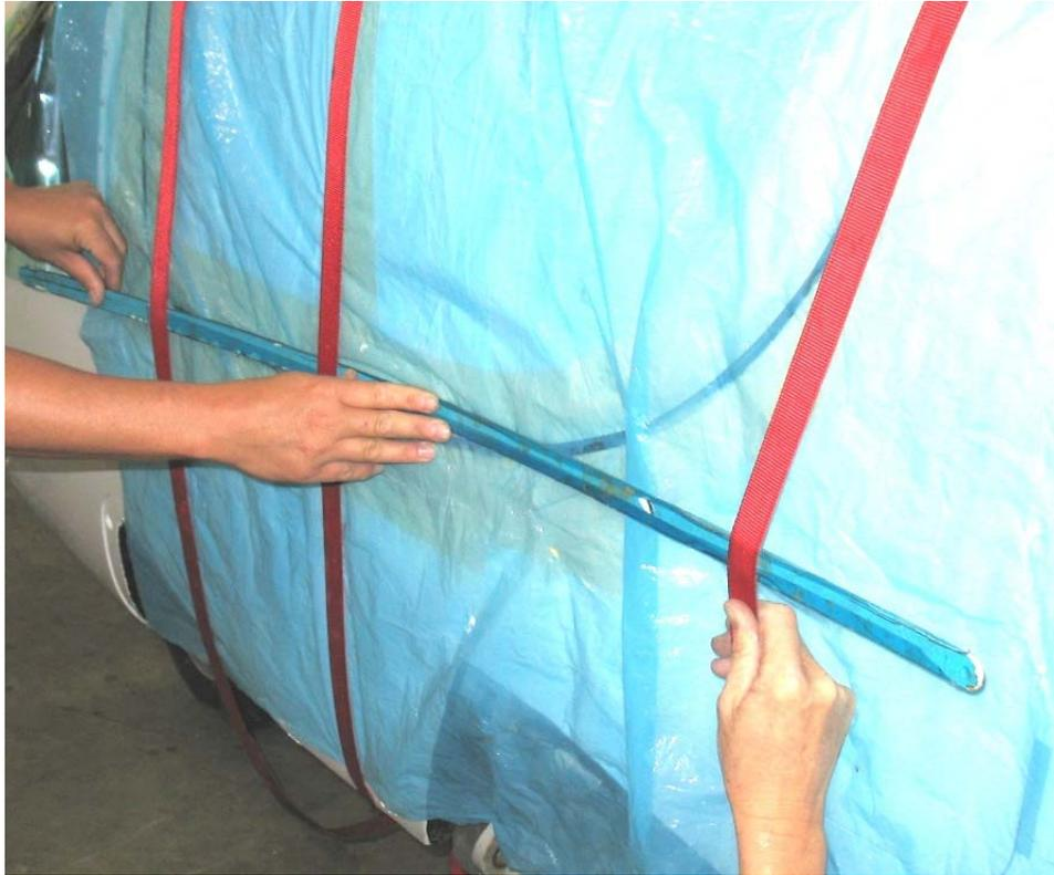
**Figure 56-10 Place the Metal Bands Under the Cloth Straps Over the Horizontal Lower Seam of the Doorframe and the Windscreen**
