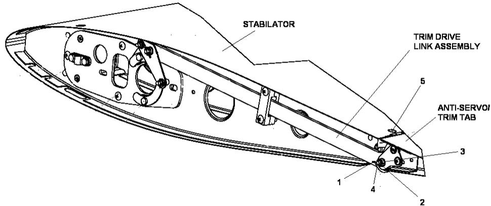
**Figure 27-53 Stabilator and Anti-servo/Trim Tab**
