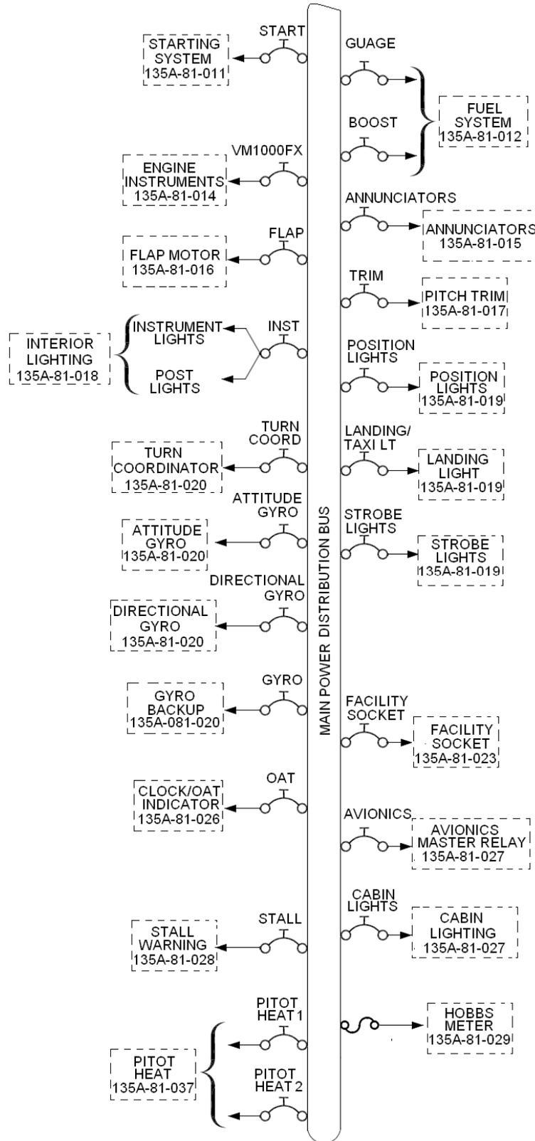
Figure 91-4 Drawing Hierarchy of the Main Power Distribution Bus
