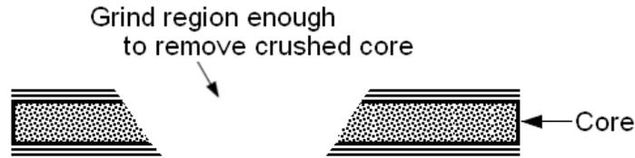
**Figure 51-17 Damaged Area after Grinding**
