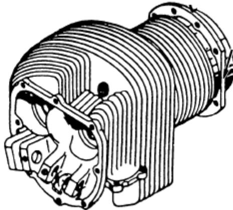
Figure 72-4 Cylinder Head Assembly
