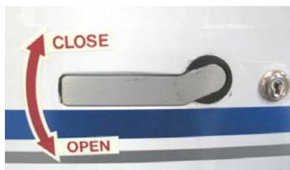
**Figure 52-2 Location of the Exterior Door Handle (Port Side Shown)**
