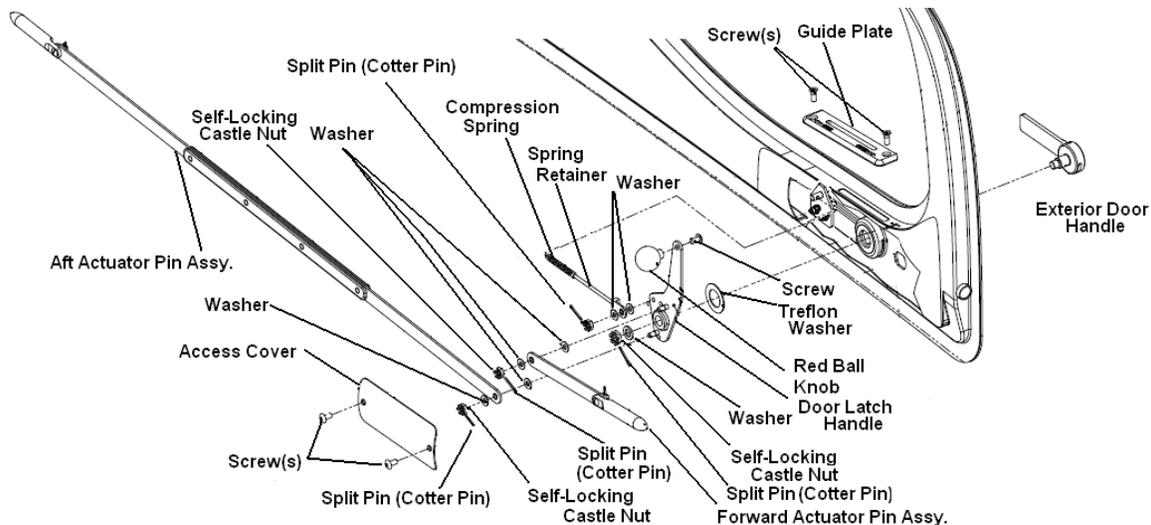
Figure 52-8 Door Latch Assembly (Port Side)
