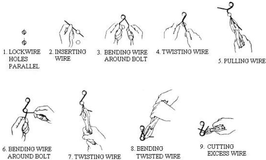
**Figure 20-3 Illustration of the Procedure to Use Lockwire**
