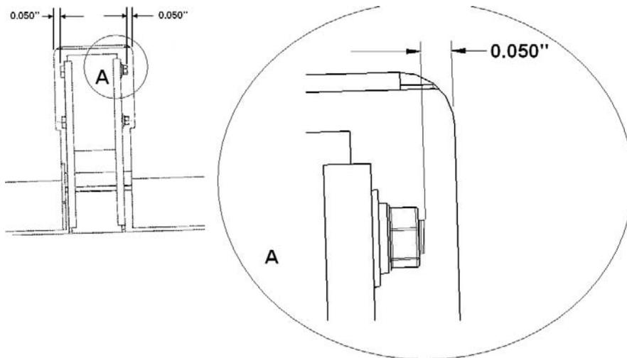
**Figure 27-7 Clearance Between Balance Weight and Wing**
