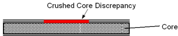
**Figure 51-4 Original View of the Damage**
