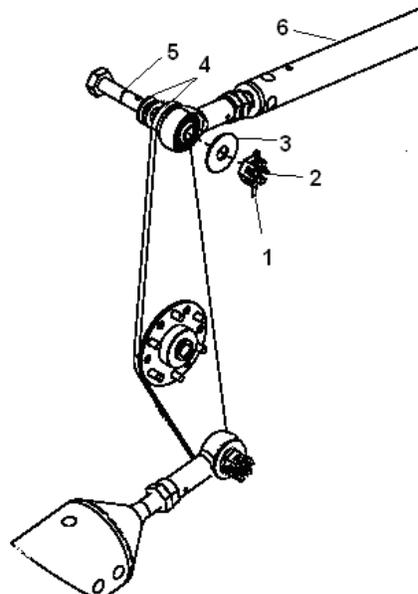
**Figure 27-42 Aft Pushrod to Aft Idler Plate Connection**
