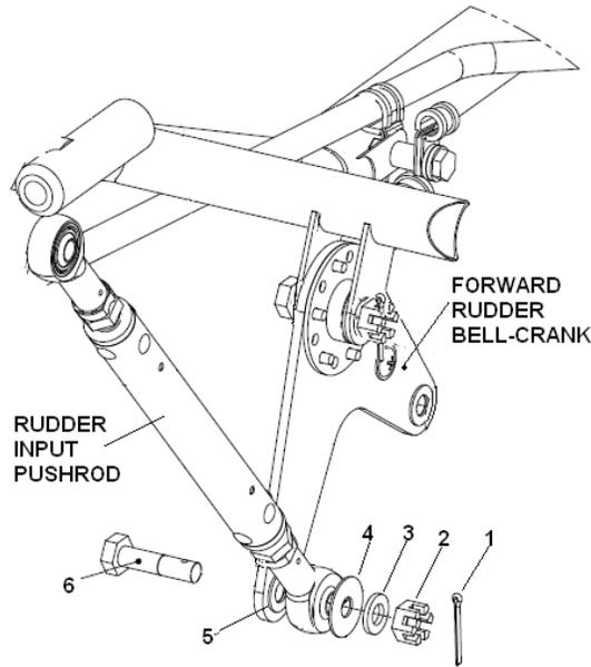
**Figure 27-36 Exploded View of the Input Pushrod to Forward Bell-crank**
