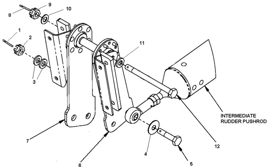
**Figure 27-29 Intermediate Rudder Pushrod and Center Idler-plate**
