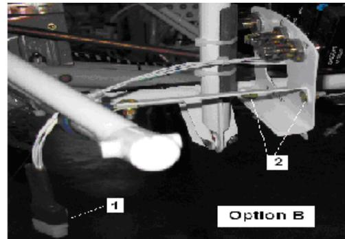
**Figure 27-72 Flap Position Sensor**
