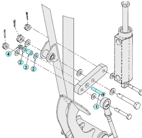
**Figure 32-28 Toe Brake Over-Center Stop Hardware**
