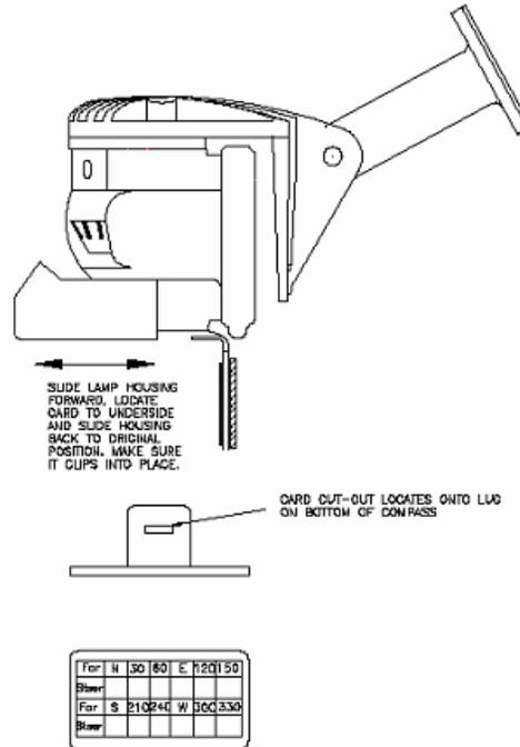
**Figure 34-33 Compass Correction Card Installation**
