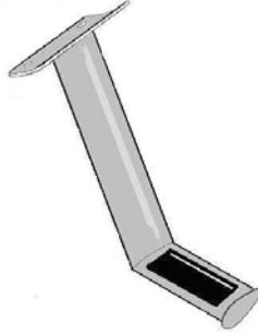
**Figure 11-32 Location of the anti-skid strip tape on the foot step**
