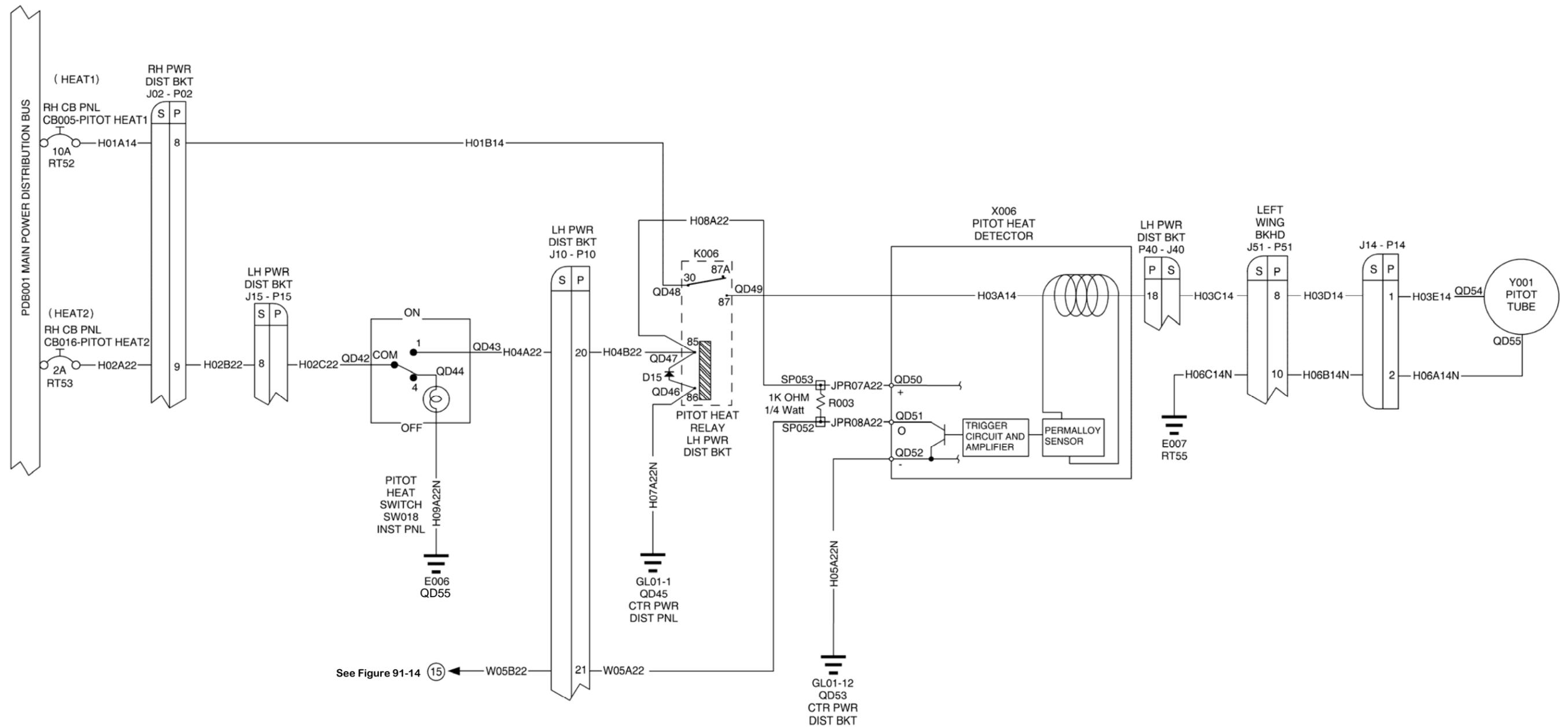
Figure 91-38 Pitot Heating System
