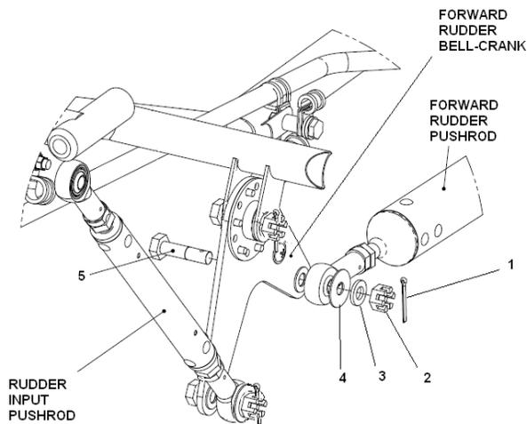
**Figure 27-37 Forward Rudder Bell-crank to Forward Rudder Pushrod Connection**
