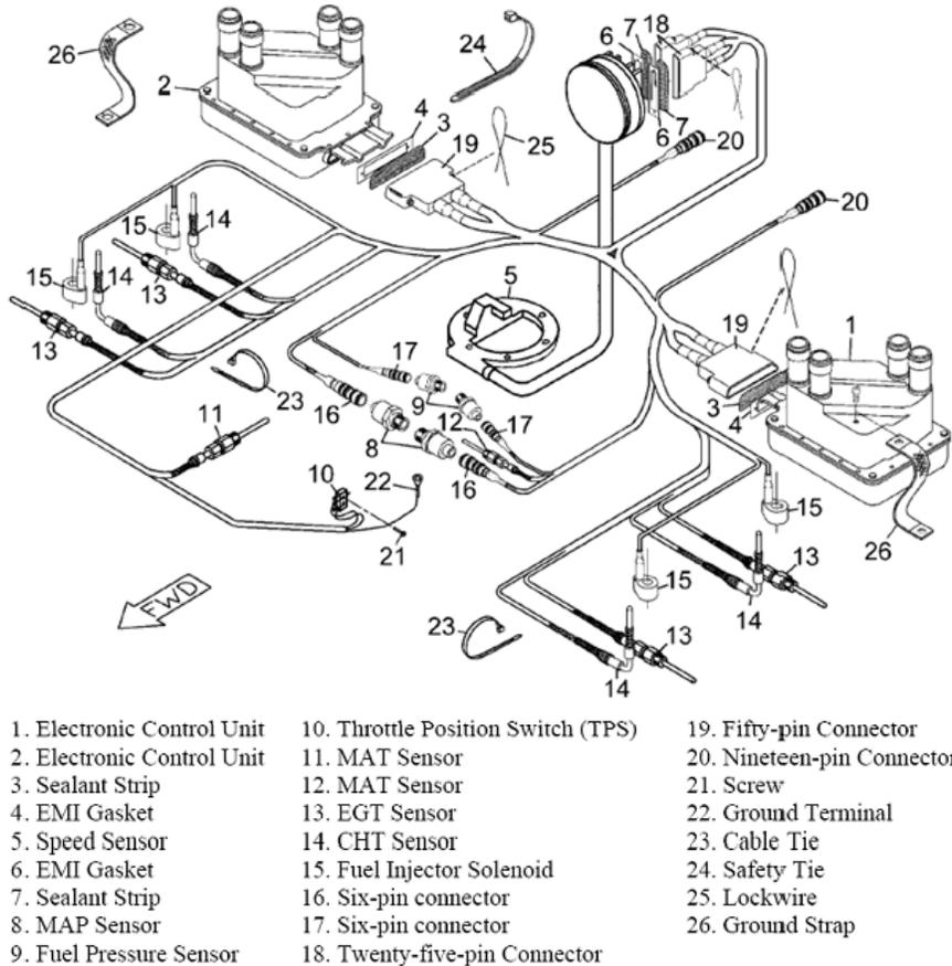
**Figure 71-40 Low Voltage Harness on IOF-240-B Series Engine**
