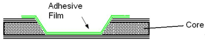
**Figure 51-6 Application of the Adhesive Film**
