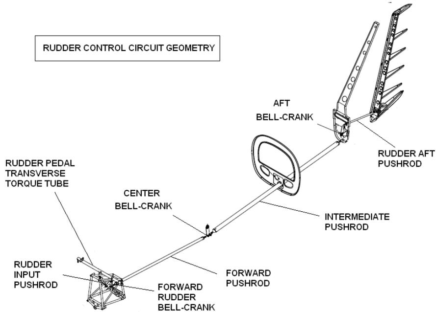
Figure 27-22 Rudder Control Circuit Geometry
