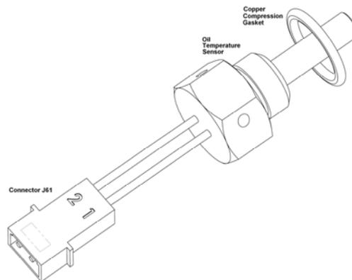
**Figure 79-12 Oil Temperature Sensor Showing the Copper Compression Gasket**
