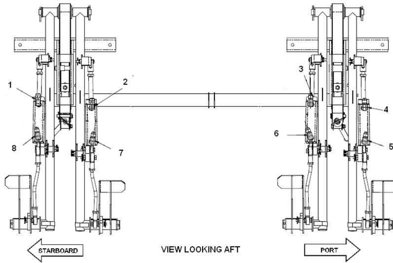
**Figure 27-41 Brake Pedal Assembly Hydraulic Line Fittings**
