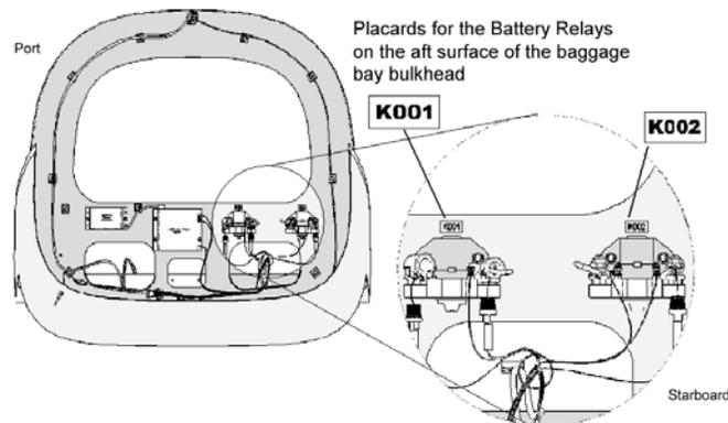
Figure 11-16 Aft side of the Baggage Bay Bulkhead showing the location and details of the relay placards
