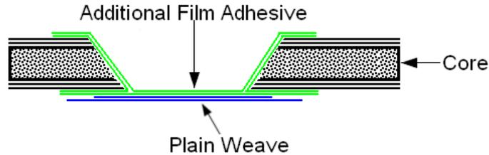
**Figure 51-20 Application of Additional Layers of Adhesive Film**
