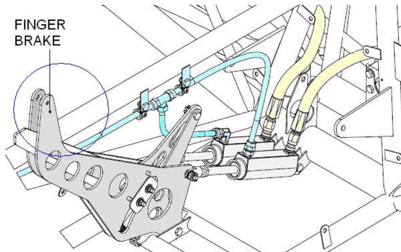
**Figure 32-31 Finger Brake Location**
