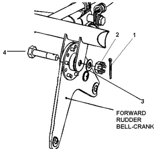
**Figure 27-35 Forward Rudder Bell-crank**
