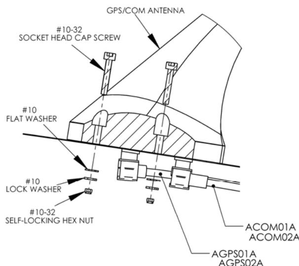
**Figure 23-10 CI 2480-200 COM/GPS Antenna Installation details**
