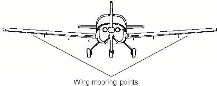
**Figure 10-1 Mooring Points on the Wings**
