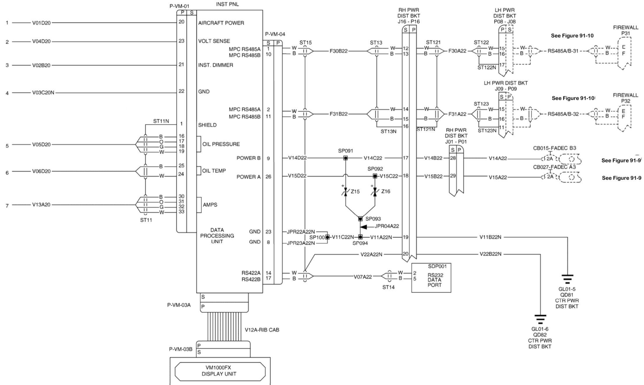
Figure 91-13 VM1000FX Engine Instrument System (2 of 2)
