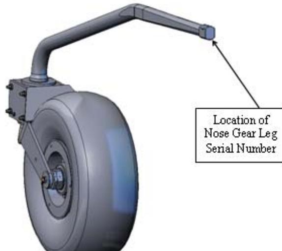
**Figure 32-41 Location of Nose Gear Leg Serial number**
