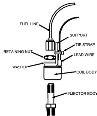
Figure 73-5 Fuel Injector Assembly
