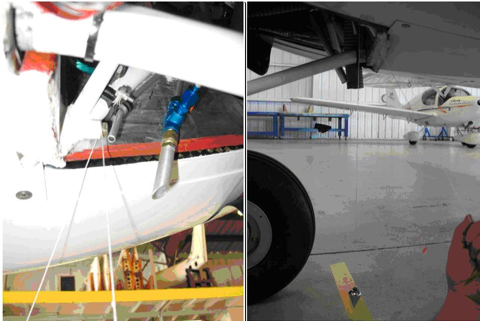
**Figure 08-1 Plumb Bob Dropped at Reference Location (STA 48.1)**
