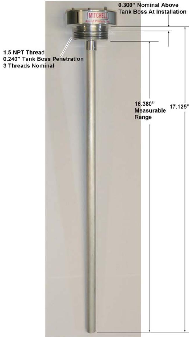
Figure 28-20 Capacitive Fuel Sender
