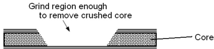
**Figure 51-10 Section of Composite After the Grinding**
