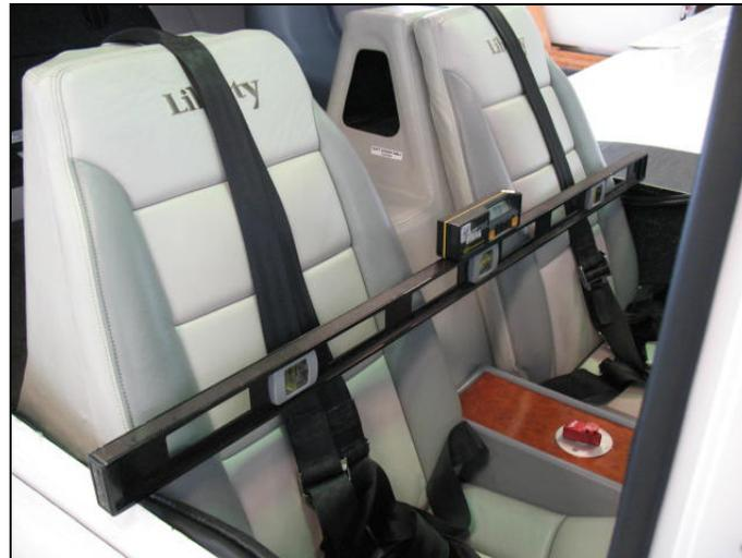
**Figure 08-7 Aircraft Laterally Leveled (Aileron Yoke Blocks Are Not Shown)**
