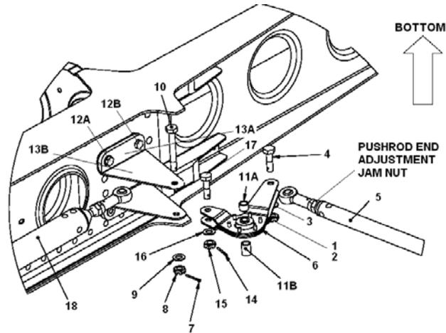
**Figure 27-10 Aileron Wing Bell-crank Assembly**
