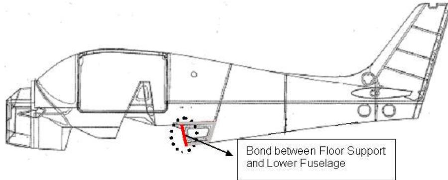
**Figure 53-3 Inspection Location Between The Bonded Sections Of The Baggage Bay Floor**
