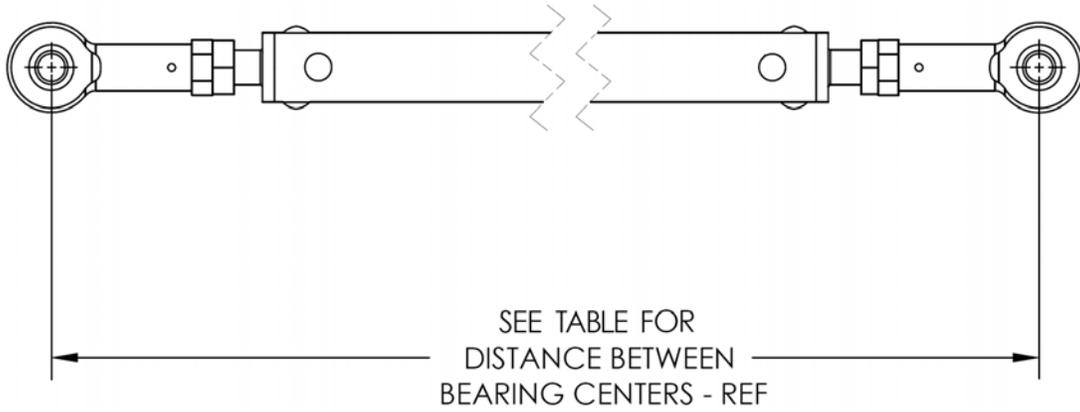
**Figure 27-1 Torque Tube Distance**
