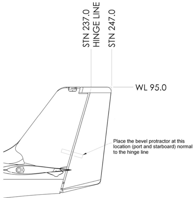
**Figure 27-93 Rudder Measurements**
