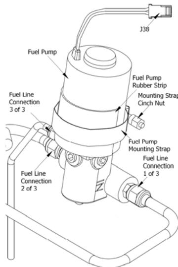
**Figure 28-11 Fuel Pump Mounting**
