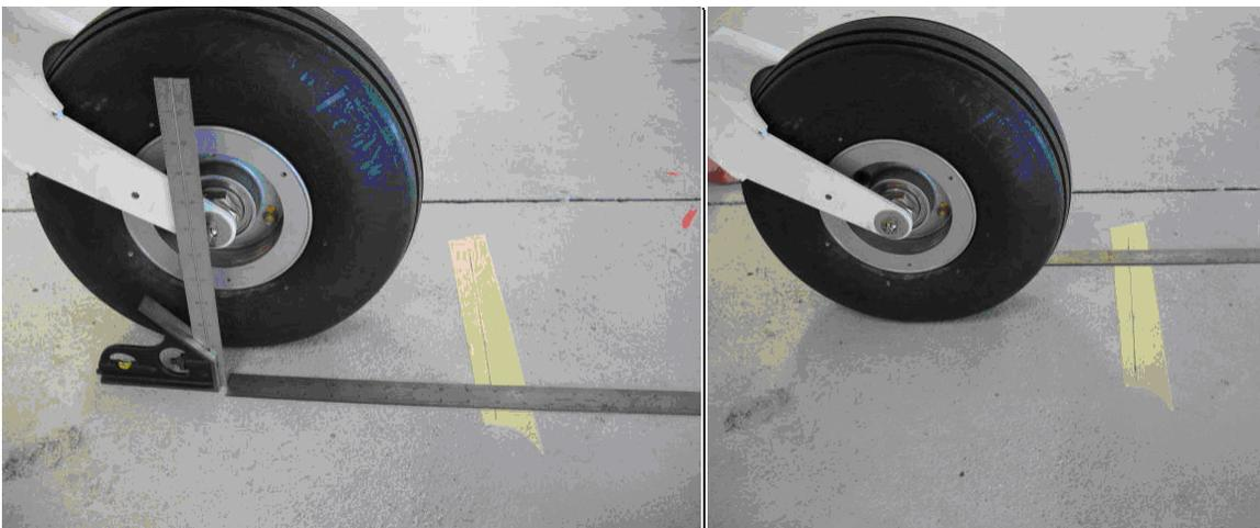
**Figure 08-2 Measurement of Distance Between STA 48.1 and Both Sides of Nose Gear Axle**
