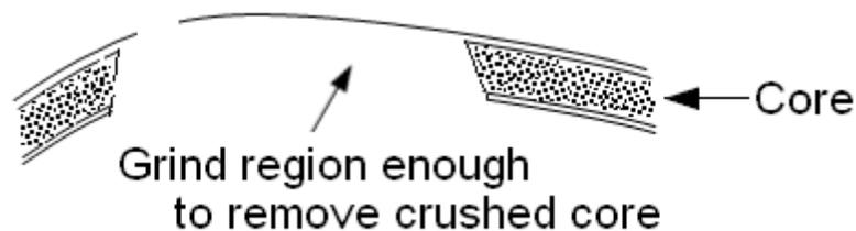
**Figure 51-25 Same Region After Grinding to Remove the Damaged Core**
