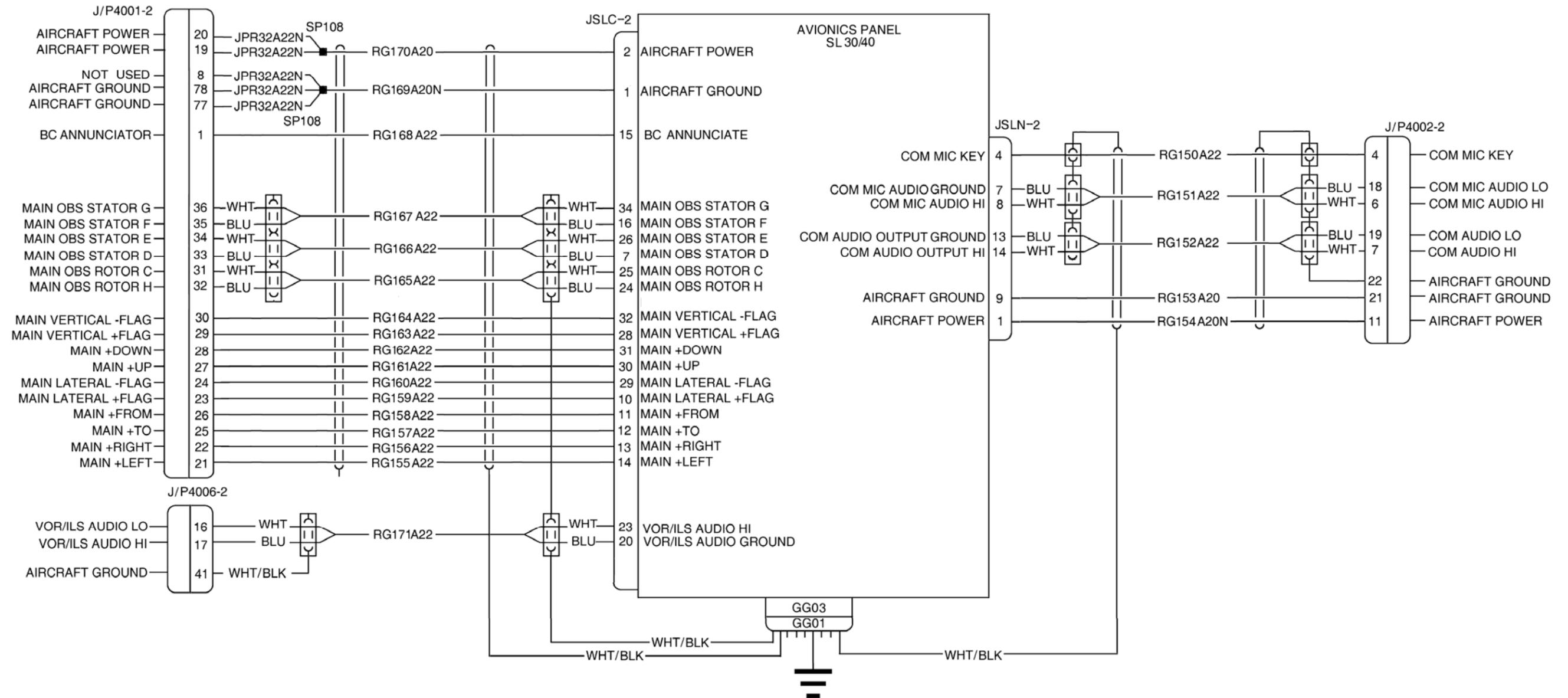
Figure 91-35 Avionics (GNS to SL Adapter)
