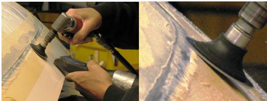
**Figure 56-14 Grinding the Cured Epi-Bond on the Outside Surface of the Doorframe and Windscreen**
