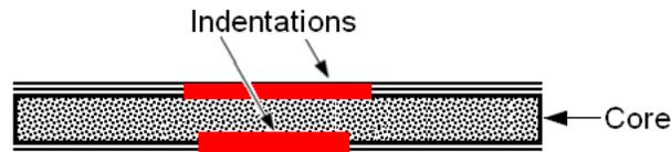
**Figure 51-16 Cross Section of Damaged Area**
