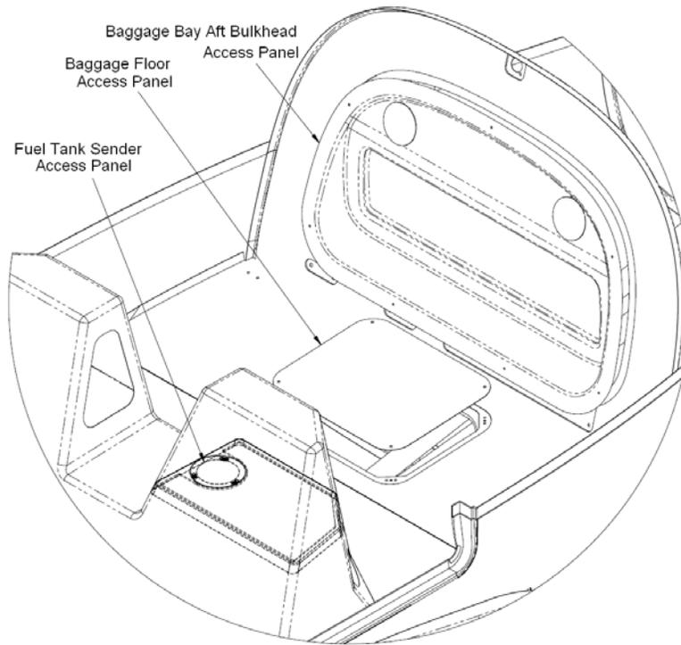
Figure 03-8 Interior Access Panels Aft of the Cockpit
