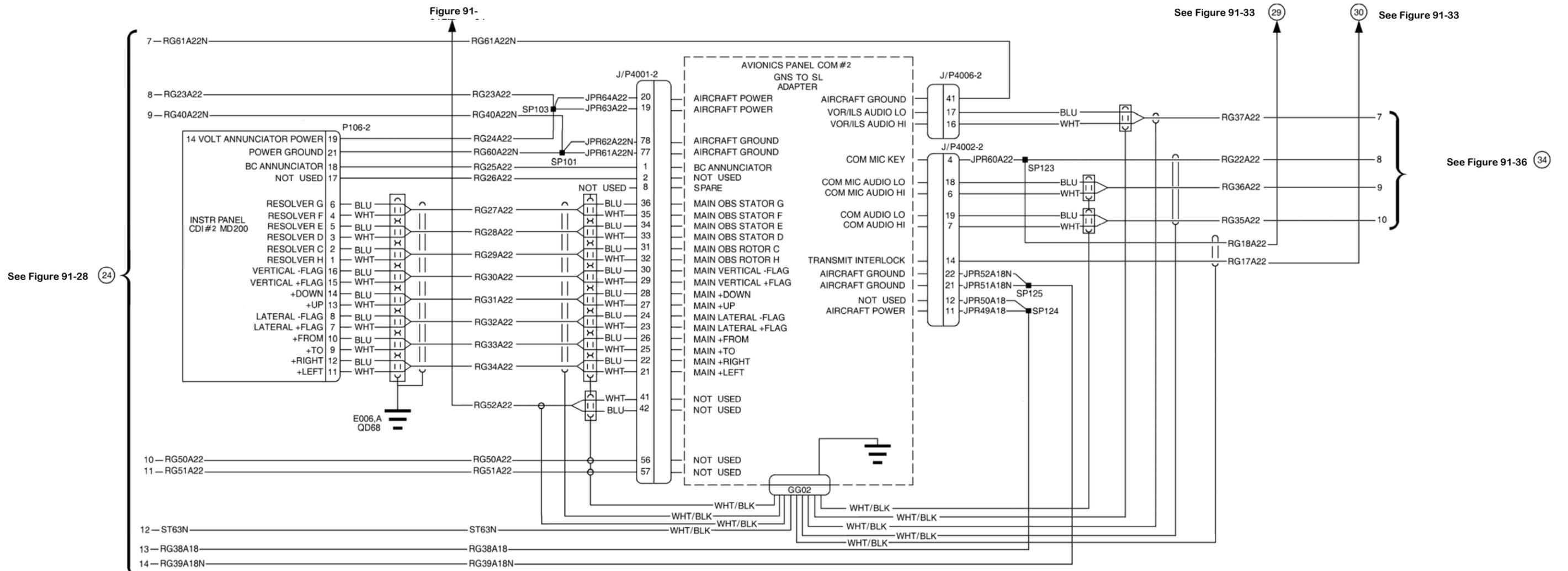
Figure 91-34 Avionics (Dual SL System) 2 of 2
