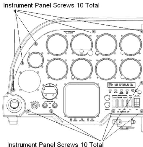
**Figure 77-5 Location of the Screws Securing the Instrument Panel**
