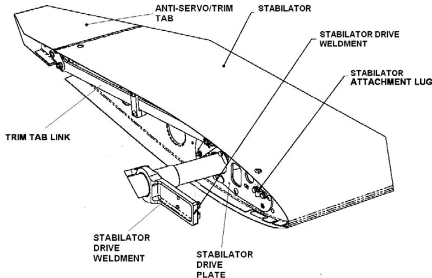
**Figure 55-1 Stabilizer Drive Components**
