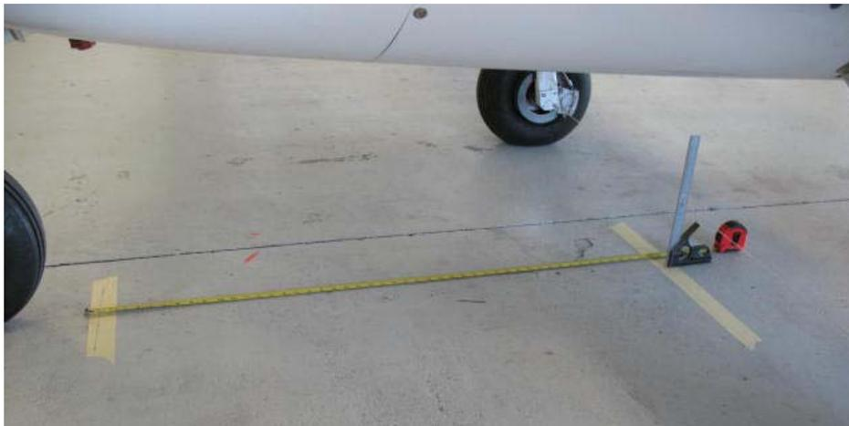
**Figure 08-3 Measurement of Distance Between STA 48.1 and Main Gear Axles**
