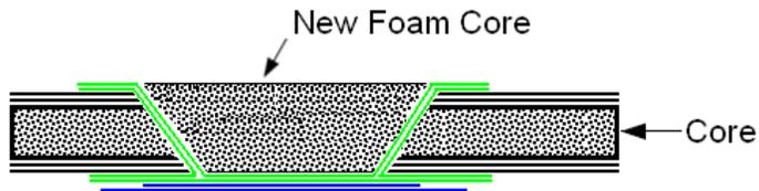
**Figure 51-21 Insertion of the New Core**
