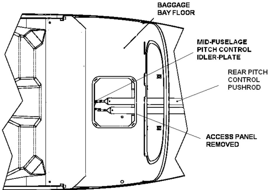
**Figure 27-49 Mid-fuselage Pitch Control Idler-plate Location**
