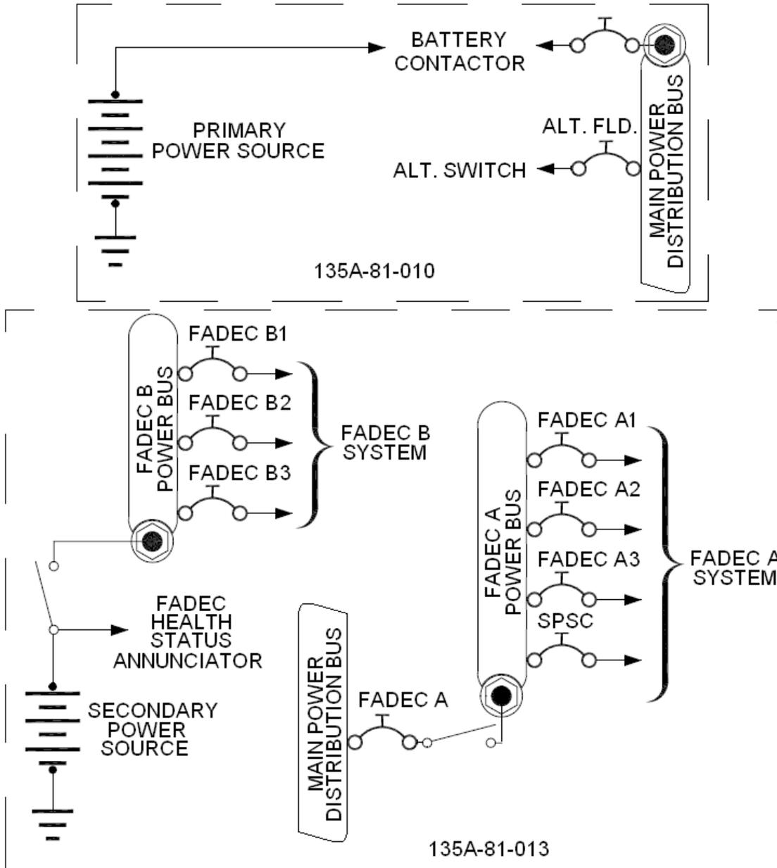
**Figure 91-3 Drawings For the Two Battery Systems**
