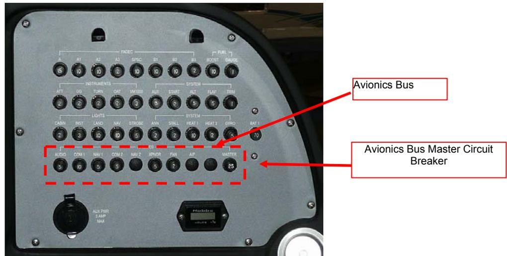
**Figure 24-20 Circuit Breaker Panel – Avionics Bus**
