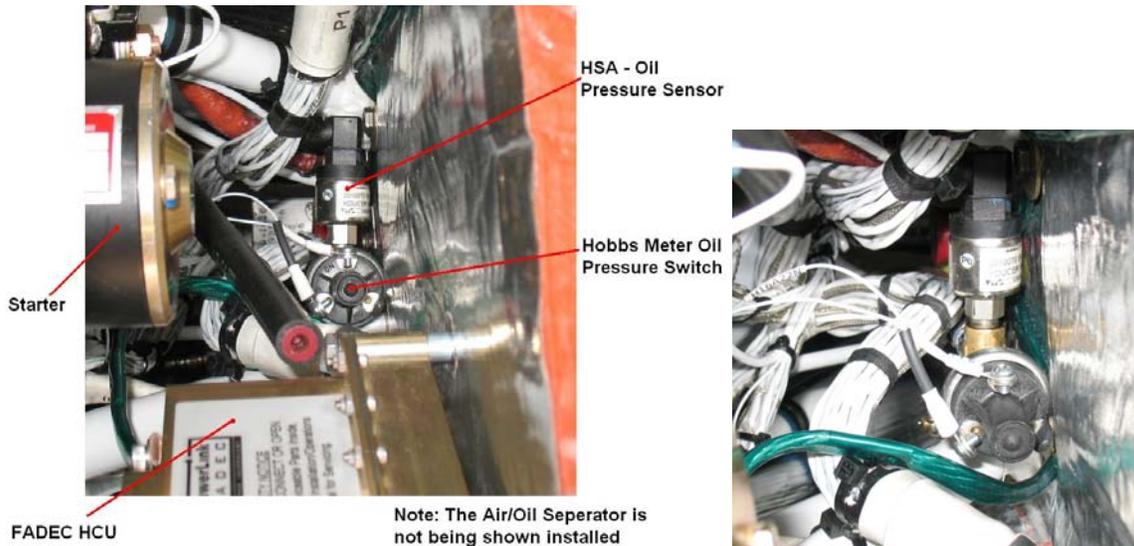
**Figure 79-8 Location of the Oil Pressure Switch (Hobbs) and the Oil Pressure Sensor (HSA) (The Air/Oil Separator Not Shown)**
