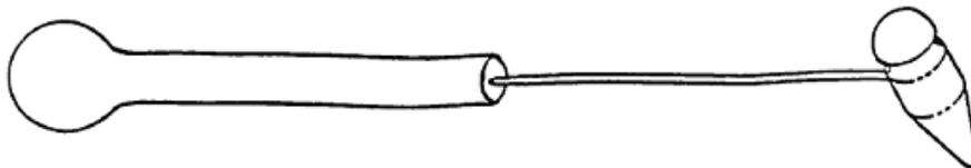
**Figure 51-3 Sample Of Special Tap Test Hammer For Tap Testing**
