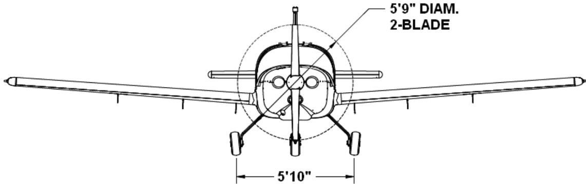
**Figure 06-1 (Reference Only) Front View of Airplane Dimensions \***
