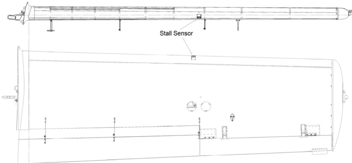
**Figure 31-25 Stall Sensor Location**
