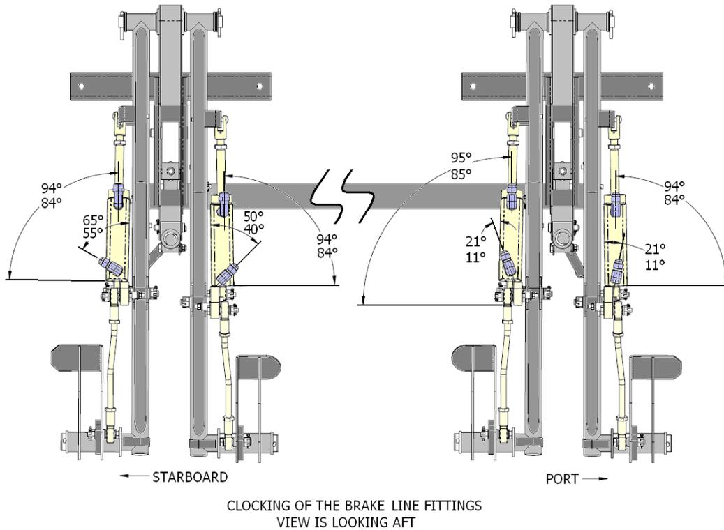
**Figure 32-25 Clocking of the Brake Line Fittings**
