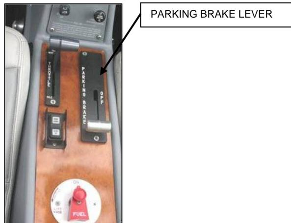
**Figure 32-21 Toe Brake System Parking Brake Lever**
