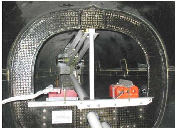
**Figure 53-24 AFT Bulkhead Mid Fuselage**
