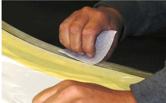
**Figure 56-5 Sanding the Edge of the Door Windscreen to Prep for the Adhesive**
