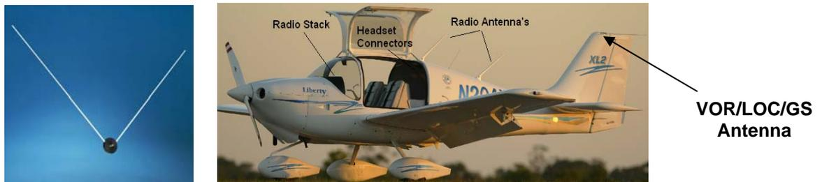
**Figure 34-43 VOR/Glideslope Antenna Installation**
