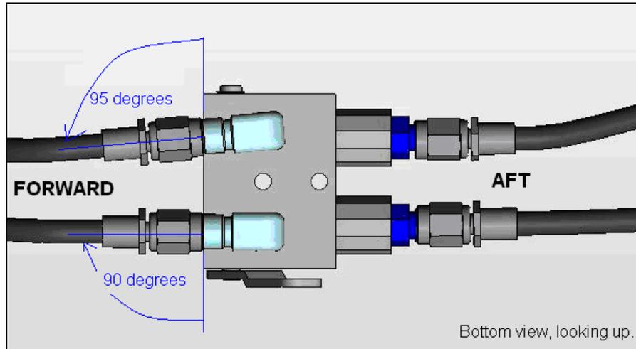
Figure 32-29 Clocking of Parking Brake Valve Fittings (Earlier Brake Valve ONLY)
