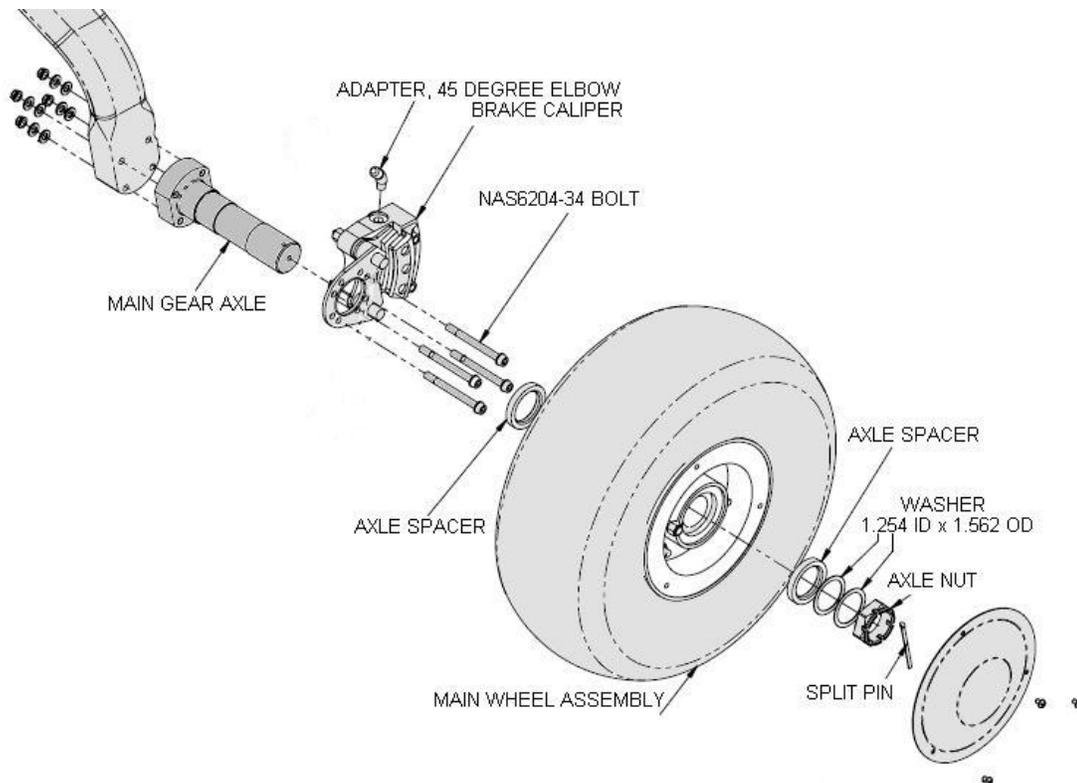
**Figure 32-4 Main undercarriage Assembly**
