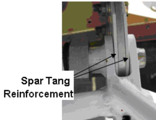
Figure 57-4 Tang Reinforcements Installed
