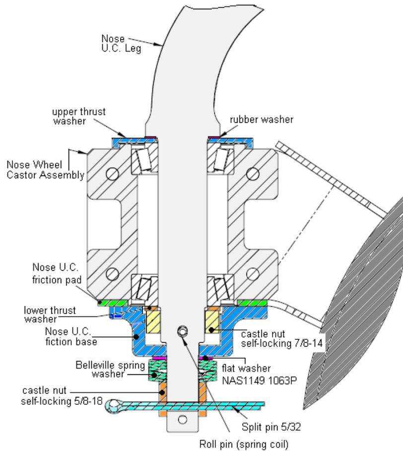
**Figure 32-42 Nose Wheel Steering Assembly**
