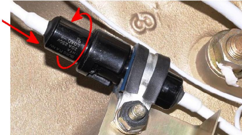
**Figure 24-7 Fuse Holder F3 Disassembly**
