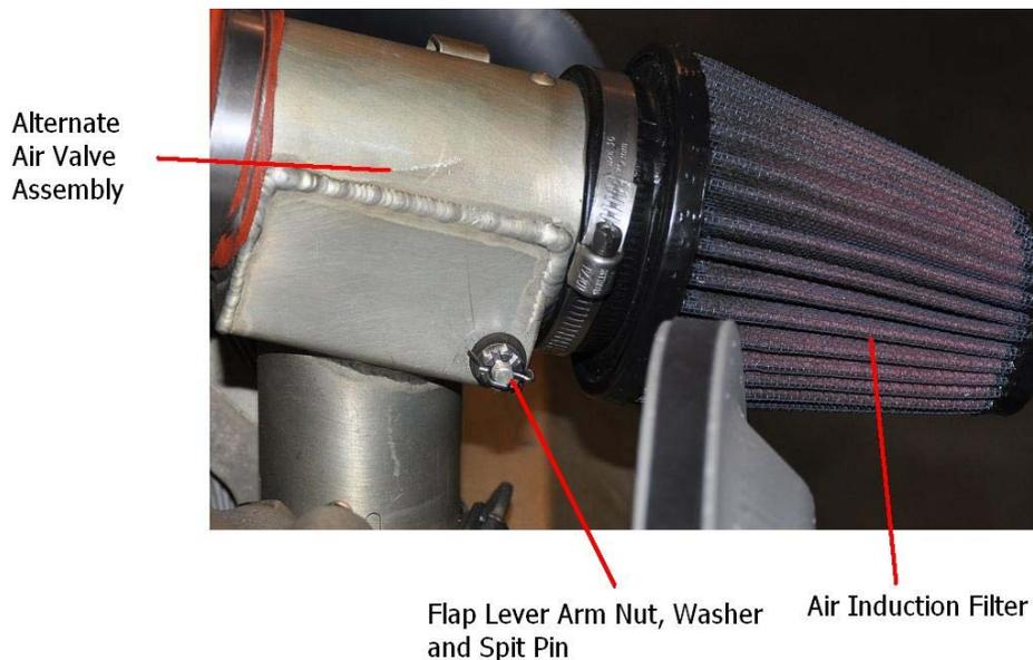
**Figure 71-50 Alternate Air Valve Assembly**
