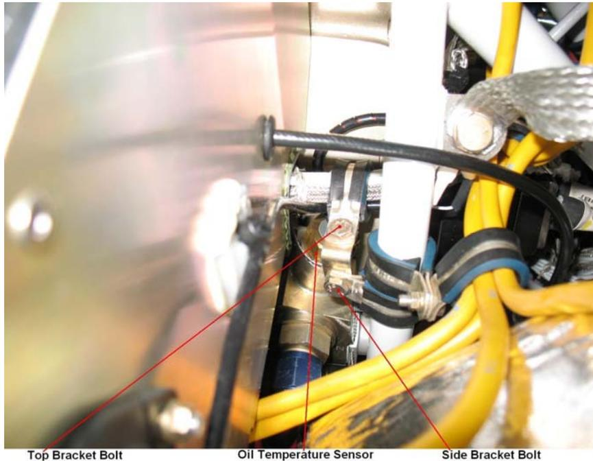
**Figure 77-15 Location of the Oil Temperature Sensor**
