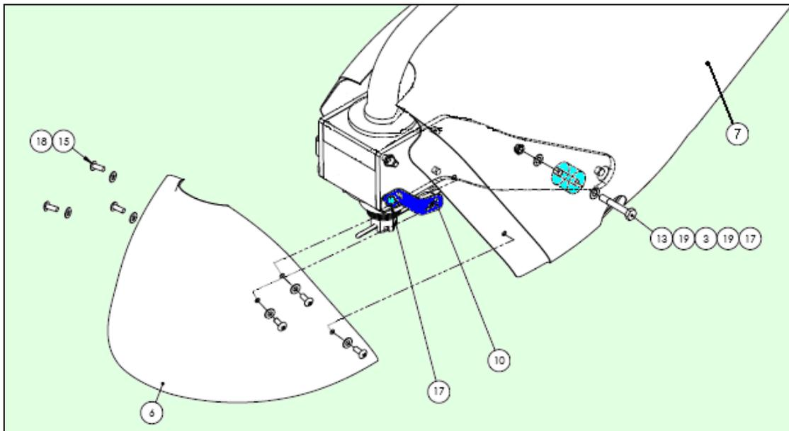
**Figure 32-8 Exploded View of Nose Wheel Fairing**
