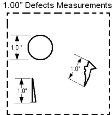
Figure 51-1 Laminate Defect Size Definition Examples
