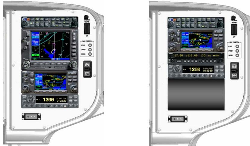
**Figure 23-1 Typical Radio Installation on the left, is the GNS530/430 typical installation, on the right, is the GNS 430W/SL30 typical installation**
