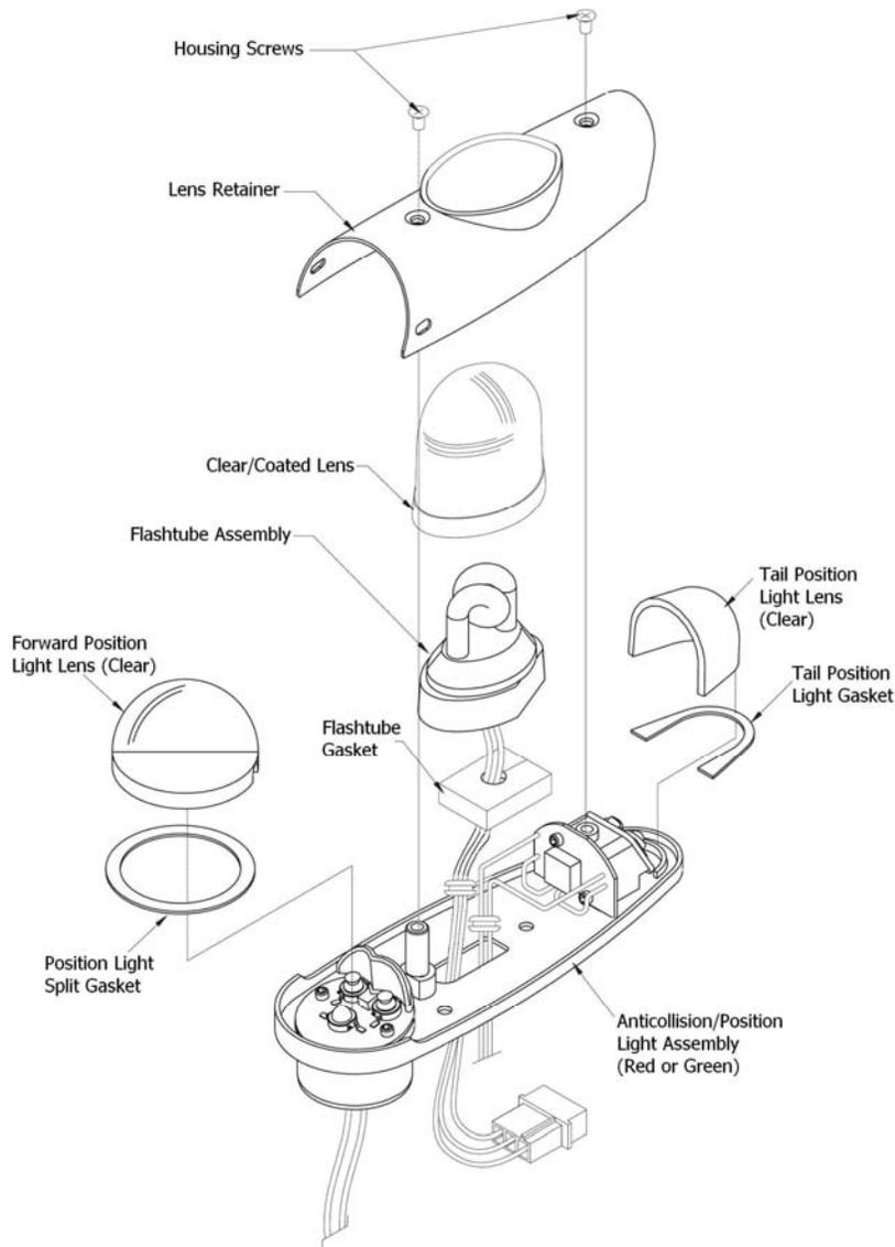
**Figure 33-11 Anti-collision light installation**
