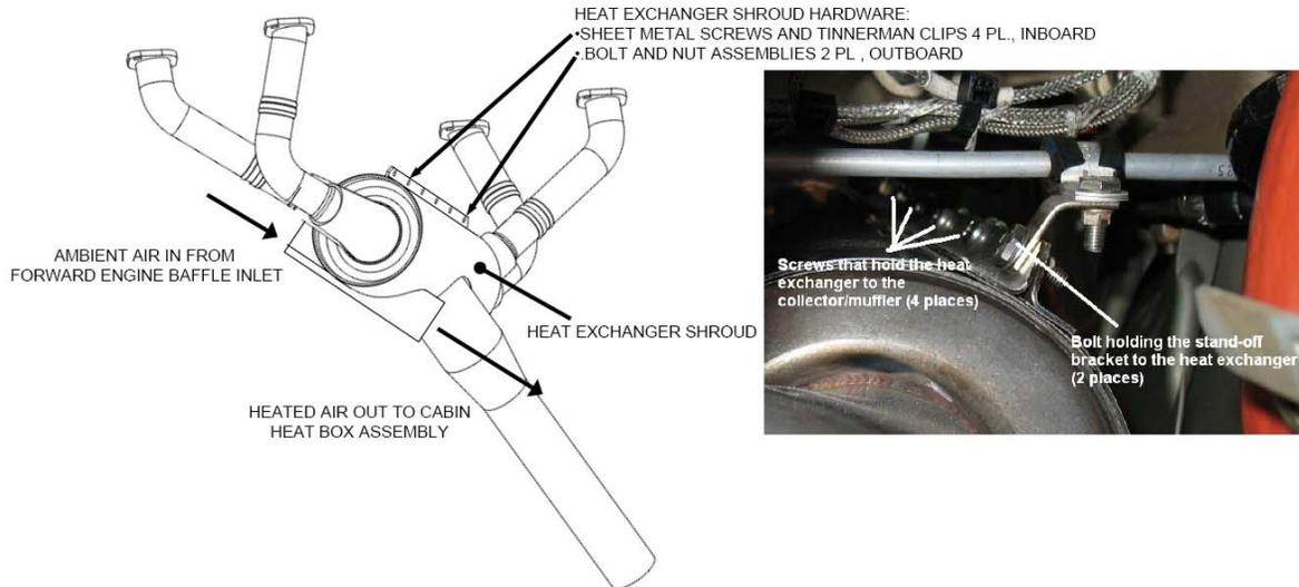
**Figure 21-5 Heat Exchanger Hardware**
