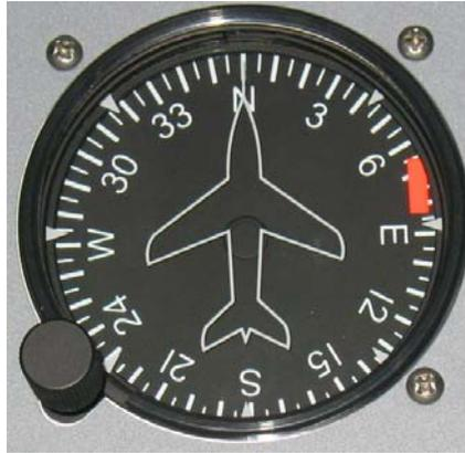
**Figure 34-36 Directional Gyro Indicator**
