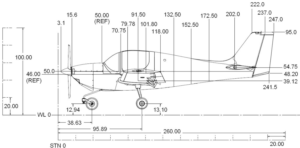
**Figure 03-4 Measurements from the Waterline and Station**
