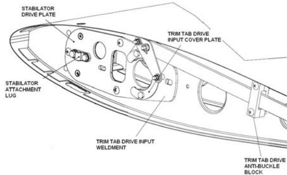
**Figure 55-3 Stabilator Drive Plate**
