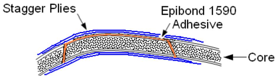
**Figure 51-27 Finished Repair Showing the Layers of Plain Weave**
