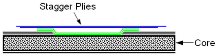
**Figure 51-31 Application of the Staggered Layers of Plain Weave**
