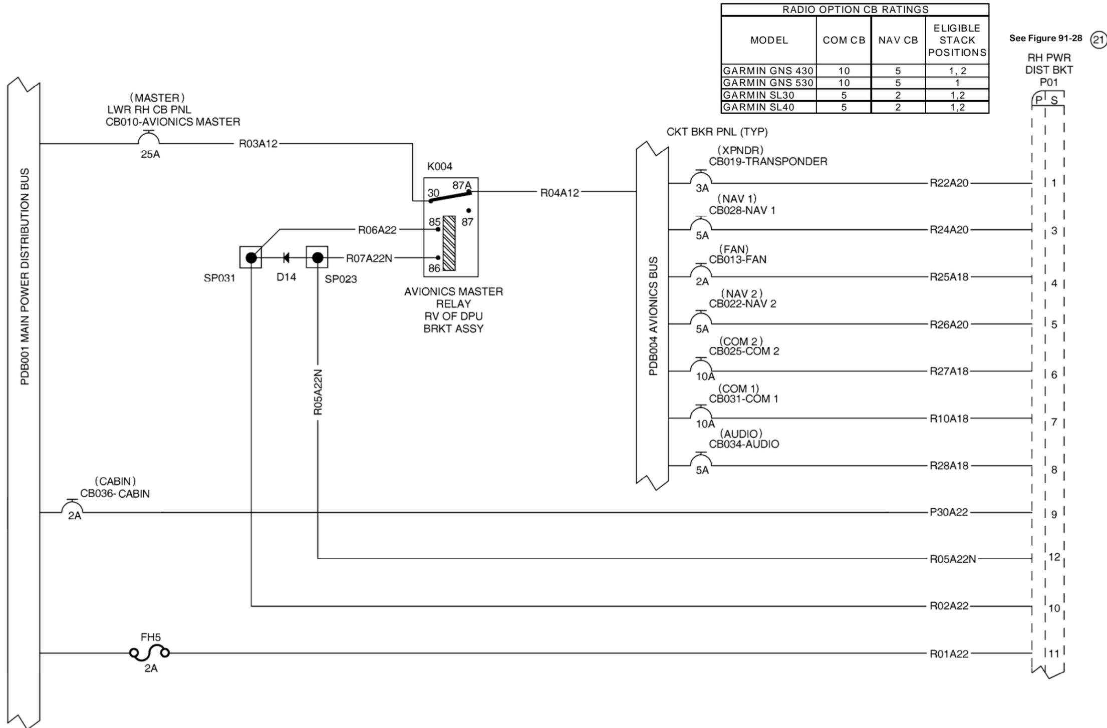
Figure 91-24 Avionics Power Distribution System
