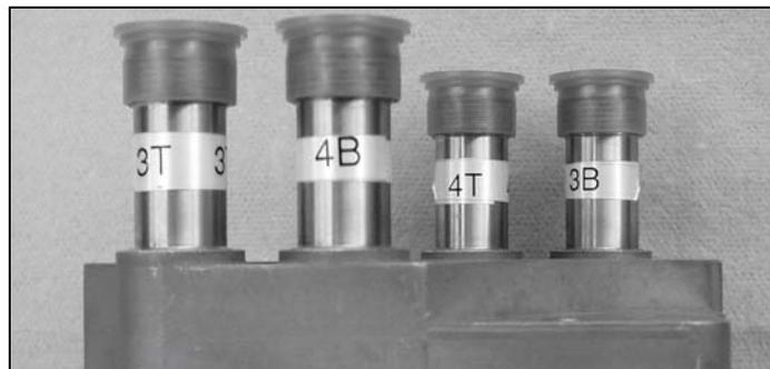
**Figure 71-43 Ignition Lead Wire Connections to ECUs**
