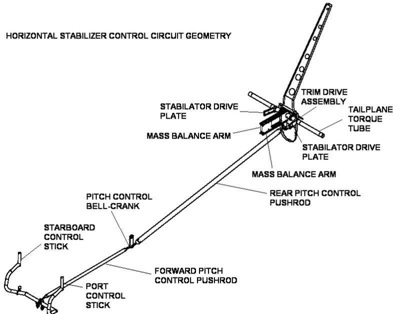
**Figure 27-46 Horizontal Stabilizer Control Circuit Geometry**
