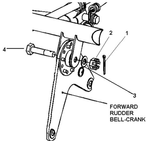
**Figure 27-34 Forward Rudder Bell-crank**
