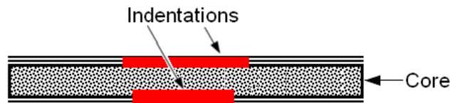
**Figure 51-12 Cross Section of Damaged Composite Sandwich**
