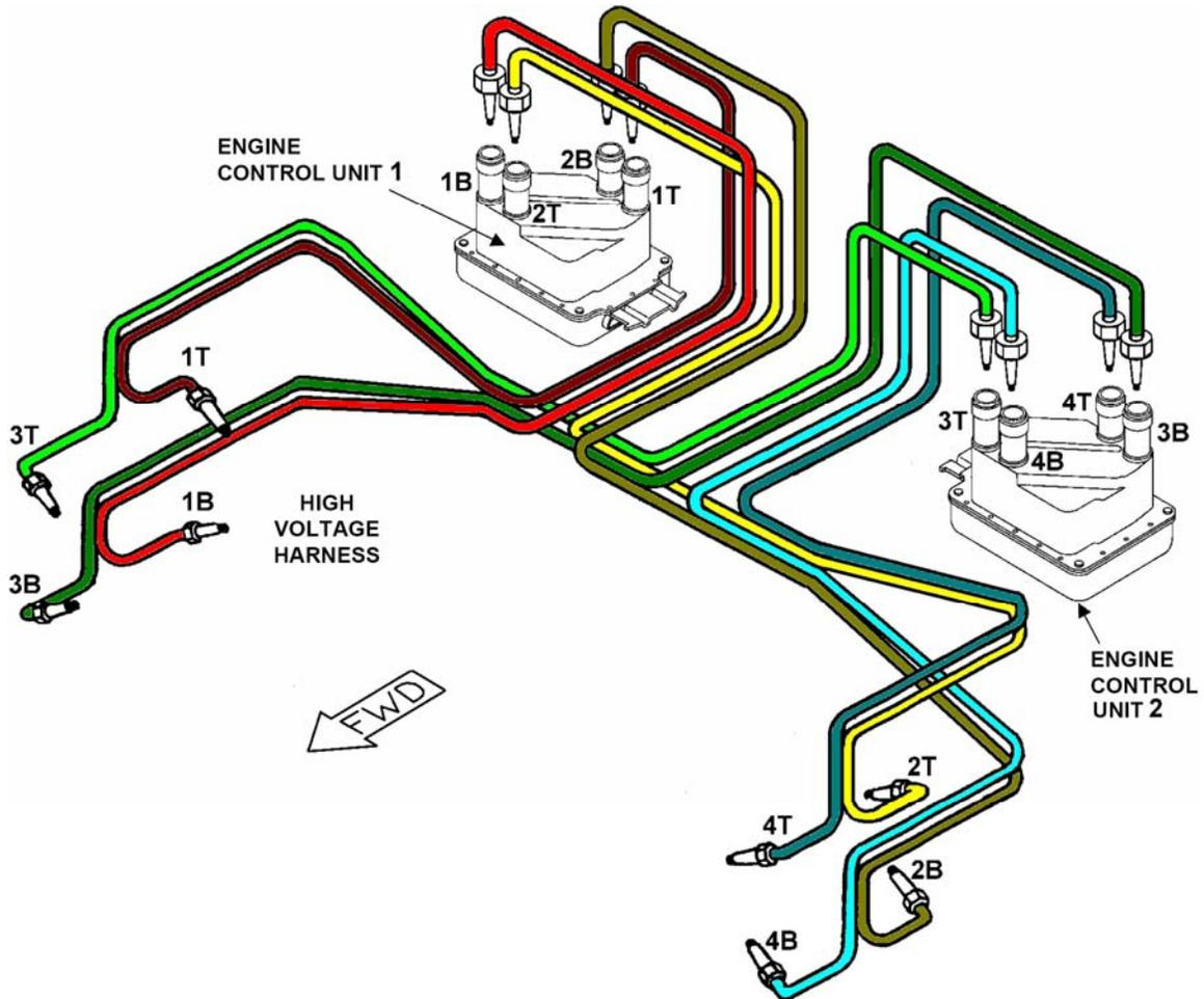
Figure 71-41 FADEC Ignition System Harness
