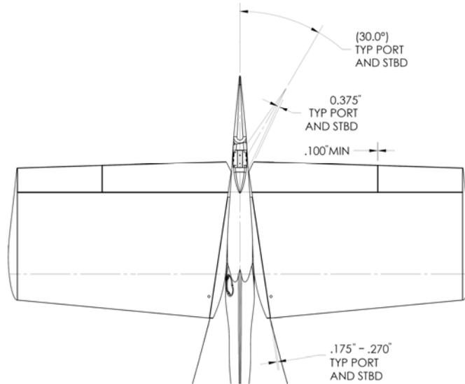
**Figure 27-80 Tail Section Measurements**
