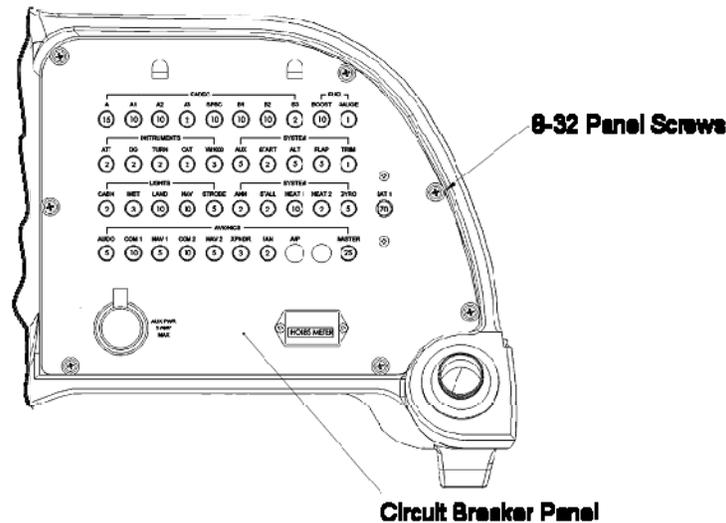
Figure 24-22 Circuit Breaker Panel
