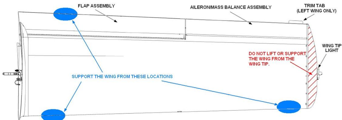
**Figure 57-5 Wing Handling Positions**
