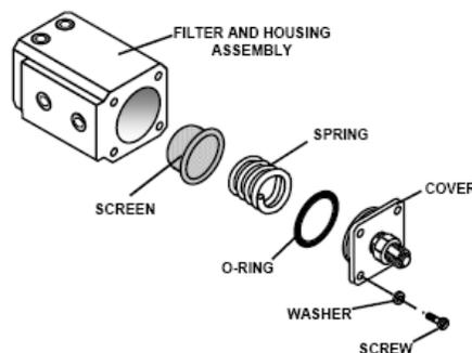
**Figure 73-3 Bypass Fuel Filter Assembly**
