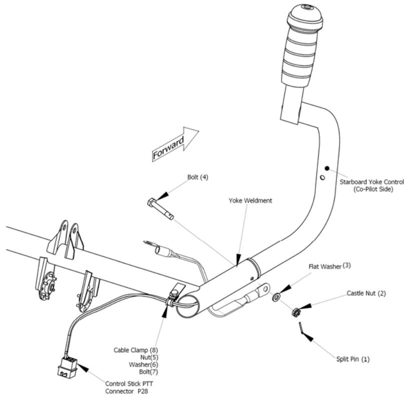
**Figure 27-60 Starboard Control Stick Removal and Installation**
