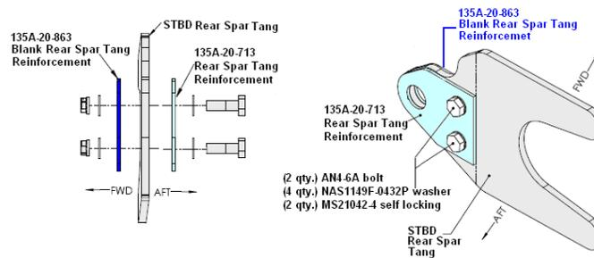
Figure 57-2 Starboard Rear Spar Tang Reinforcement Installation
