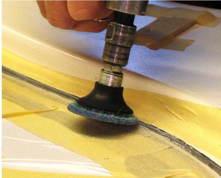
**Figure 56-15 Grinding the Cured Epi-Bond on the Inside Surface of the Doorframe and Windscreen**
