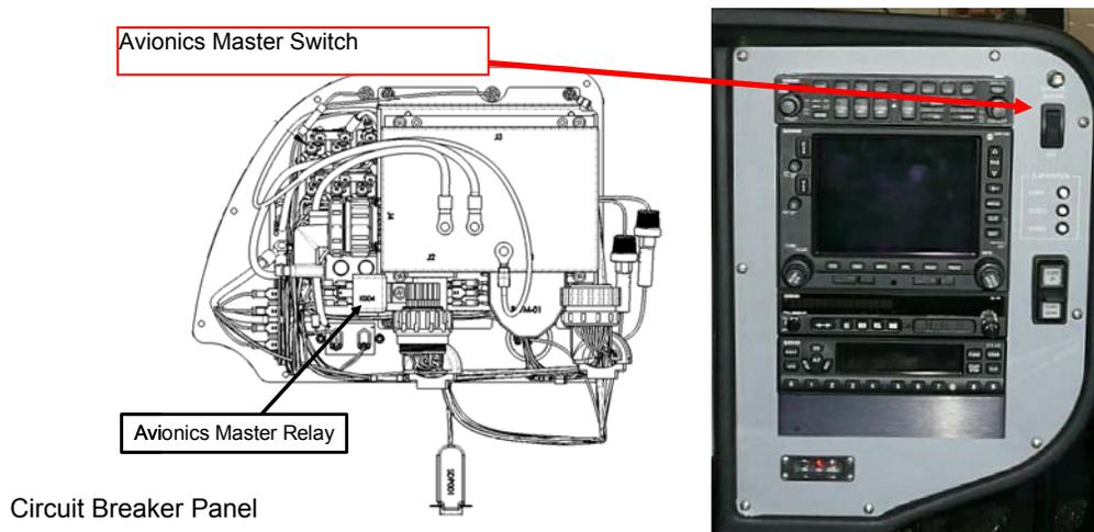
**Figure 24-21 Avionics Panel – Avionics Master Switch**
