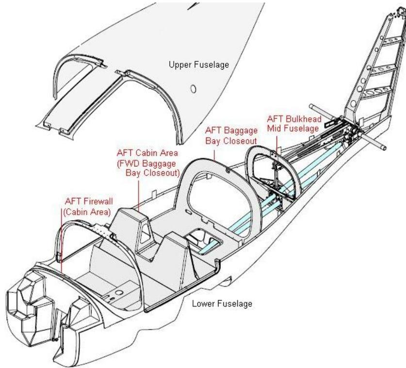
**Figure 53-7 Composite Fuselage Sections**
