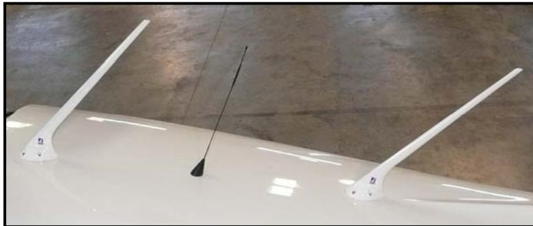
**Figure 25-6 AK450 Antenna Placement**
