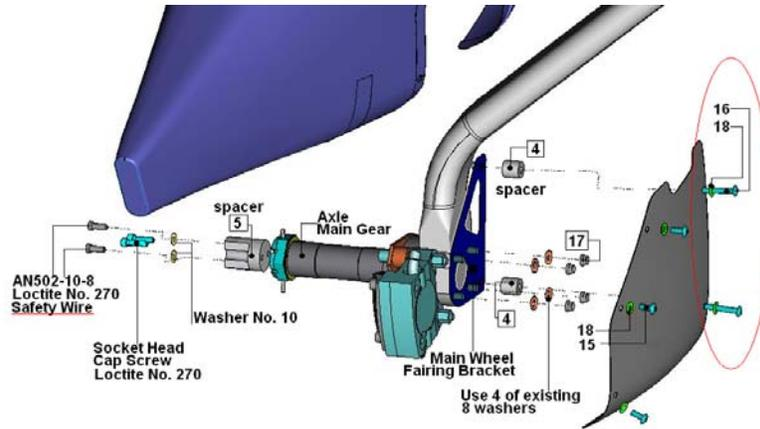
Figure 32-6 Exploded View of Main Wheel Fairing, Port
