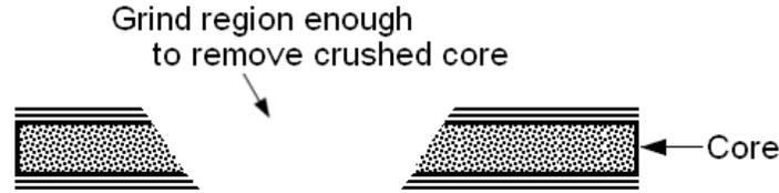
**Figure 51-13 Section of the Composite after Grinding to Remove Damaged Area**
