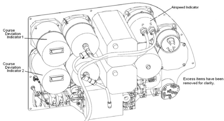
**Figure 34-58 Rear View of the instrument Panel Showing Location of the Course Deviation Indicator(s)**
