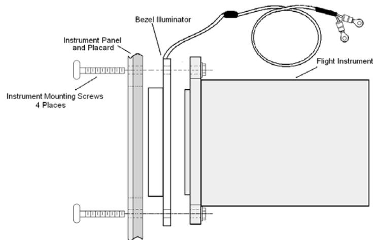
**Figure 33-3 Showing the Assembly of the Bezel Luminary into the Instrument Panel**
