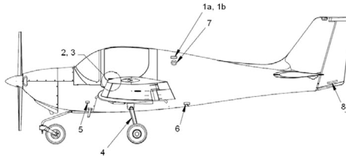
Figure 11-8 Exterior Placards – Port Side of Airplane
