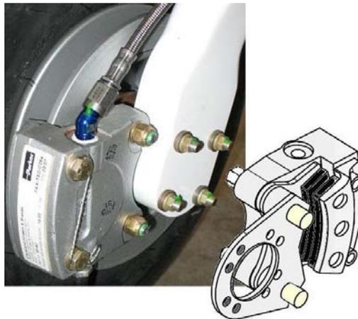
**Figure 32-34 Main Wheel Brake Caliper**
