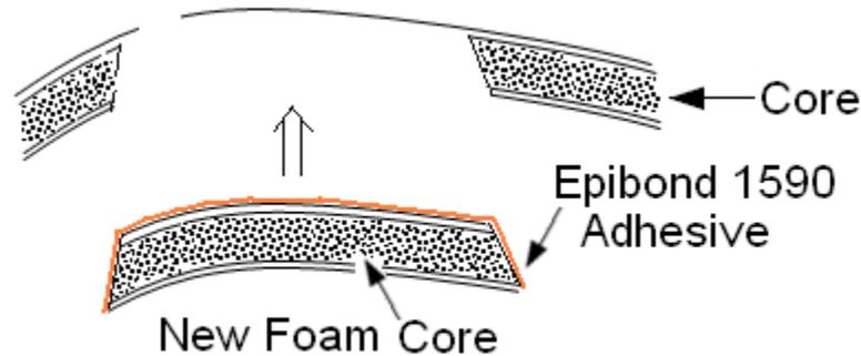
**Figure 51-26 The Core Insert Ready for Insertion into Damaged Area**
