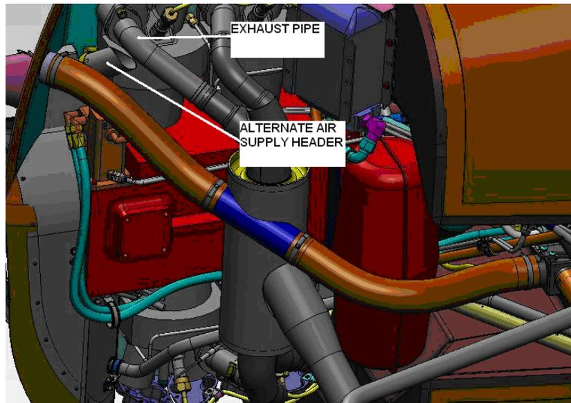
**Figure 78-4 Exhaust Pipe to Alternate Air Supply Header**
