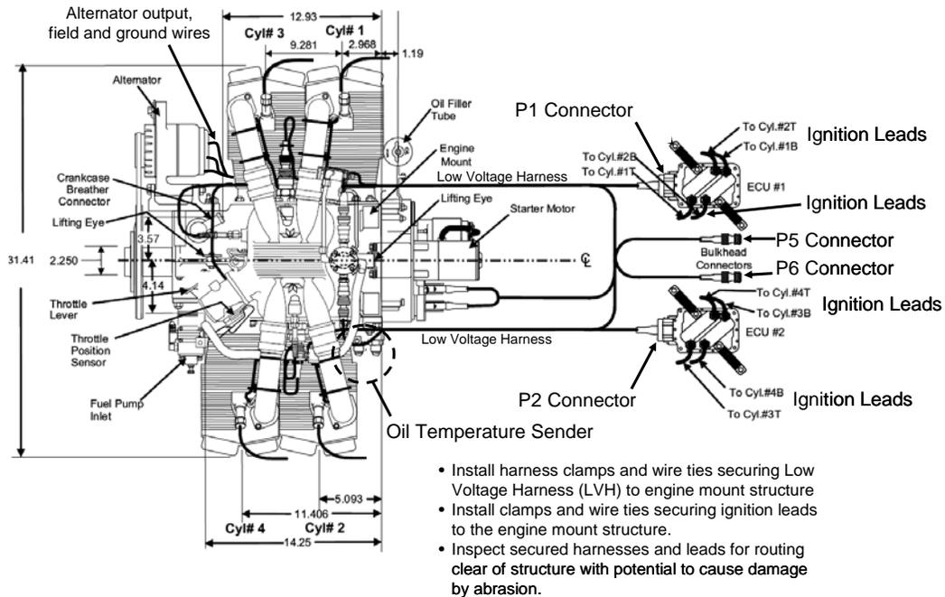
**Figure 71-15 Engine Connections**
