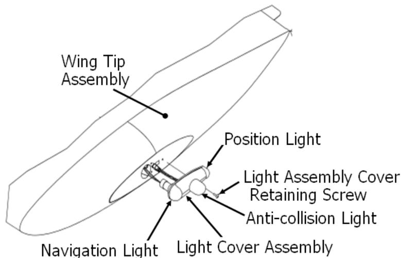
**Figure 33-8 Wing Tip Assembly**
