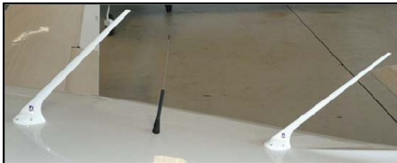
**Figure 25-7 ME406 Antenna Placement**
