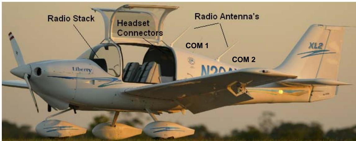
**Figure 23-3 Communications Equipment Placement**
