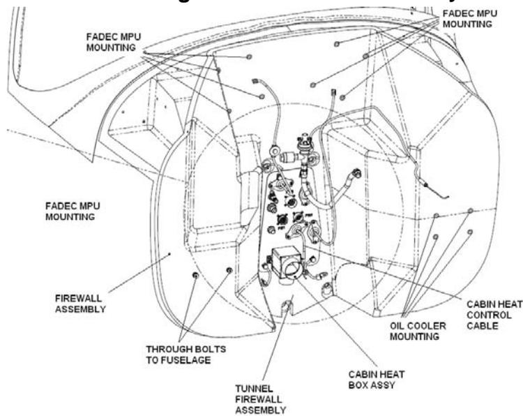
Figure 71-28 Engine Firewall Blanket Installation
