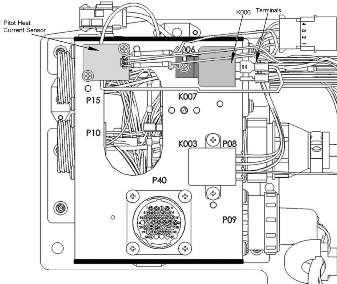
**Figure 30-9 Location of the Pitot Heat Relay K006**
