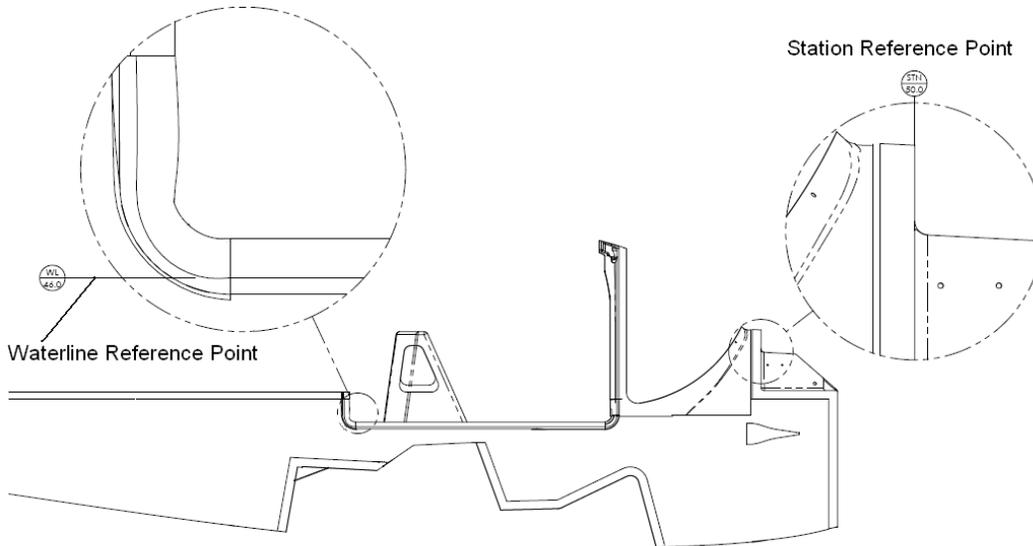
Measurements in Chapter 11 -*Placards and Markings* that would normally reference the Waterline are shown as above or below of the Waterline Reference Point. This point is defined as the lower edge of the lower doorsill (WL46) of the airplane.
