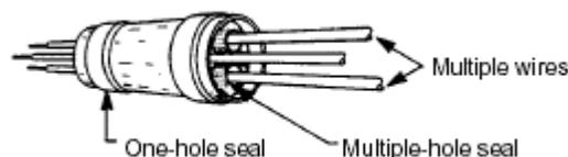
**Figure 20-18 Multiple Wires**
