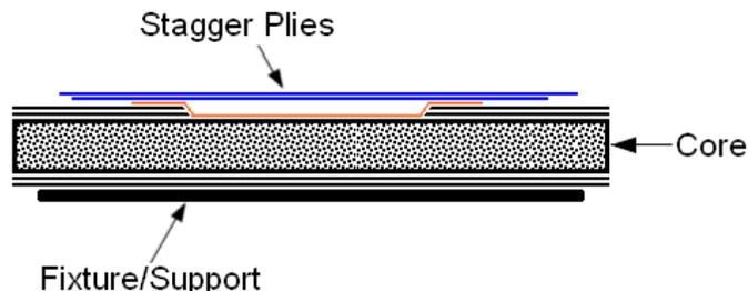
**Figure 51-38 Application of the Epibond adhesive and the Staggered Plies of Plain Weave**
