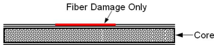
**Figure 51-28 Cross Section of Damaged Area**
