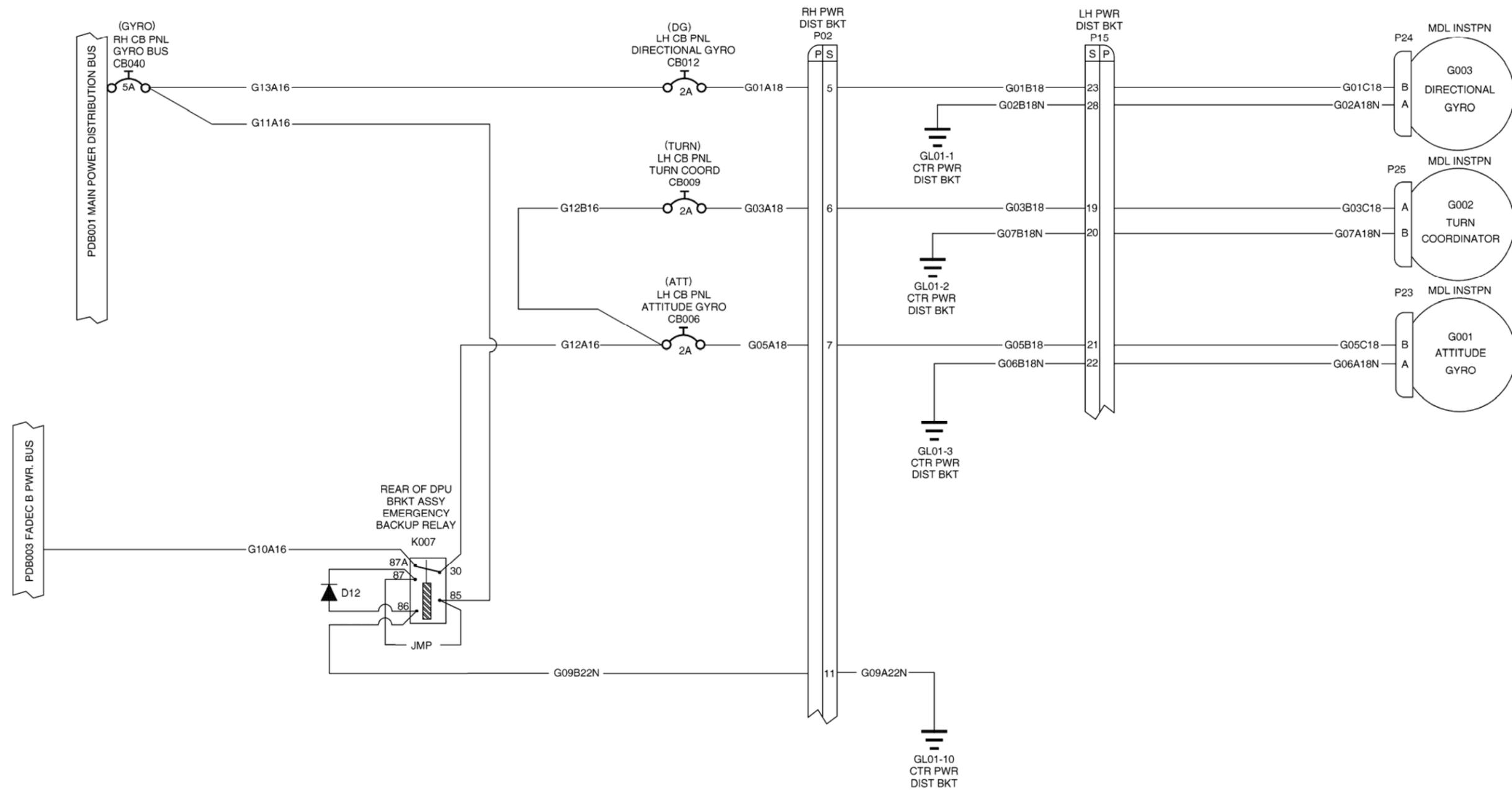
Figure 91-19 Electric Gyro Instrument System
