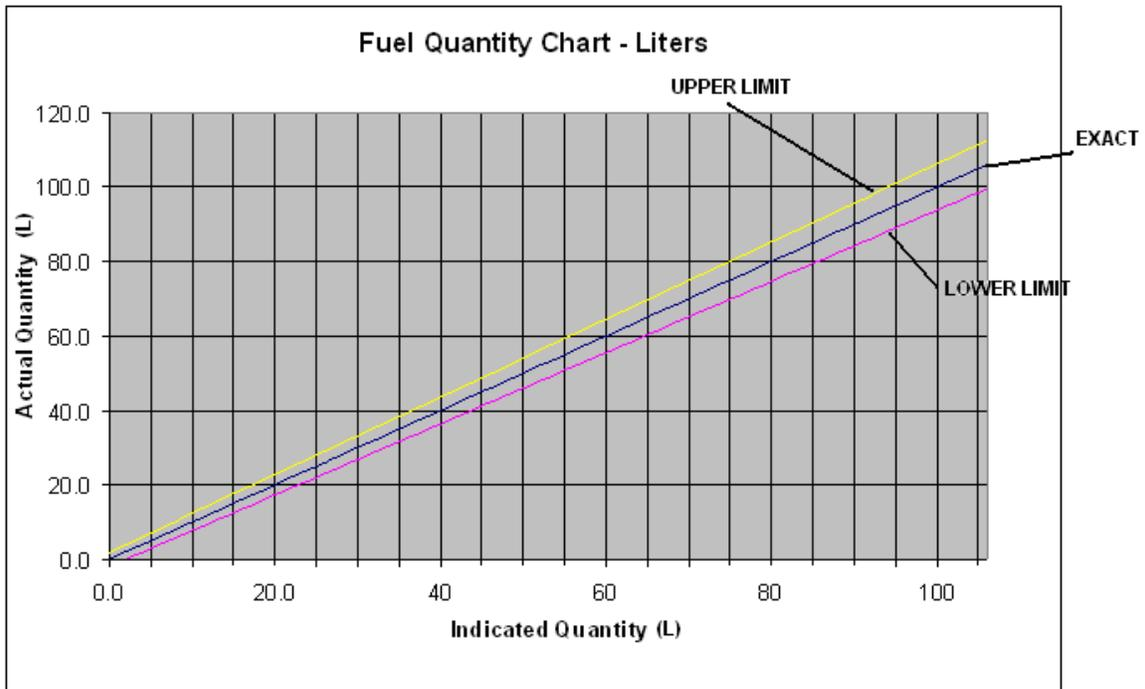
**Figure 28-30 Fuel Quantity Tolerance Chart – Liters**
