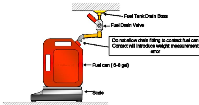
Figure 28-27 Fuel Drain Equipment Set Up
