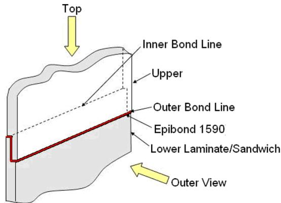
Figure 51-41 Representation of the Laminate/ Sandwich adhesive joint
