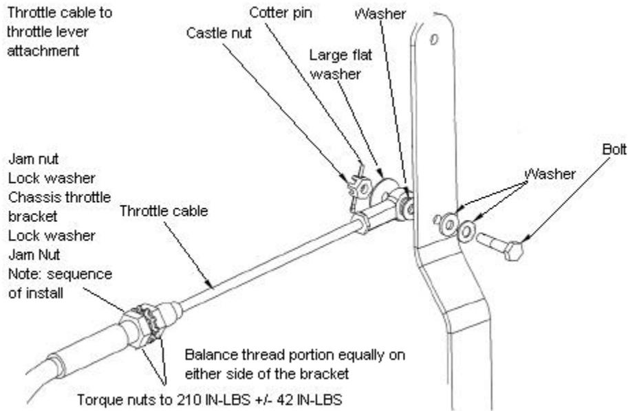
**Figure 76-3 Throttle Cable and Lever Attachment**
