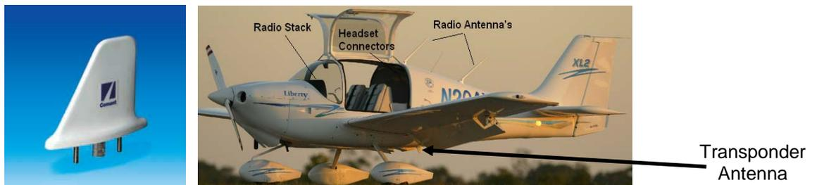
Figure 34-52 Transponder Antenna Placement.
