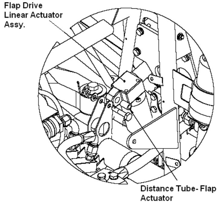
**Figure 27-65 Flap Drive Linear Actuator Assembly**
