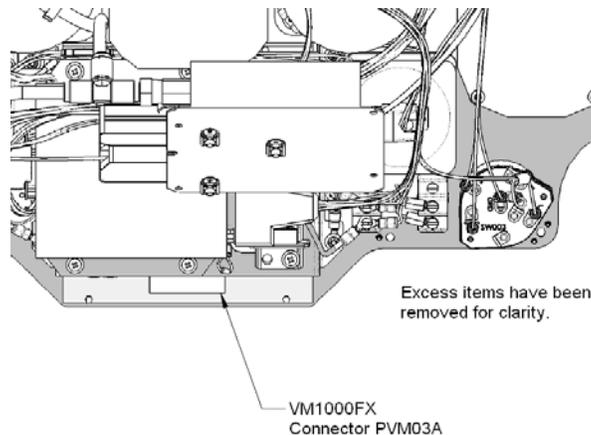
**Figure 31-5 Location of the Connector on the VM1000FX**
