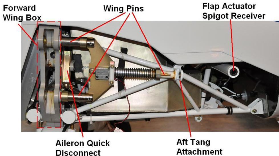
Figure 57-13 Fuselage Inspection Points
