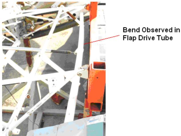
**Figure 27-78 Bent Flap Drive Tube**
