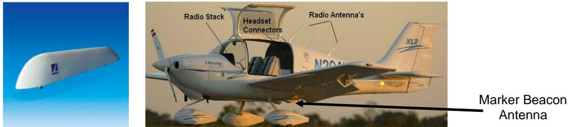
**Figure 34-45 Marker Beacon Antenna Installation**
