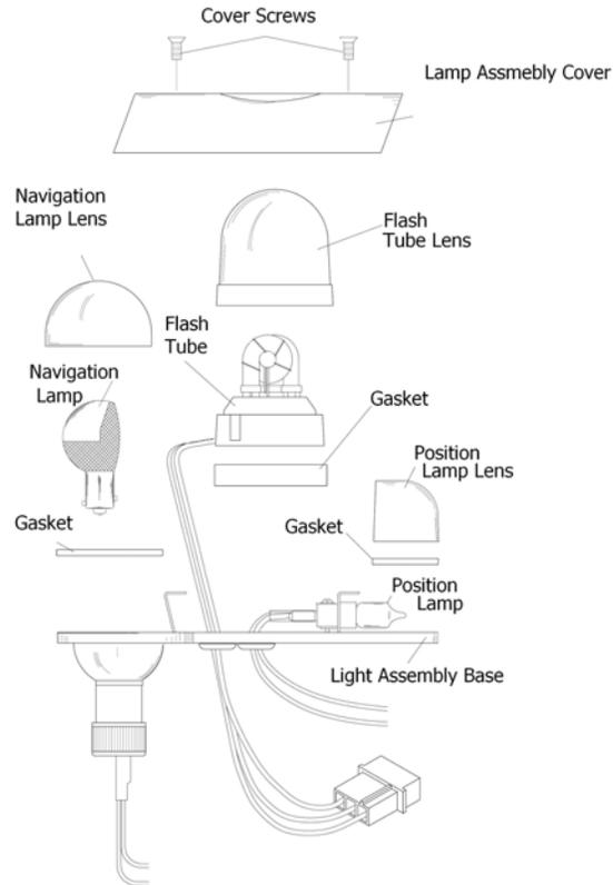
**Figure 33-9 Anti-collision light installation**
