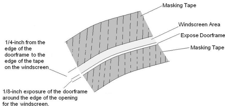
**Figure 56-16 Diagram Showing the Area to Mask-off Before Applying the Pro-Seal Sealant**
