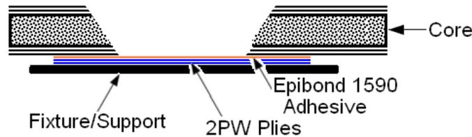
**Figure 51-14 Application of the Epibond Adhesive and the Staggered Plies of Plain Weave with a Backing Support**
