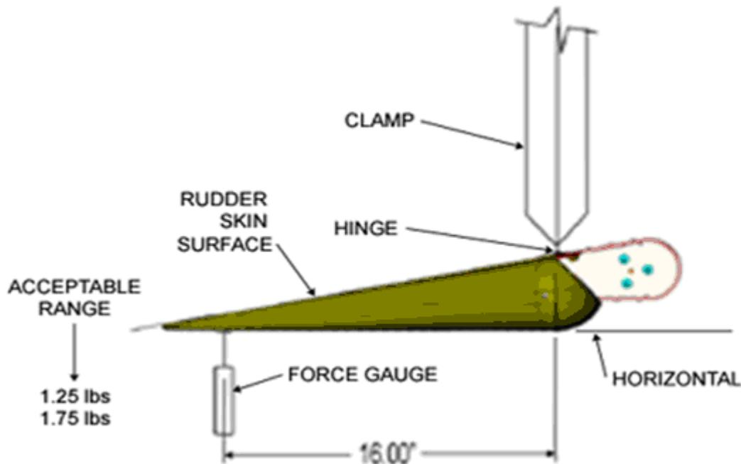
**Figure 51-57 Location of Load Cell on Rudder**
