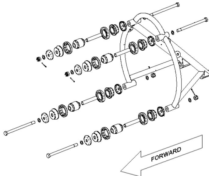
Figure 71-24 Exploded View of Engine Mount Installation
