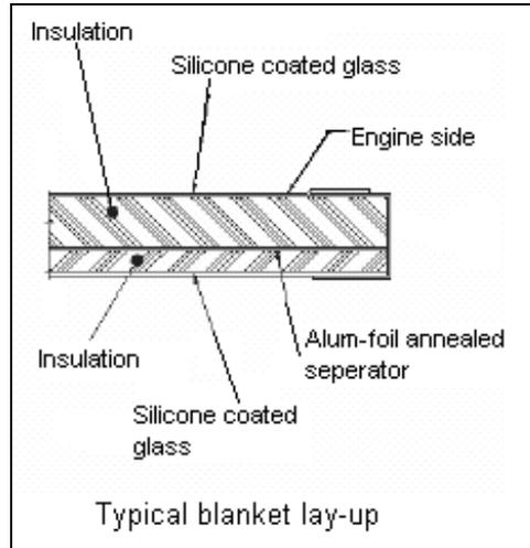
Figure 71-27 Firewall Cutaway
