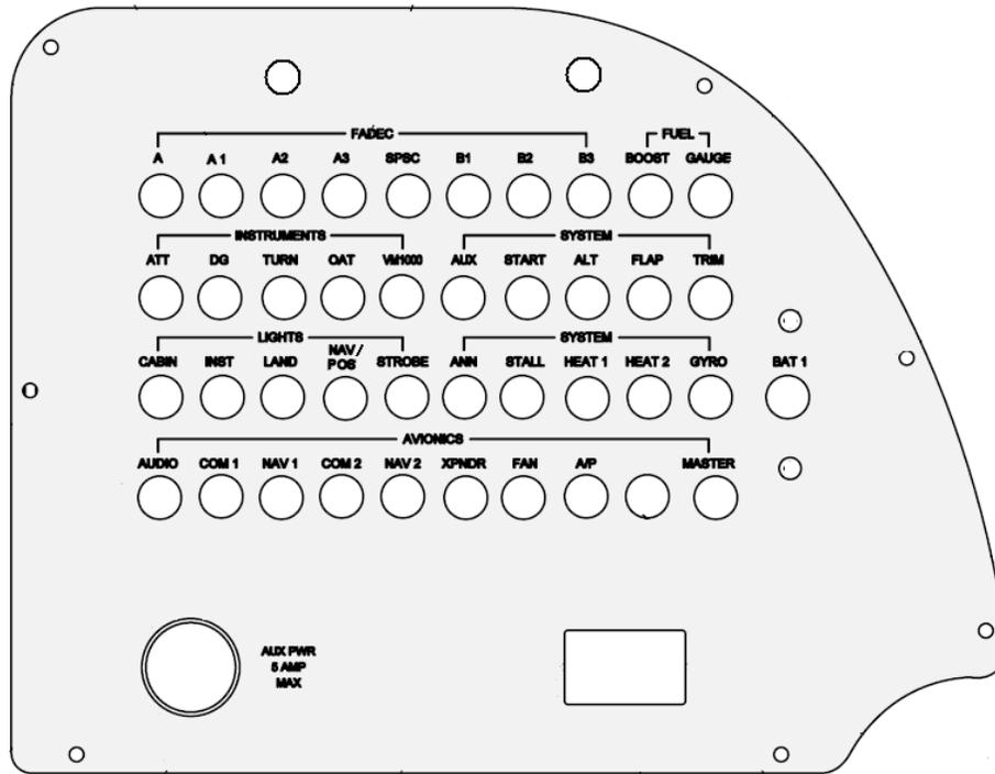
**Figure 11-26 Placard for the CB (Circuit Breaker) Panel P/N 135A-80-303**
