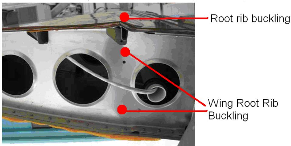
**Figure 57-15 Buckling on Root Rib Aft of Main Spar and Wing Skin**
