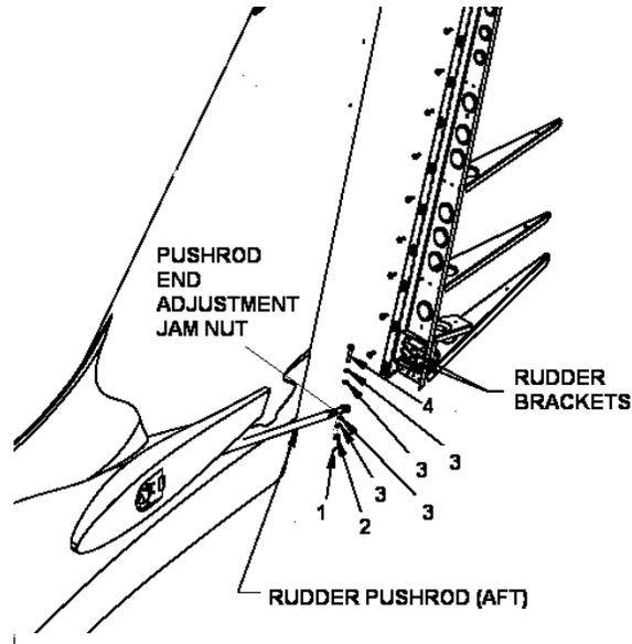
**Figure 27-26 Rudder Pushrod Aft Connection**
