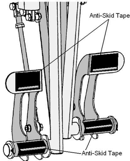
**Figure 11-33 Location of the anti-skid strip tape on the rudder pedals and the toe brake pedals**
