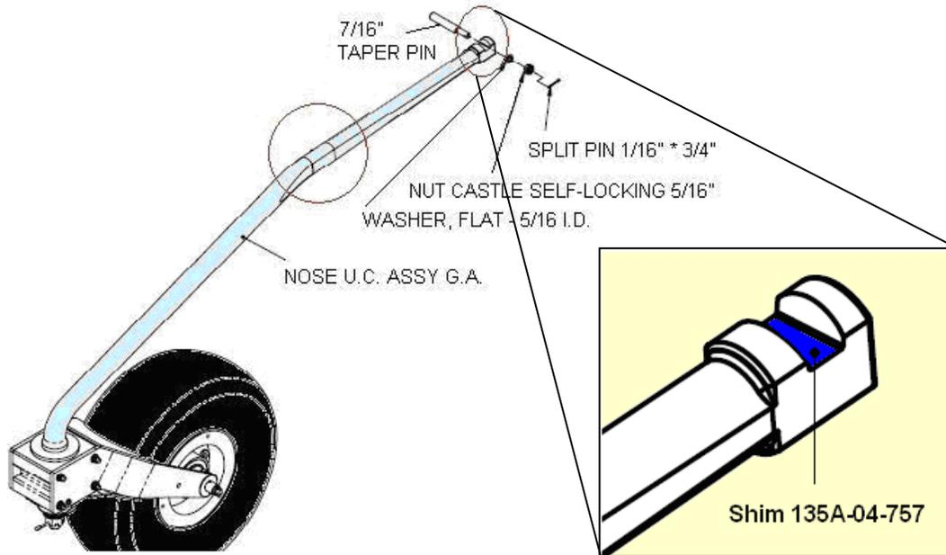
**Figure 32-3 Nose Gear Installation**
