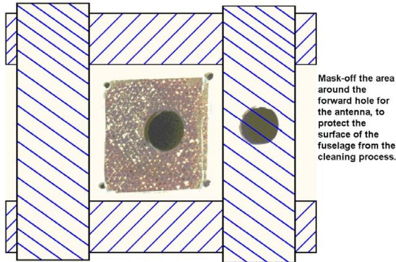
**Figure 23-12 Area of the Fuselage to Mask-Off to Protect the Fuselage**
