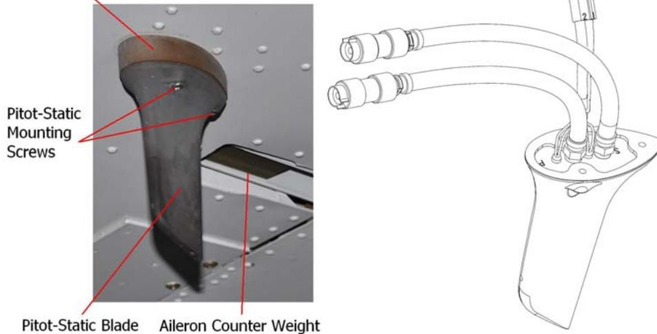
**Figure 30-1 Pitot-Static Blade**
