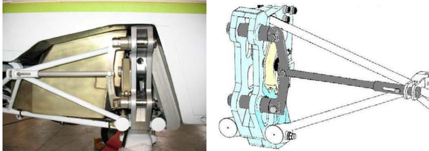
**Figure 57-6 Mechanical Wing Lock Mechanism**
