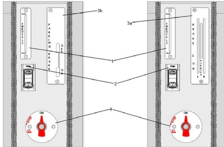
**Figure 11-29 Placards on the Lower Center Console**
