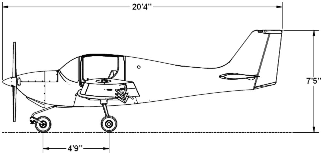
**Figure 06-2 (Reference Only) Side View of Airplane Dimensions \***
