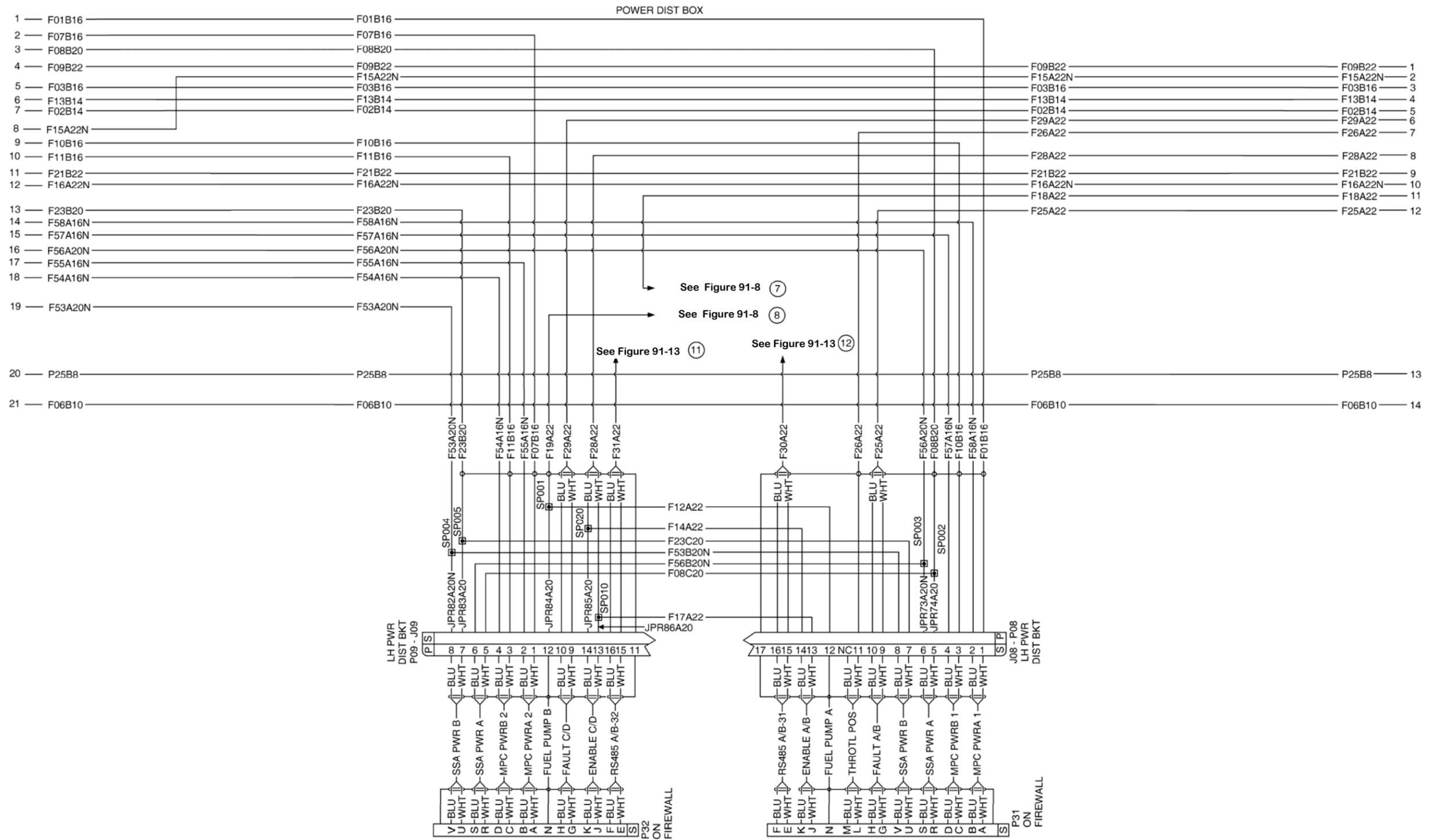
Figure 91-10 FADEC System Cabin Harness (2 OF 3)
