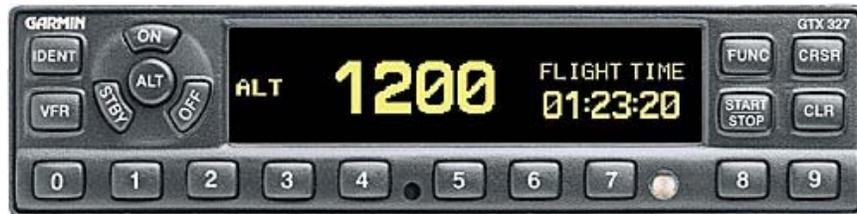
Figure 34-51 GTX 327 Transponder
