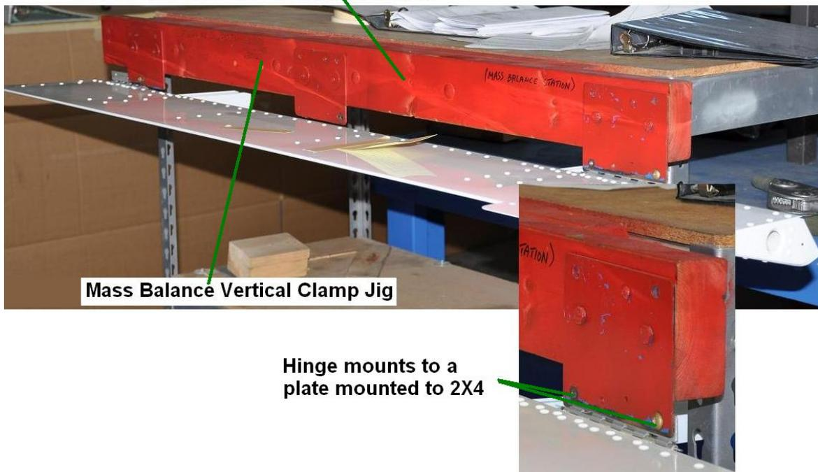
**Figure 51-55 Mass Balance Vertical Clamp Jig**
