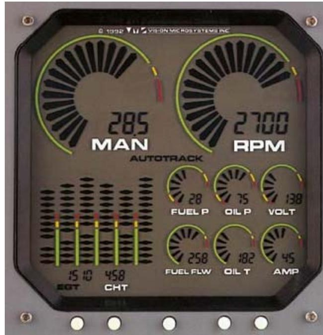
**Figure 31-20 VM-1000FX Engine Instrument Display**
