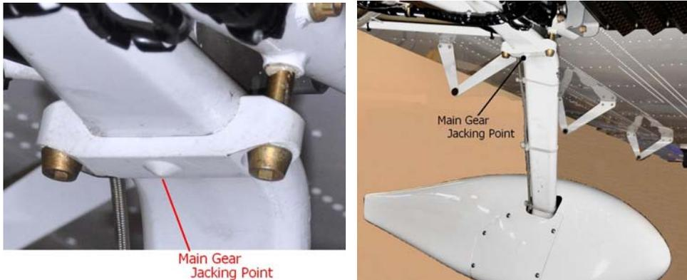
**Figure 07-6 Main Gear Jacking Points**
