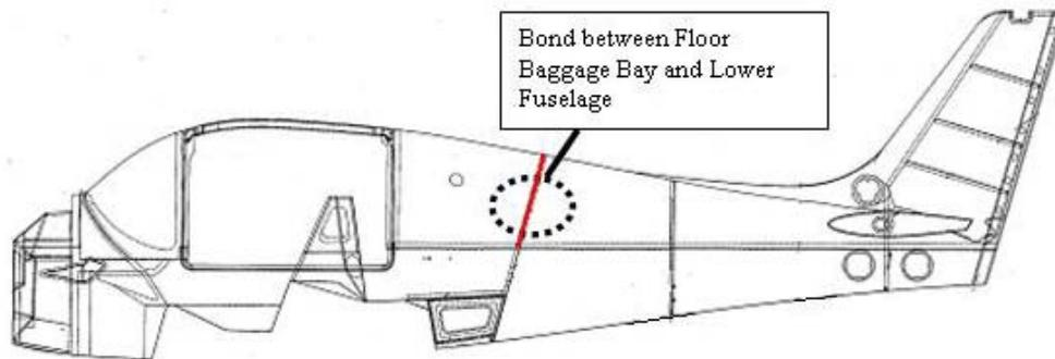
**Figure 53-4 Inspection Location Between The Bonded Section Of The Baggage Bay Closeout**
