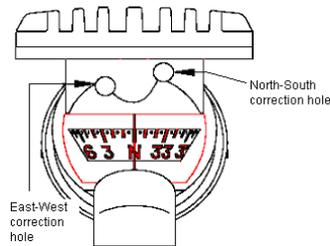
**Figure 34-32 View of Compass Showing Correction Holes**
