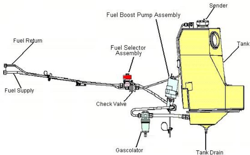
**Figure 28-1 Fuel System Components**
