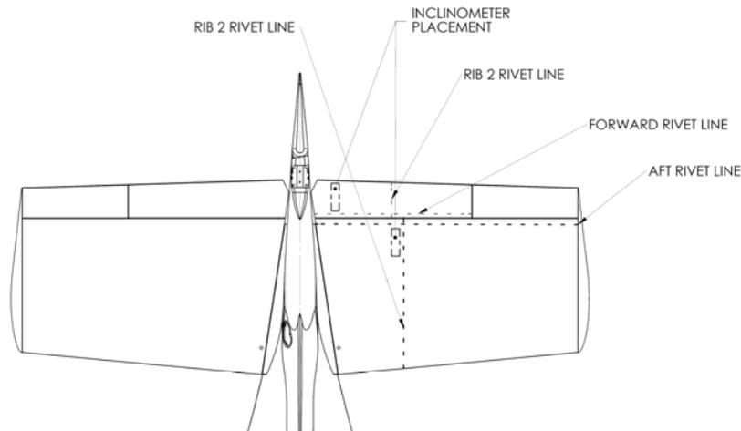
**Figure 27-89 Location Inclinator for horizontal stabilizer**
