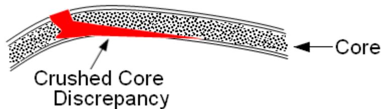
**Figure 51-24 Same Area Indicating the Damaged Area**
