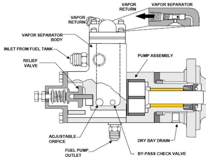
Figure 73-2 Engine Drive Fuel Pump
