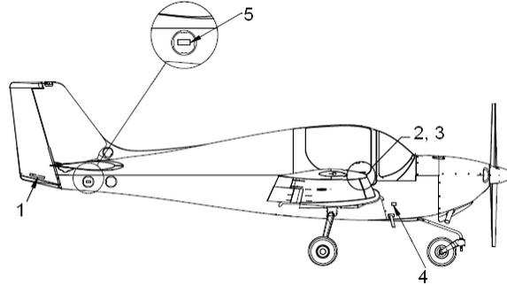
Figure 11-9 Exterior Placards – Starboard Side of Airplane
